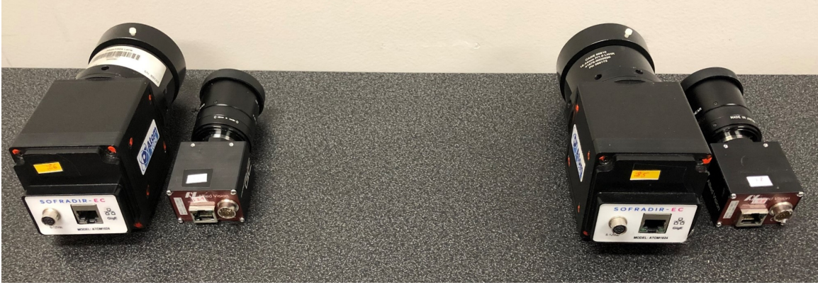
Figure 6. From the Left to the Right: Left IR Camera, Left EO Camera, Right IR Camera, Right EO Camera
