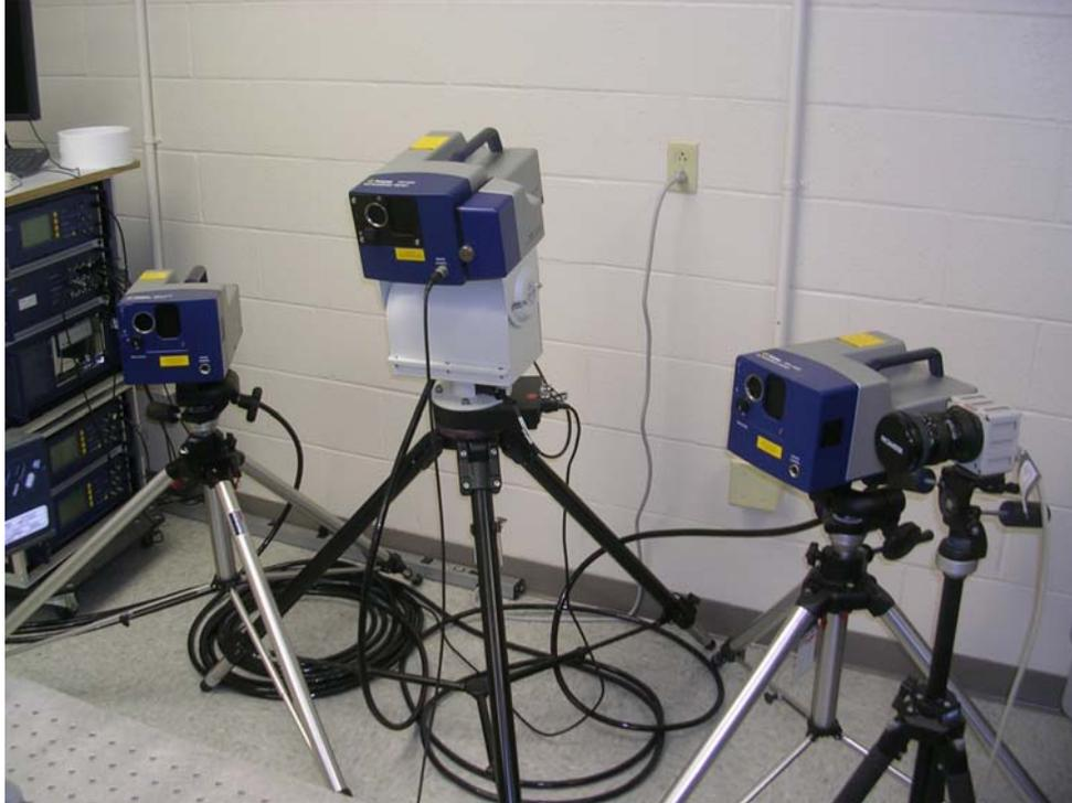
Figure 12: 3-D Laser Vibrometer Setup
