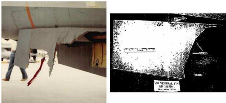
Figure 5.8: Typical Ventral Fin Failure Geometry
