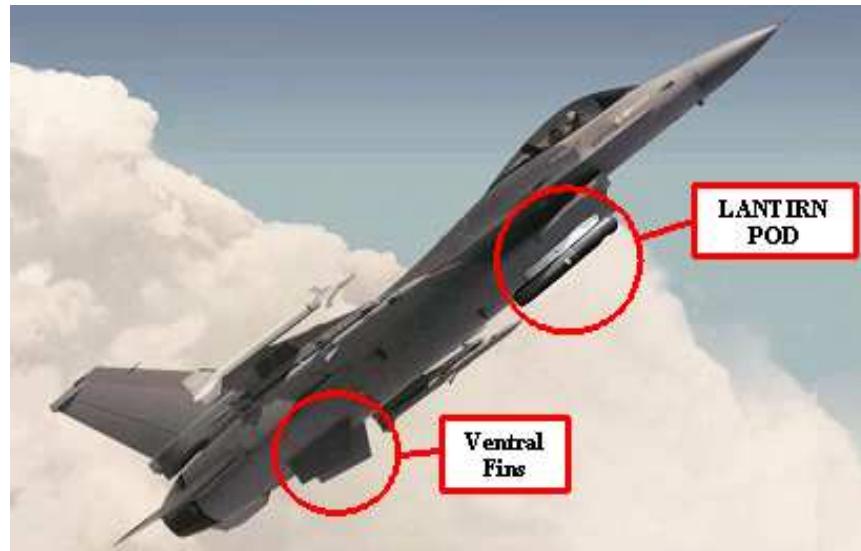
Figure 1.1: Location of Ventral Fins and LANTIRN Pods
