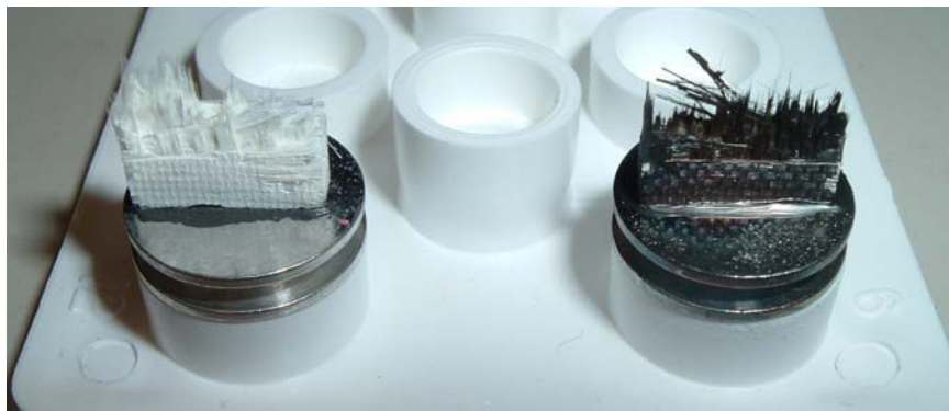
Figure 17. Specimens prepared for SEM. Uncoated specimen on left, carbon coated specimen on right.
