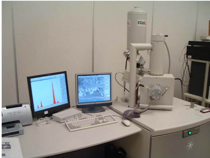
Figure 13. FEI Scanning Electron Microscope (SEM) and EDAX Energy Dispersive X-ray Analysis Systems (EDS).
