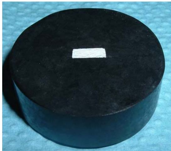
Figure 18. Mounted and polished N720/A specimen.
