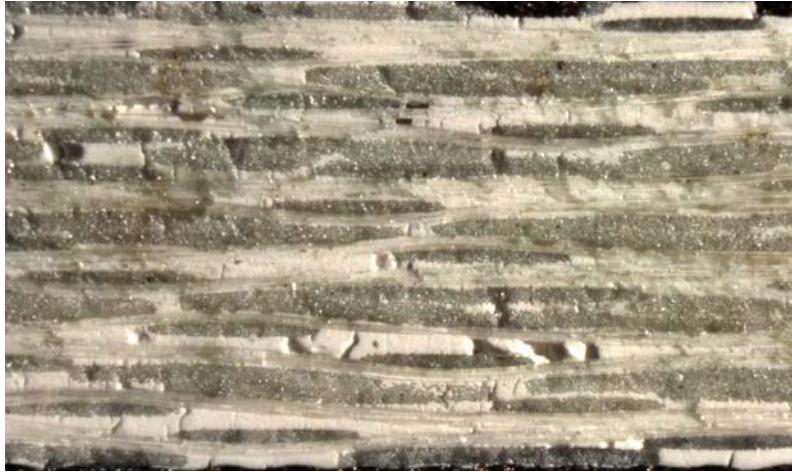
Figure 7. Optical micrograph of polished as-received N720/A material.
