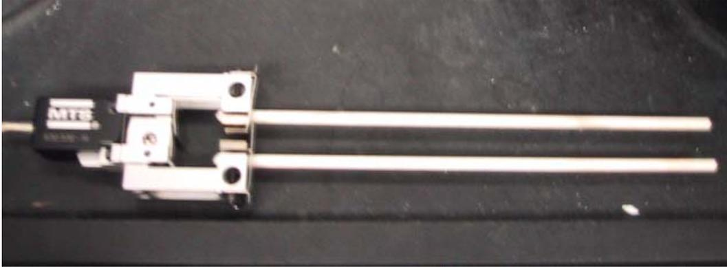
Figure 18. Extensometer Equipped with Alumina Rods
