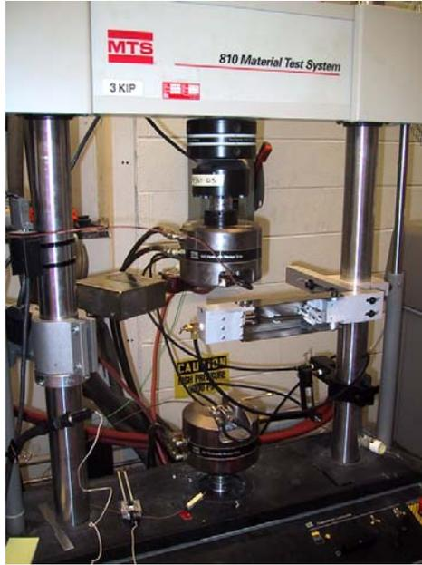
Figure 12. 25kN Servo Hydraulic Machine
