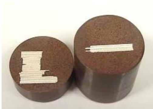
Figure 23. Pieces of Specimen Mounted in Conductive Resin
