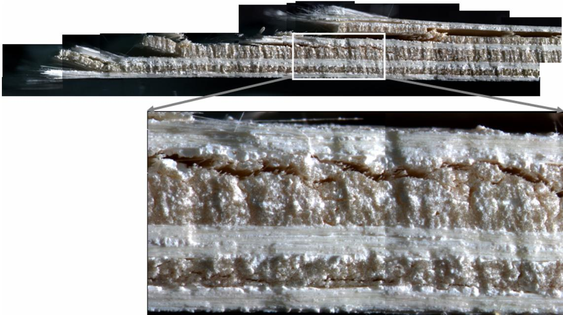
Figure 61. Magnified View of a Fracture Surface from Panel M1 Showing Cracks Initiating and Self-arresting in 90° fiber layers
