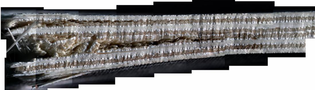
Figure 62. Crack Propagation through Fibrous 90° Layers of a Specimen from Panel M2.
