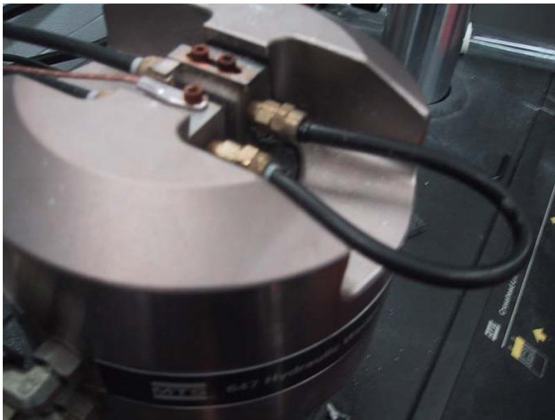
Figure 14. Tubes for Cooling Water Connected to Hydraulic Wedge Grips
