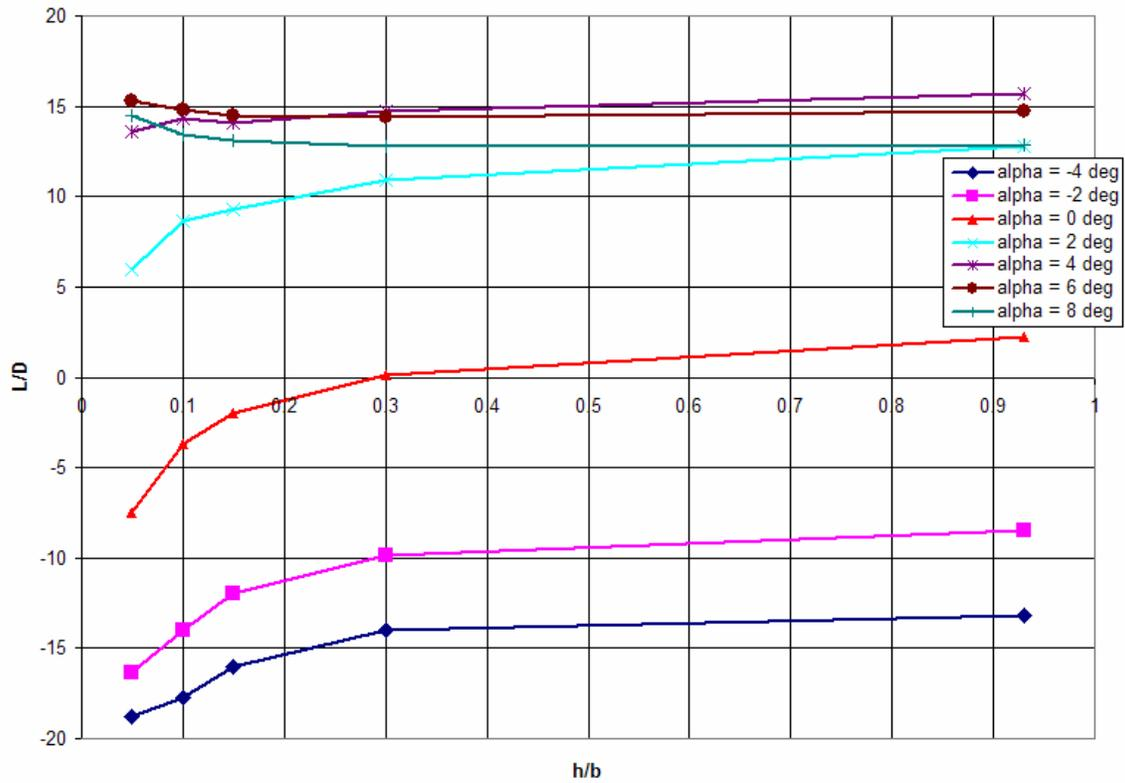
Figure 60: Chevon UCAV  $L/D$  vs.  $(h/b)$  80 mph
