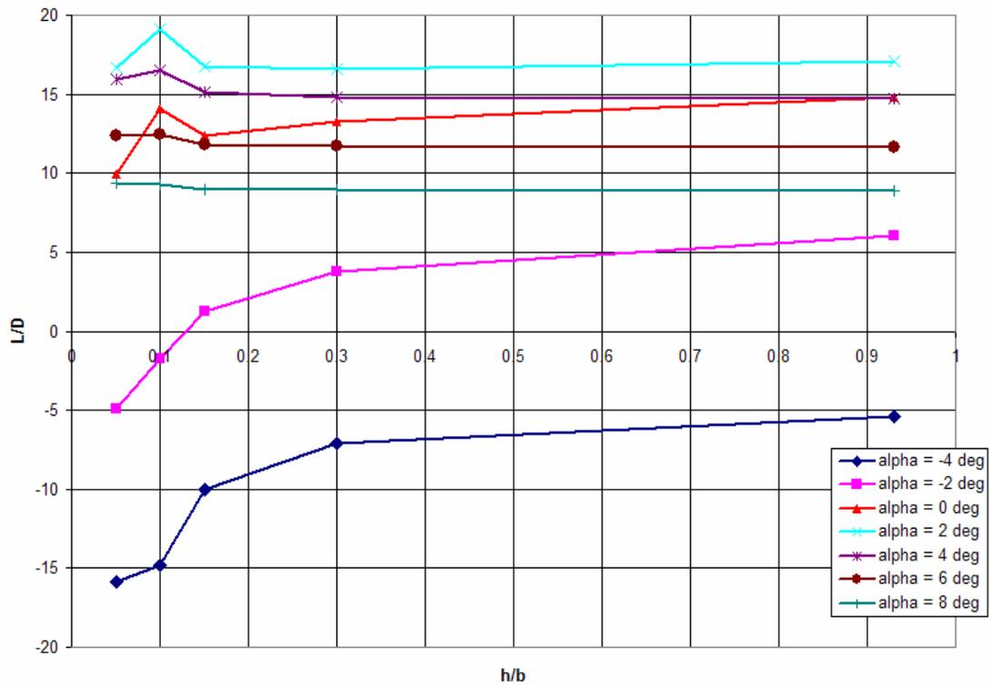
Figure 72: Lambda UCAV  $L/D$  vs. ( $h/b$ ) 80 mph
