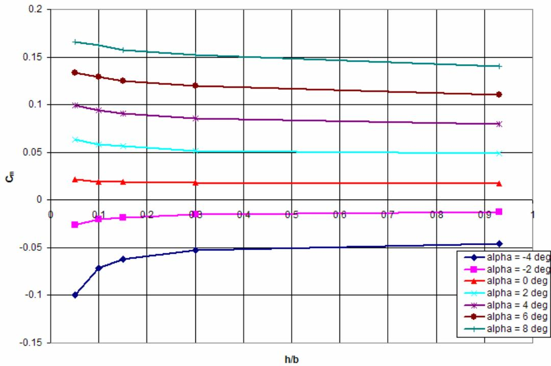
Figure 75: Lambda UCAV  $C_m$  vs.  $(h/b)$  100 mph
