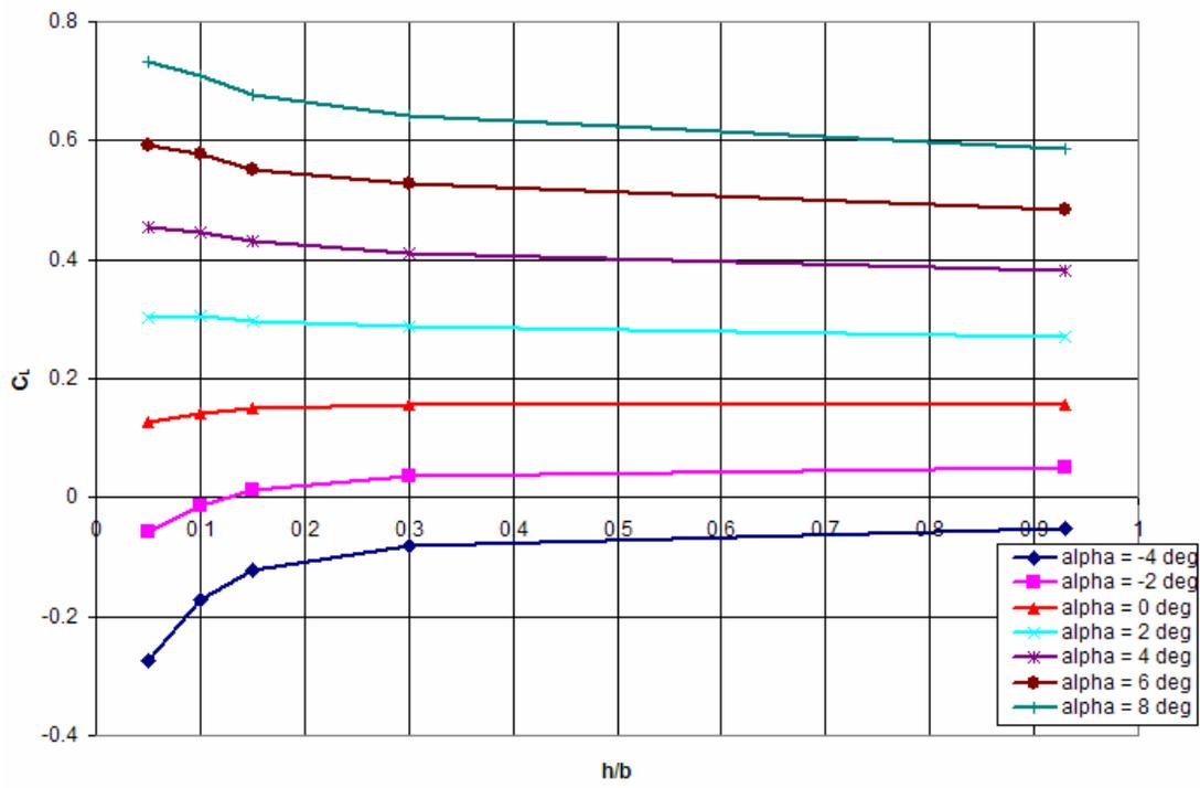
Figure 69: Lambda UCAV  $C_L$  vs. ( $h/b$ ) 80 mph
