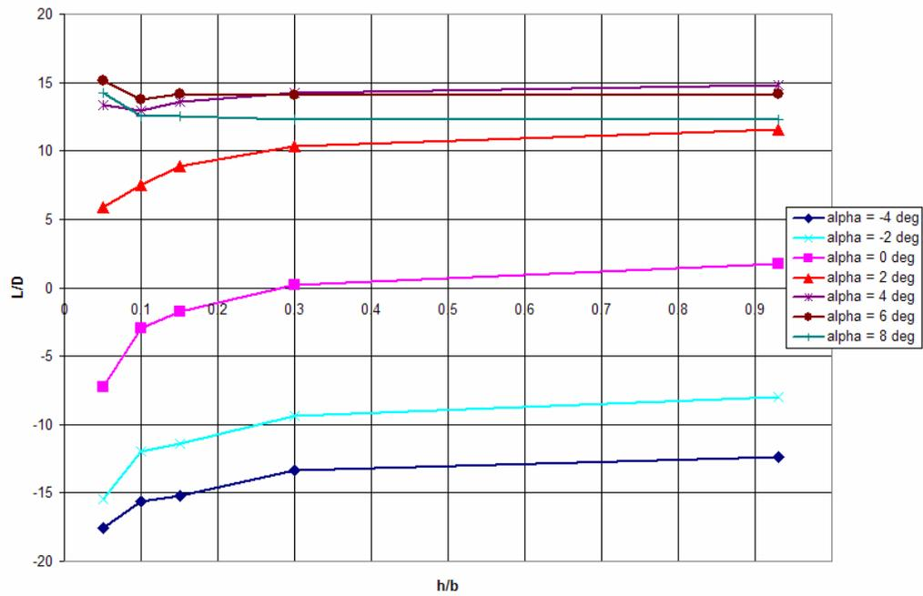
Figure 48: Chevron UCAV L/D vs. (h/b) 60 mph
