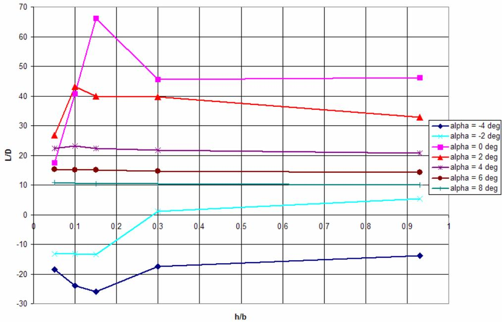
Figure 49: Lambda UCAV L/D vs. (h/b) 40 mph
