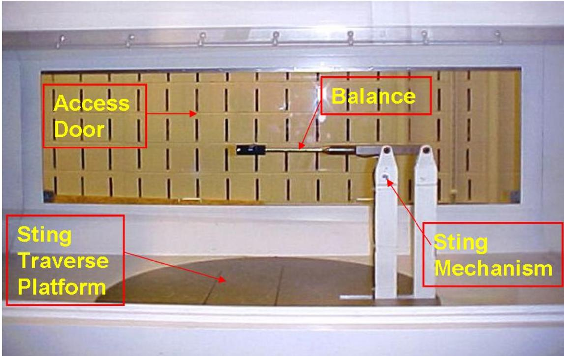
**Figure 8: Wind Tunnel Test Section and Components (22)**
