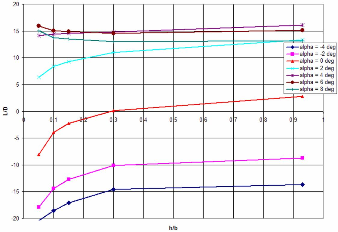
Figure 64: Chevon UCAV  $L/D$  vs.  $(h/b)$  100 mph
