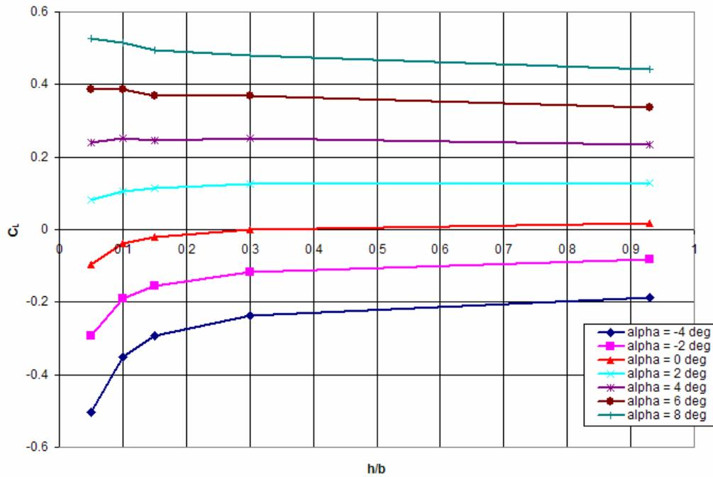
Figure 57: Chevron UCAV  $C_L$  vs.  $(h/b)$  80 mph
