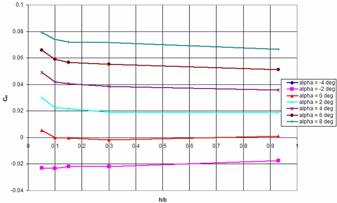
Figure 55: Chevon UCAV  $C_m$  vs.  $(h/b)$  60 mph
