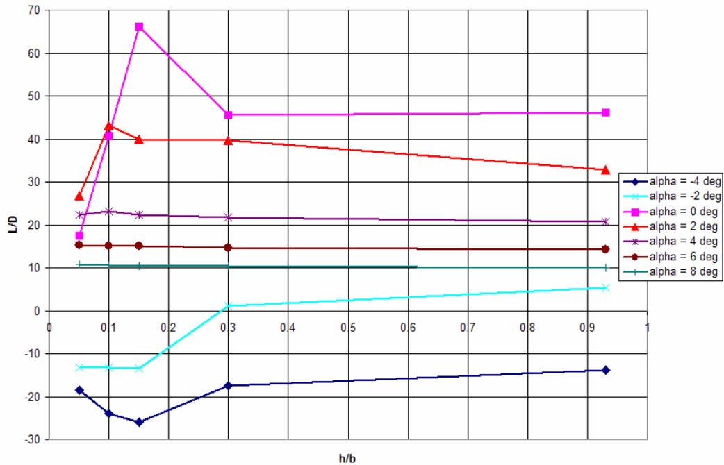
Figure 66: Lambda UCAV  $L/D$  vs.  $(h/b)$  40 mph
