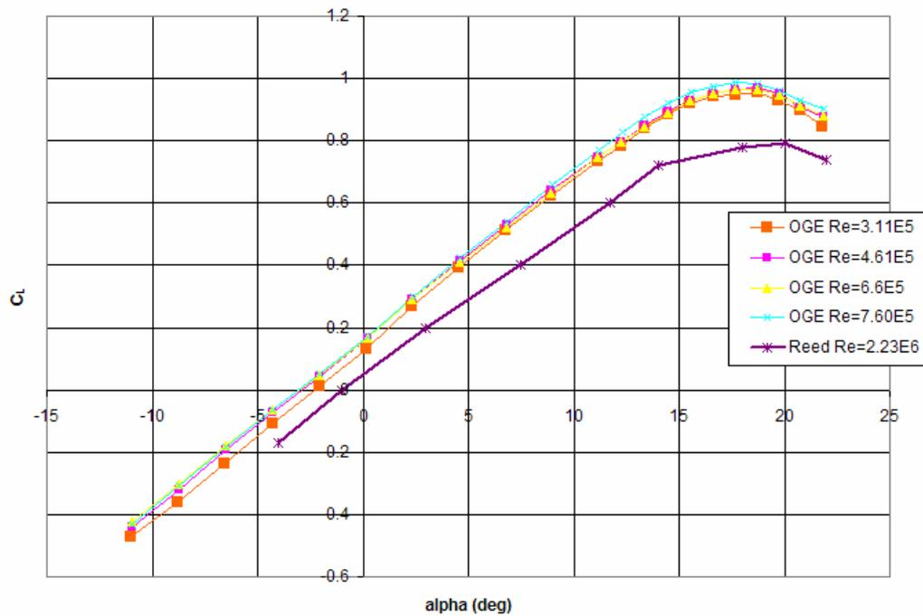
**Figure 29: Lambda UCAV Aerodynamic Comparison -  $C_L$  vs. alpha**
