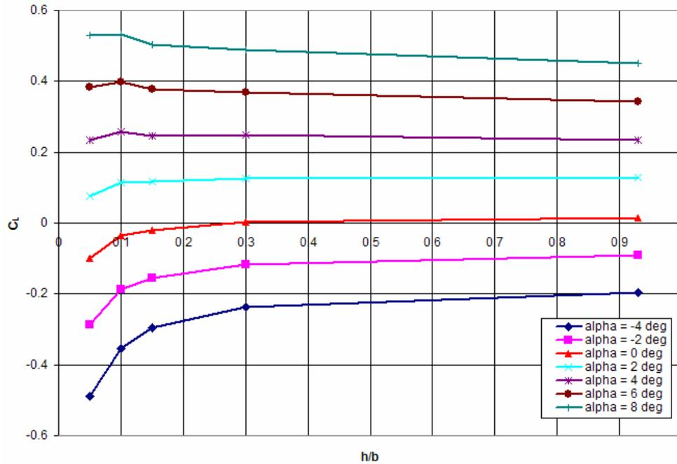
Figure 32: Chevron UCAV Ground Effect -  $C_L$  vs.  $(h/b)$  40 mph
