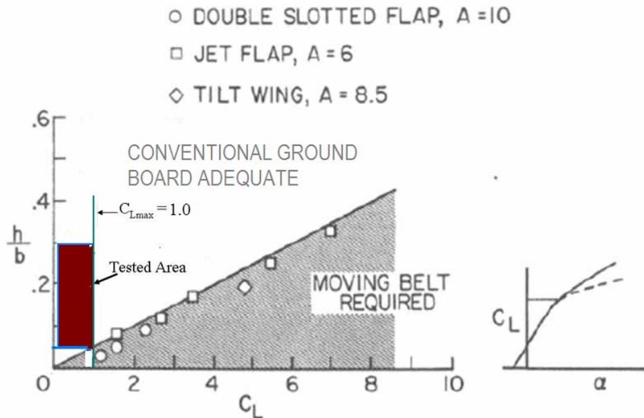
**Figure 5: Conditions Requiring an Endless-belt Ground Plane (20)**
