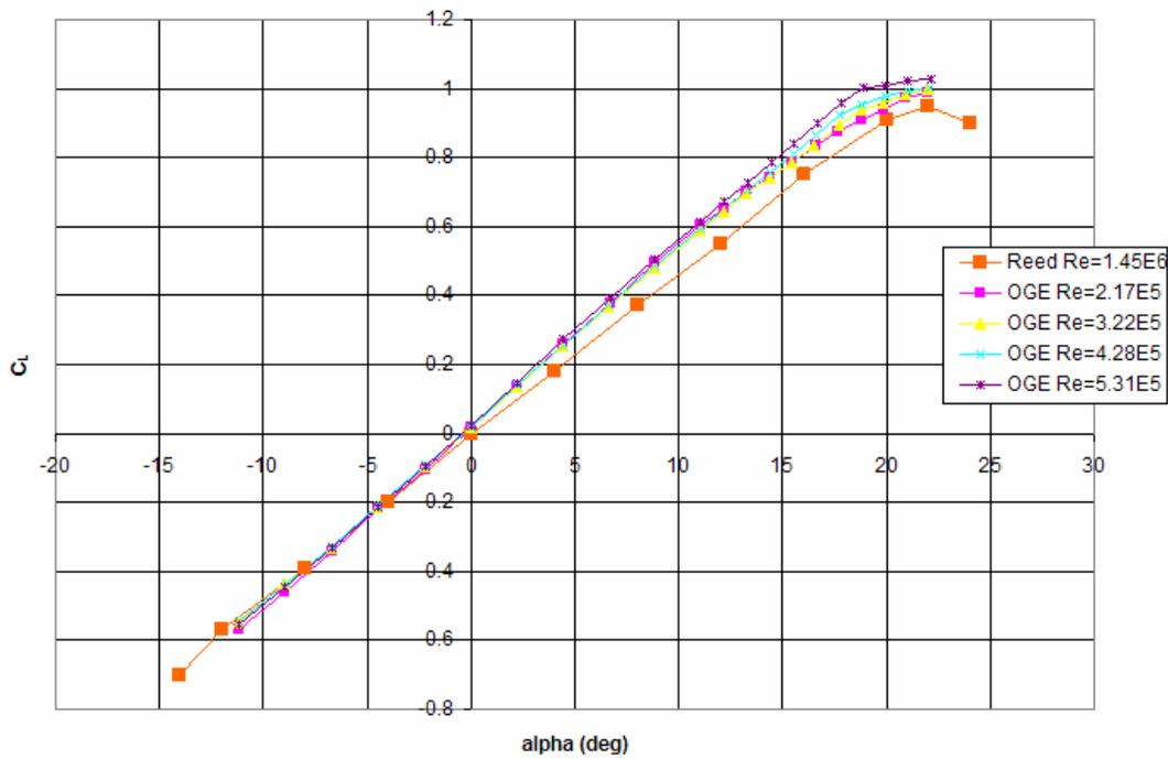
Figure 28: Chevron UCAV Aerodynamic Comparison -  $C_L$  vs.  $\alpha$
