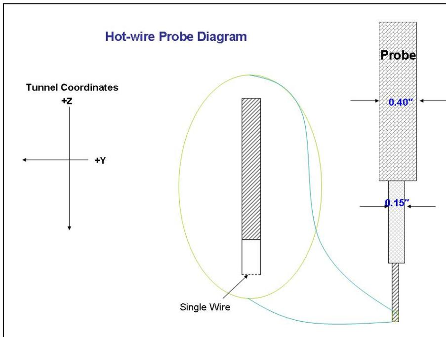
**Figure 21: Schematic of Hot-wire Probe Configuration (1)**
