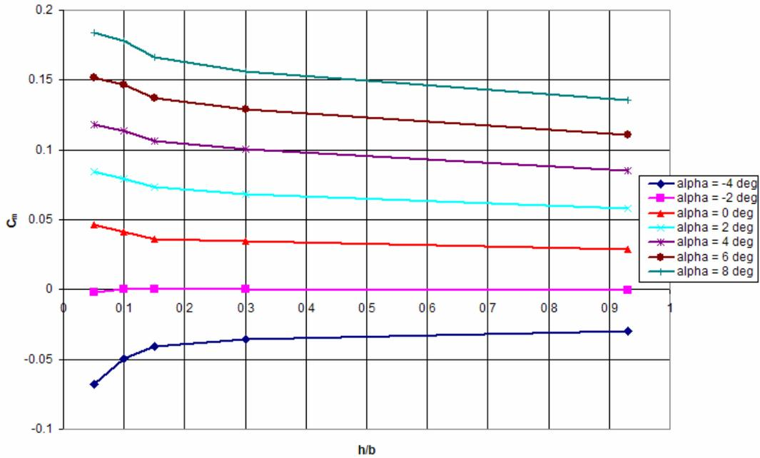
Figure 65: Lambda UCAV  $C_m$  vs.  $(h/b)$  40 mph
