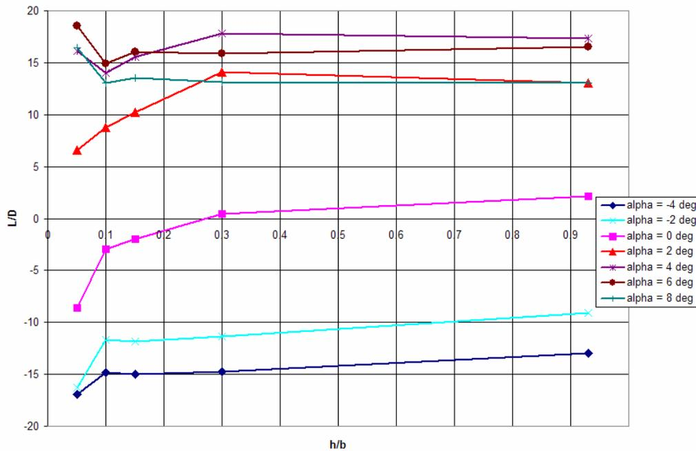
Figure 47: Chevron UCAV L/D vs. (h/b) 40 mph
