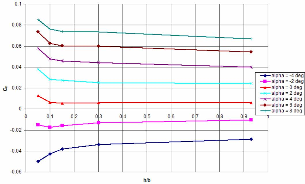
Figure 53: Chevron UCAV  $C_m$  vs.  $(h/b)$  40 mph
