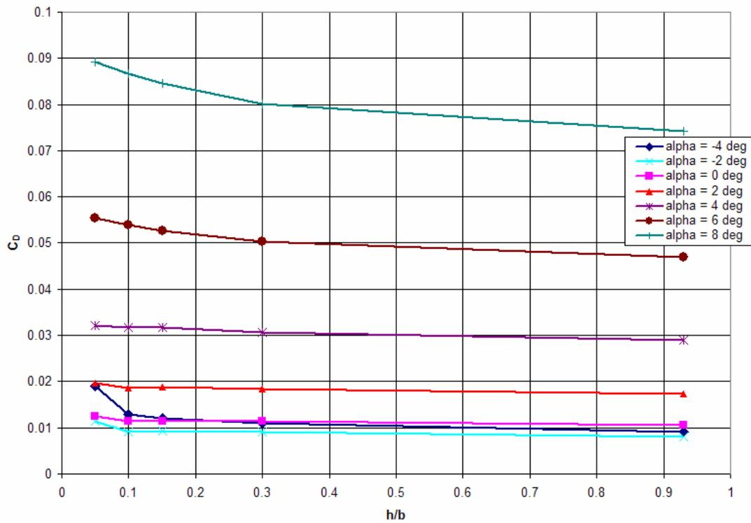
Figure 74: Lambda UCAV  $C_D$  vs. ( $h/b$ ) 100 mph
