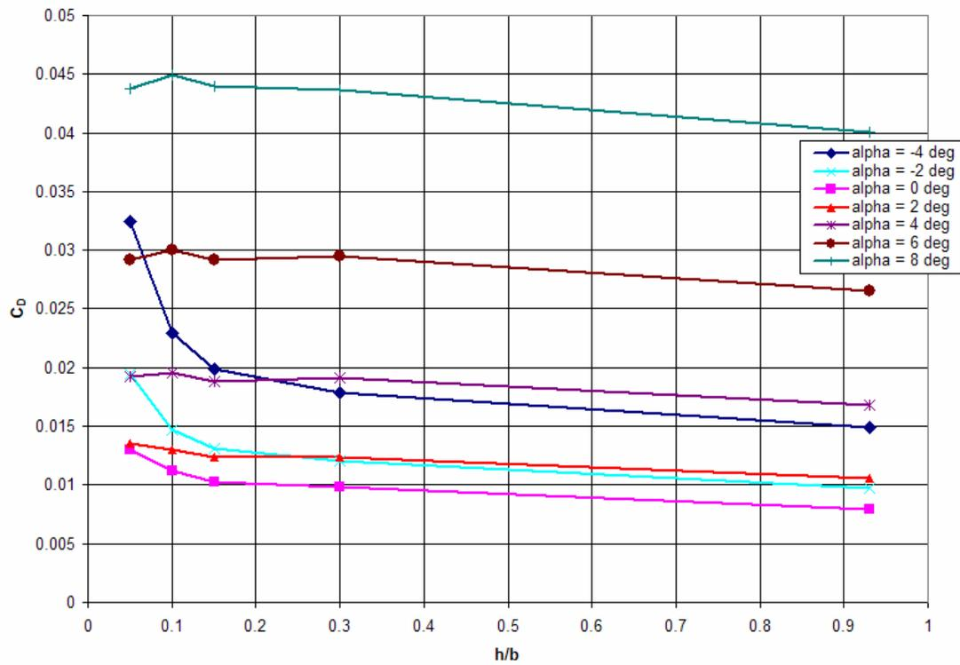
Figure 62: Chevron UCAV  $C_D$  vs. ( $h/b$ ) 100 mph
