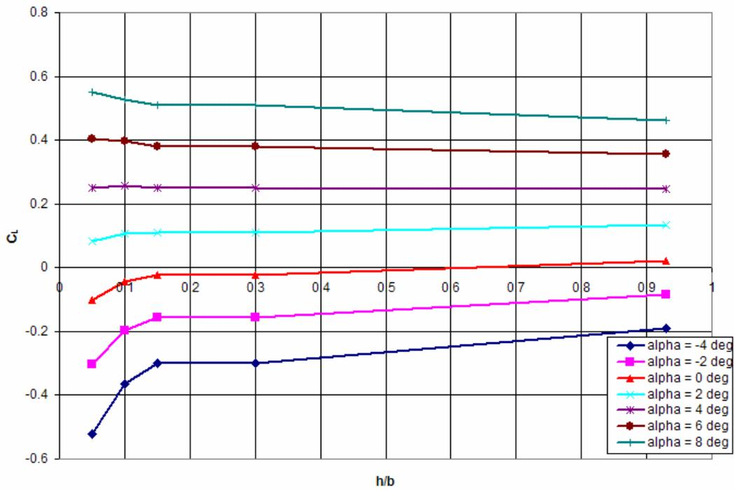
Figure 61: Chevron UCAV  $C_L$  vs. ( $h/b$ ) 100 mph
