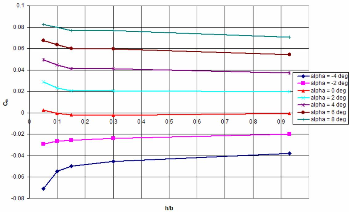
Figure 63: Chevon UCAV  $C_m$  vs.  $(h/b)$  100 mph
