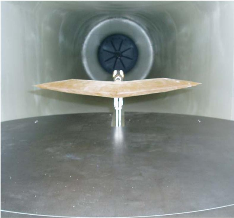
Figure 16:  $\frac{1}{2}$ -Scaled Chevron UCAV in Test Section (1)
