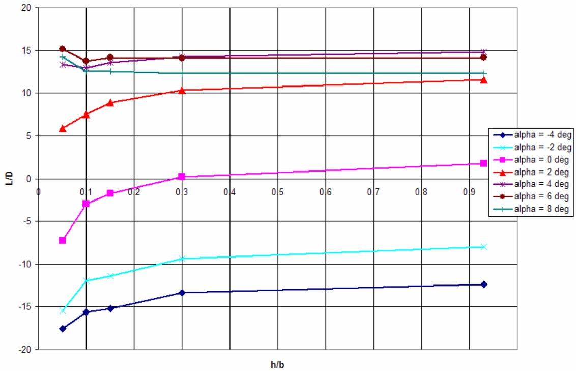
Figure 56: Chevon UCAV  $L/D$  vs.  $(h/b)$  60 mph
