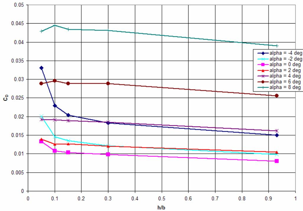
Figure 58: Chevron UCAV  $C_D$  vs.  $(h/b)$  80 mph
