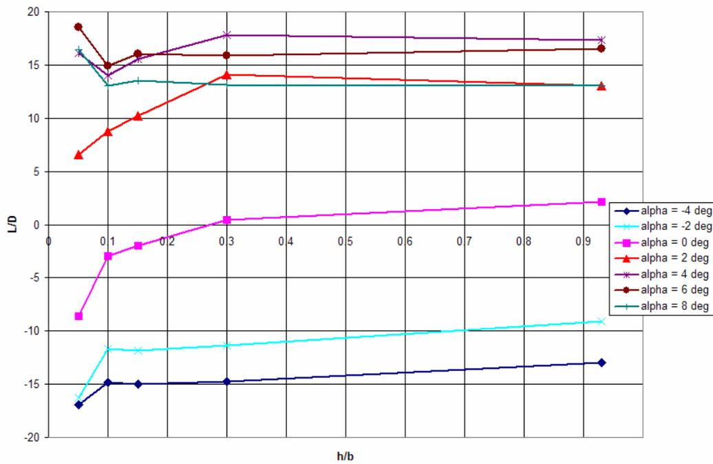
Figure 54: Chevron UCAV  $L/D$  vs.  $(h/b)$  40 mph
