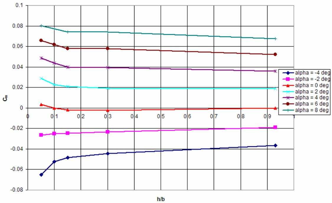
Figure 59: Chevon UCAV  $C_m$  vs.  $(h/b)$  80 mph
