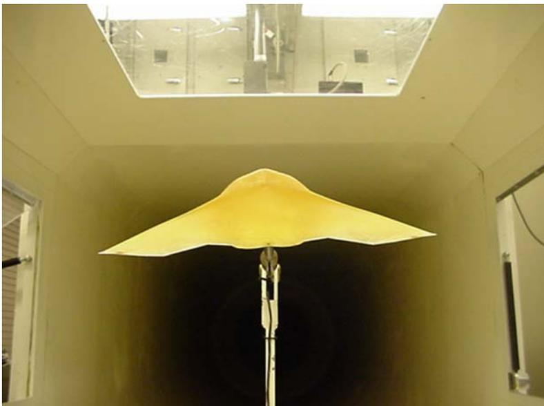
**Figure 18: 0.457-Scaled Lamda UCAV in Test Section**
