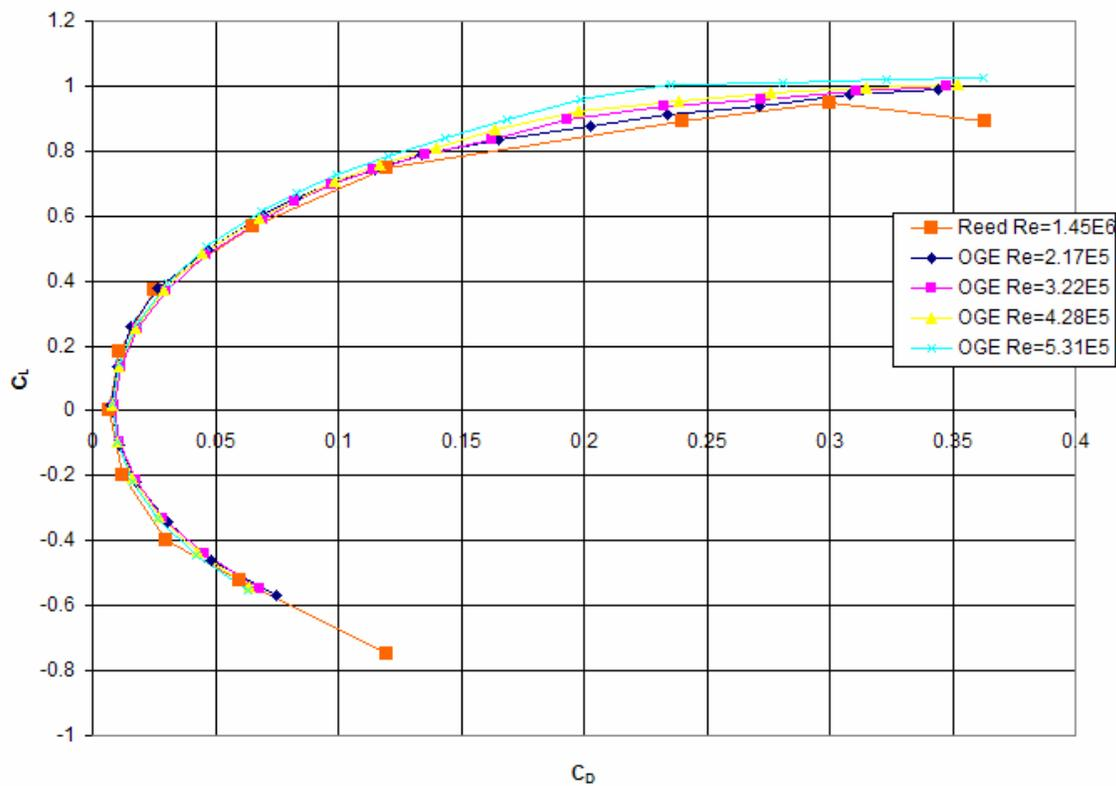
Figure 30: Chevron UCAV Aerodynamic Comparison -  $C_L$  vs.  $C_D$
