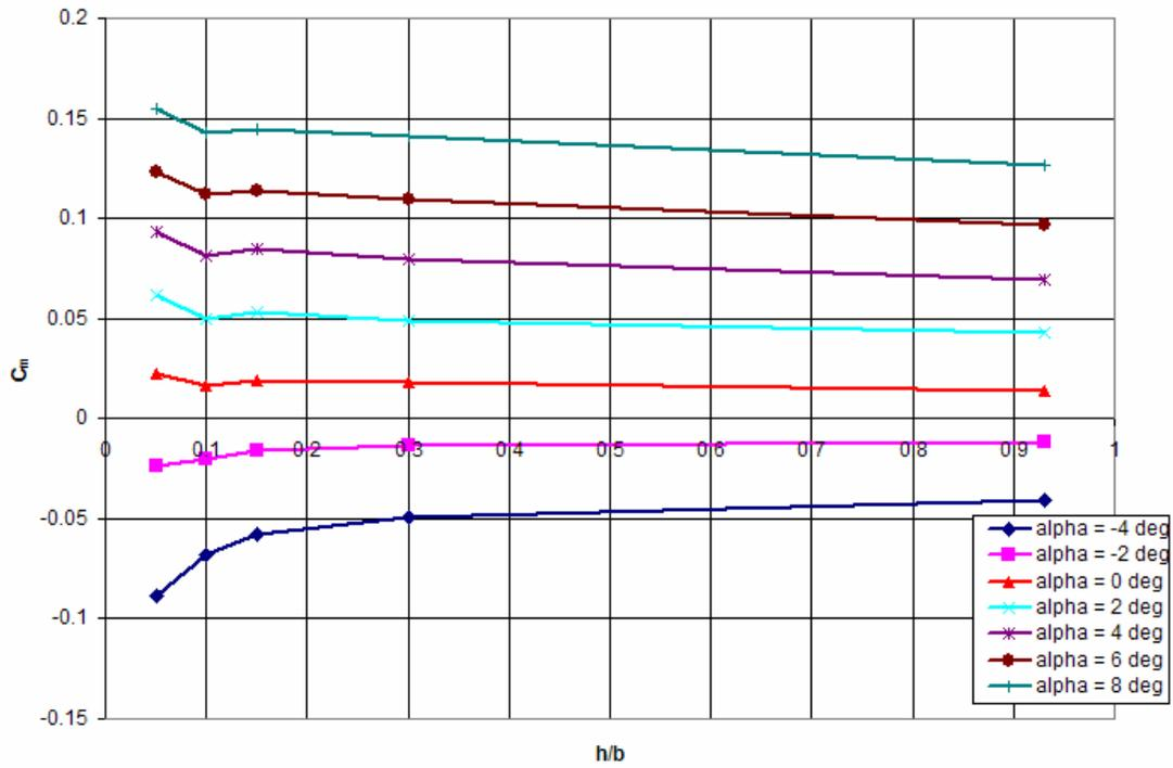
Figure 67: Lambda UCAV  $C_m$  vs. ( $h/b$ ) 60 mph
