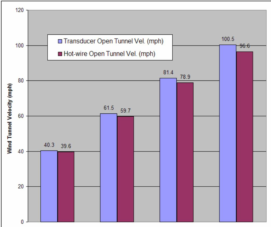
**Figure 24: Open Tunnel Hot-wire and Transducer Velocity Comparison**
