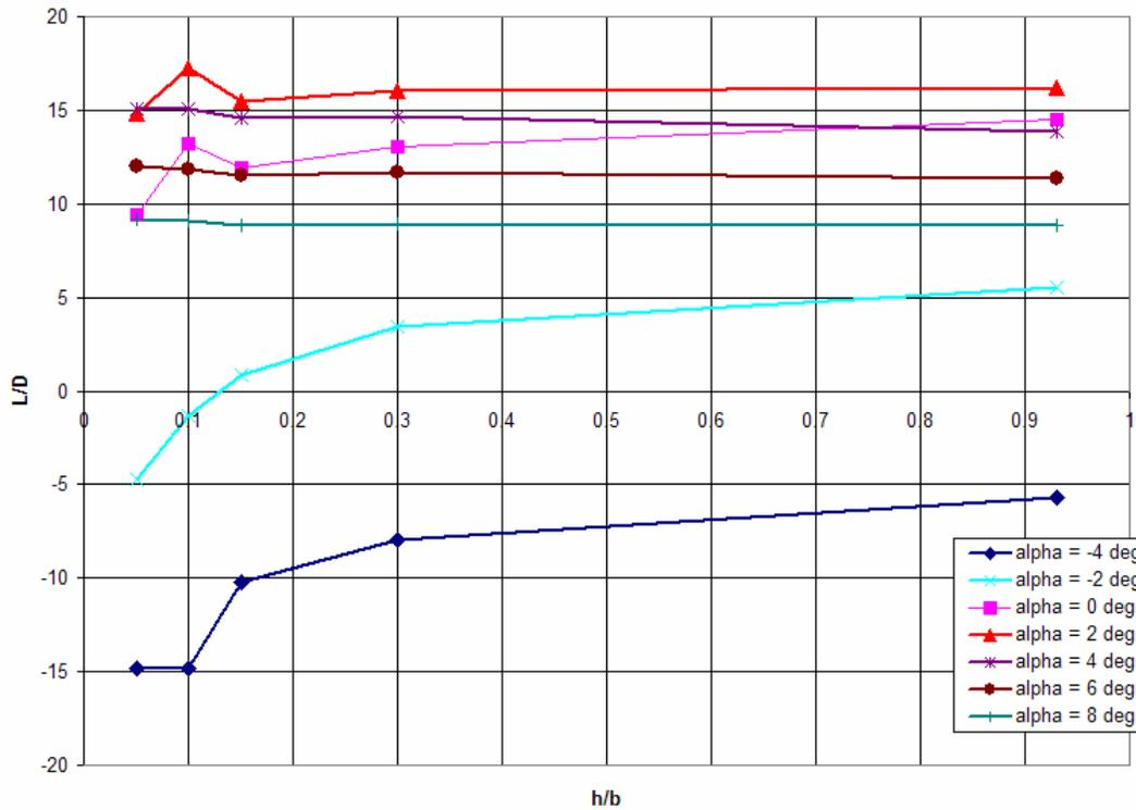
Figure 68: Lambda UCAV  $L/D$  vs. ( $h/b$ ) 60 mph
