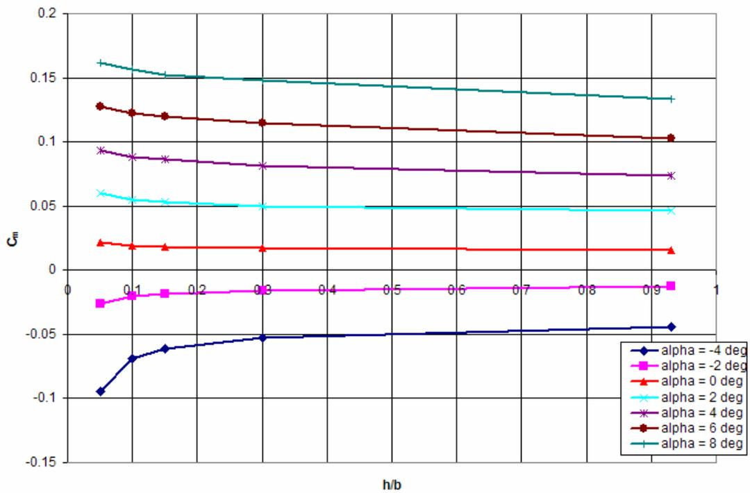
Figure71: Lambda UCAV  $C_m$  vs. ( $h/b$ ) 80 mph
