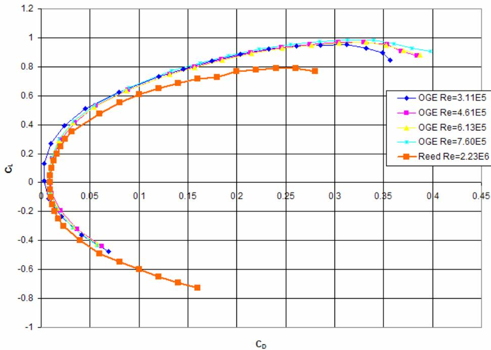
**Figure 31: Lambda UCAV Aerodynamic Comparison -  $C_L$  vs.  $C_D$**
