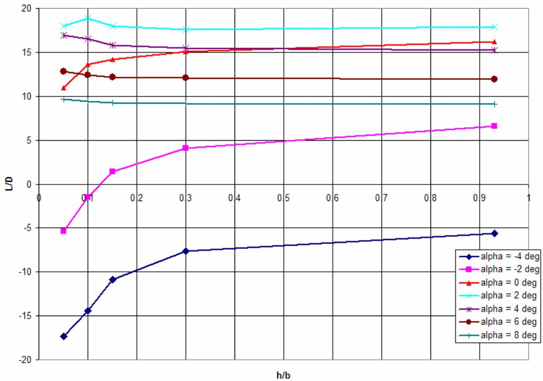
Figure 76: Lambda UCAV  $L/D$  vs.  $(h/b)$  100 mph
