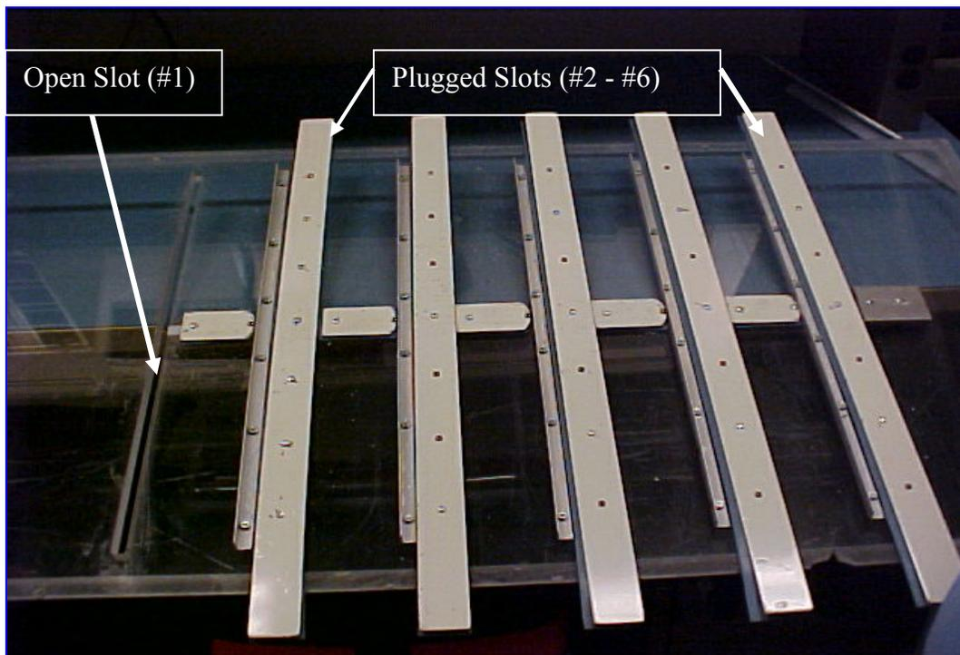
**Figure 22: Removable Plexiglas Top for Hot-wire Anemometry (22)**
