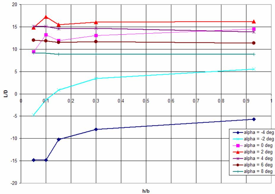
**Figure 50: Lambda UCAV L/D vs. (h/b) 60 mph**
