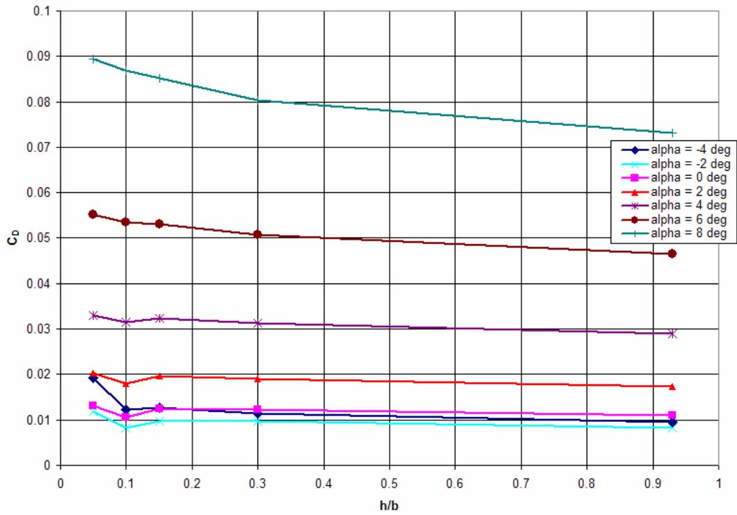
Figure 70: Lambda UCAV  $C_D$  vs. ( $h/b$ ) 80 mph
