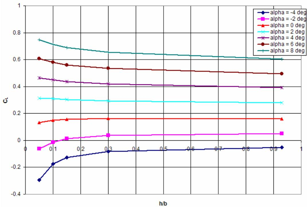
Figure73: Lambda UCAV  $C_L$  vs. ( $h/b$ ) 100 mph
