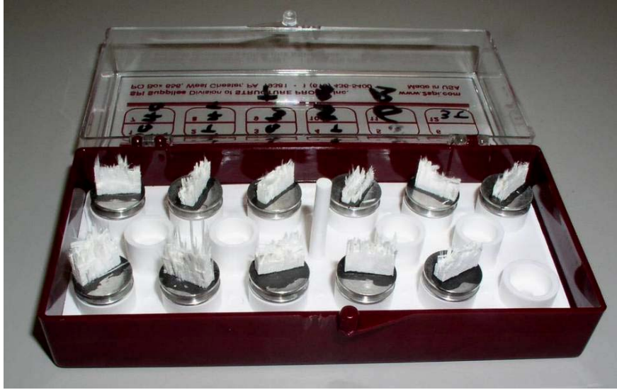
Figure 14. Uncoated N720/A specimens prepared for SEM observation.
