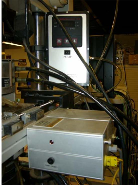
**Figure 15: Water Pump and Steam Heating Unit**
