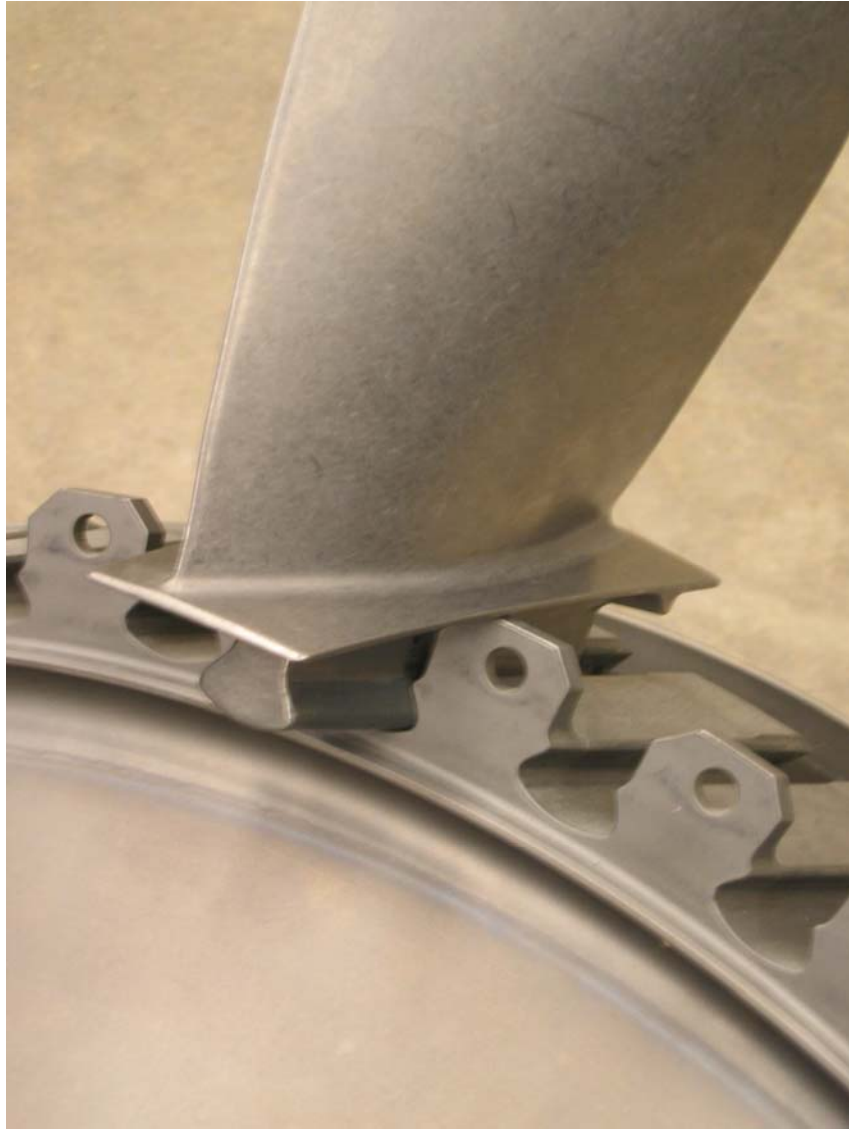
Figure 1. Blade/Disc Dovetail Joint in a Turbine Engine.
