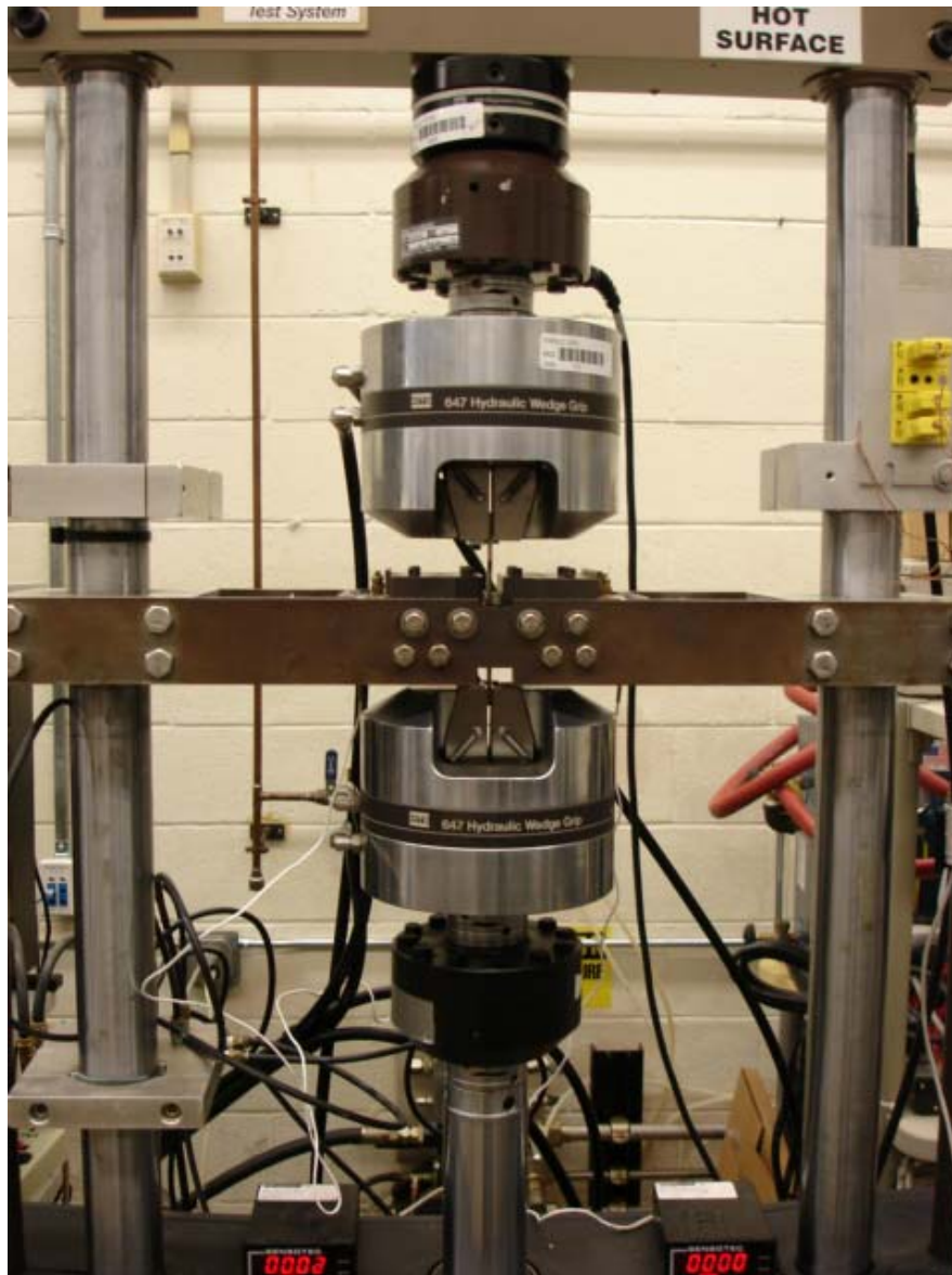
Figure 8. Uni-axial Servo-Hydraulic Material Test Machine with Fretting Fixture
