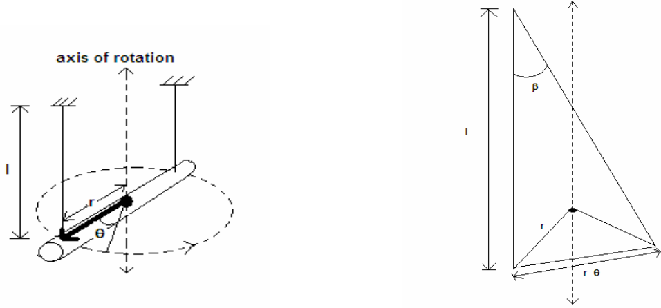
Fig A1. Twist test for a cylinder
