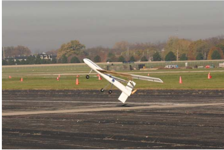
Figure 1. VA-1 Remote-Controlled Joined-Wing Aircraft [29].
