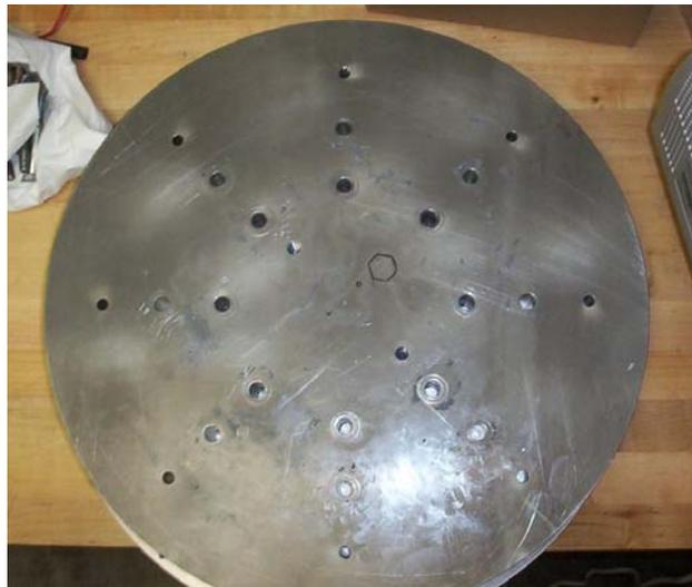
**Figure 16. New 2.5" Thick Aluminum Baseplate, no Constraint Blocks**
