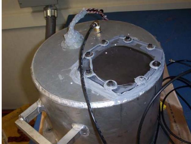
**Figure 25. Window in Top of Pressure Vessel**
