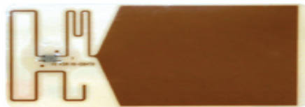
Figure 2: Passive RFID tag [Int04]
