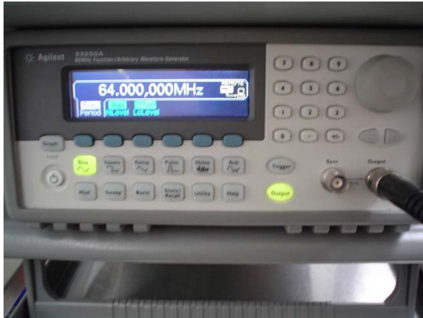
Figure 4.2 Agilent 33250A function generator used in this experiment. The function generator was used to input a sine wave at different frequencies into the cell sample.
