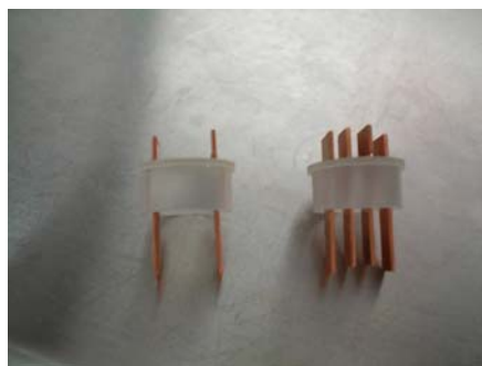
Figure 4.4 Picture of fabricated probe interface. This specific probe interface fits into a 24 sample well (see figure 4.10). Two probe interface types were considered: two leads and four leads. The four lead probe was not used because subsequent experiments found that the two inner probes did not take cell sample measurements but only measured extra-cellular material. This resulted from cells sticking to the bottom of the sample wells, where the middle leads could not properly test.
