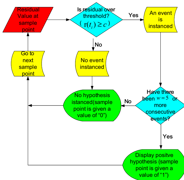
Figure 4.30 Flow diagram describing the process of windowing. Windowing is a method to determine if residuals are consistently above a certain threshold.
