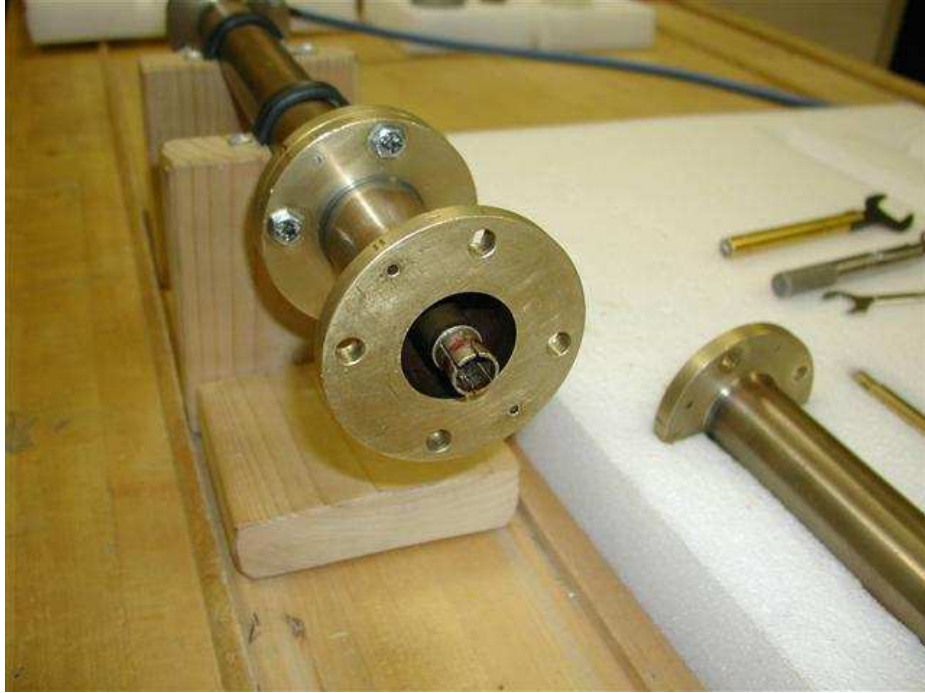
Figure 4.1: Coaxial test fixture opened with center conductor inserted.
