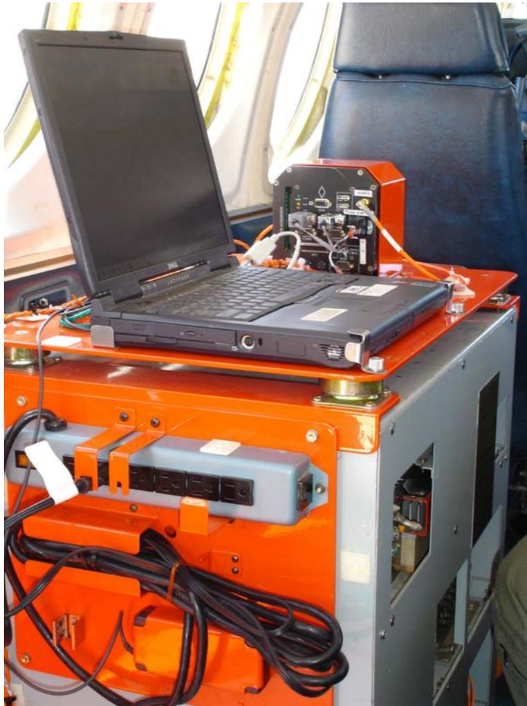
Figure 3.1: Test Unit Installed on C-12
