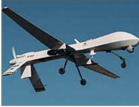
Figure 1.3: The Predator UAV is a long endurance, medium altitude platform that can operate in both reconnaissance and attack missions. [2]
