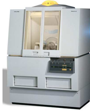
Figure 4.7: Xpert Pro system used for all the x-ray diffraction measurements
