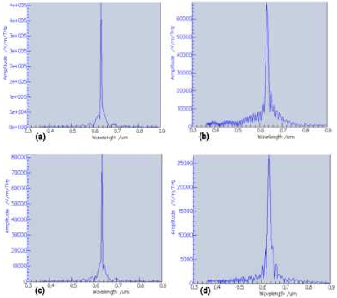
Figure 5.15: The amplitudes of (a) the reference  $E_x$  field (b) the transmitted  $E_x$  field (c) the reference  $E_z$  field, and (d) the transmitted  $E_z$  field, all at  $10^\circ$  incidence on the gold channel.
