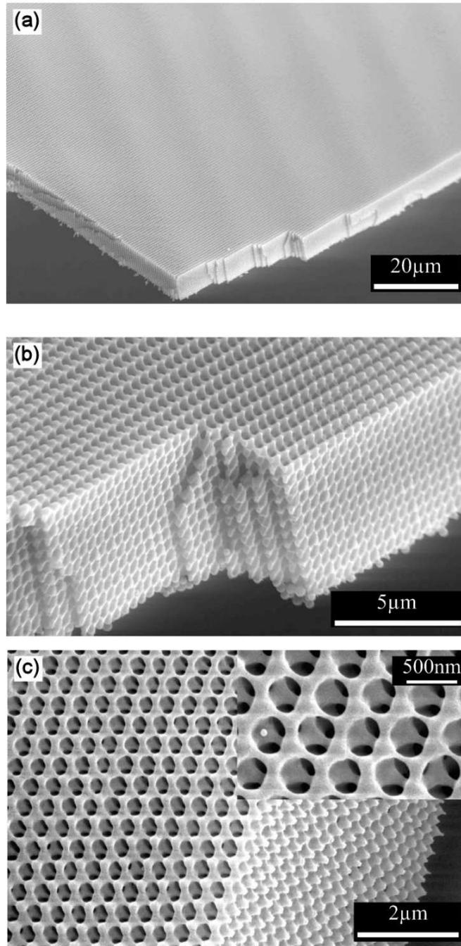
Figure 2.11: SEM image of sample produced with holographic techniques in photo-resist, where (a) shows the structure with a  $20\text{-}\mu\text{m}$  scale, (b) shows the structure with a  $5\text{-}\mu\text{m}$  scale and (c) shows the structure with a  $2\text{-}\mu\text{m}$  scale and an inserted  $500\text{-nm}$  scale [26].
