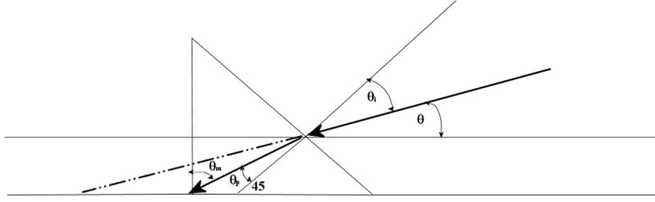
Figure 4.6: Illustration for calculating angles necessary for determining proper prism coupling.
