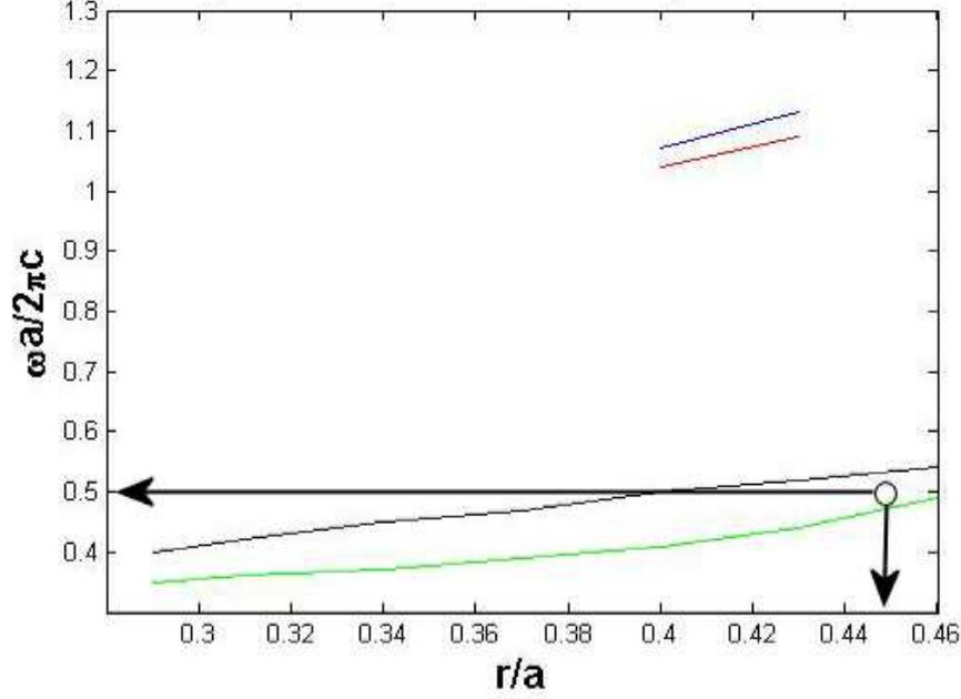
Figure 4.7: Two-dimensional triangular structured PhC gap map of silicon nitride with a periodicity of  $0.35 \mu\text{m}$  and a radius range of  $0.1\text{--}0.175 \mu\text{m}$  designed with columns of air ( $\epsilon = 1$ ) in the silicon nitride ( $\epsilon = 4$ ) where the TM field polarization band gap is shown between the red and blue lines and the TE field polarization band gap is shown between the green and black lines.
