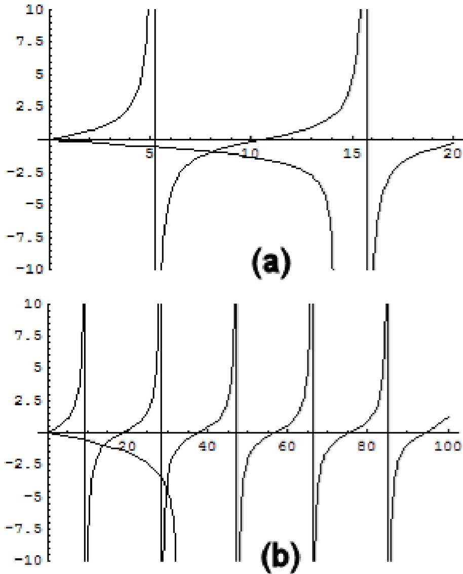
Figure 4.16: (a) Modes supported in  $Al_{0.6}Ga_{0.4}As$  that is 300-nm thick with air on one side and  $Al_{0.98}Ga_{0.02}As$  on the other, (b) modes supported in  $Al_{0.6}Ga_{0.4}As$  that is 300-nm thick with air on both sides.
