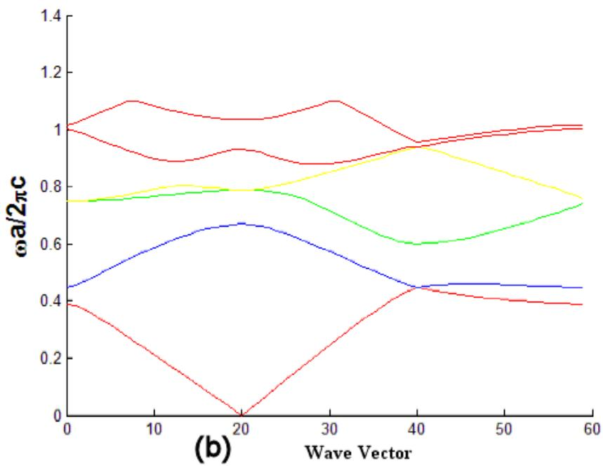
Figure 4.8: (a) Band diagram of E polarization and (b) H polarization for silicon nitride with  $a = 0.3165 \mu\text{m}$  and  $r = 0.1424 \mu\text{m}$ , based on columns of air ( $\epsilon = 1$ ) in the silicon nitride ( $\epsilon = 4$ ). Notice there is no band gap for this case.
