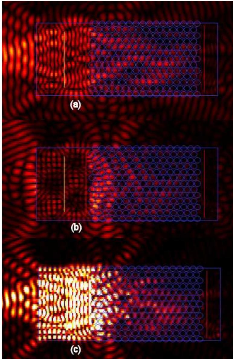
Figure 4.30: PhC design in SU-8 with a periodicity of 320 nm and a column radius of 134 nm excited by a 632.8-nm Gaussian mode at a  $0^\circ$  incidence showing the (a)  $E_x$  field and (b)  $E_z$  field and (c) intensity.
