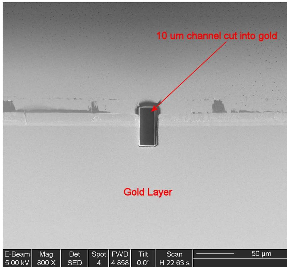
Figure 4.2: SEM image of gold stripe with a 10- $\mu\text{m}$  wide channel cut part way into gold by the FIB.
