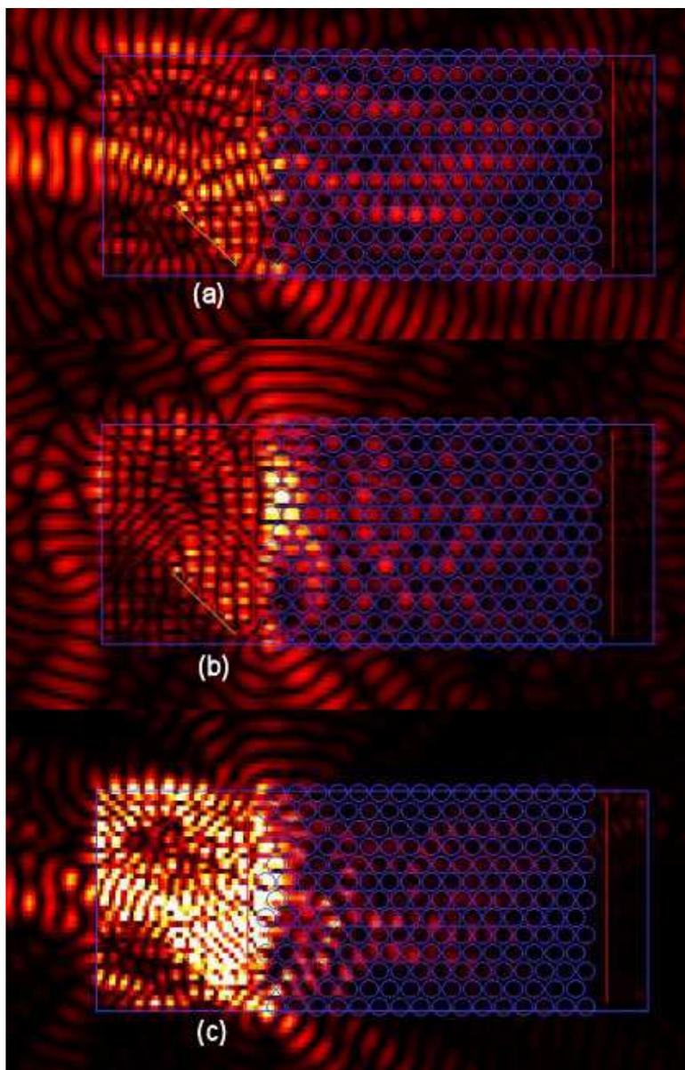
Figure 4.32: PhC design in SU-8 with a periodicity of 320 nm and a column radius of 134 nm excited by a 632.8-nm Gaussian mode at a  $45^\circ$  incidence showing the (a)  $E_x$  field and (b)  $E_z$  field and (c) intensity.
