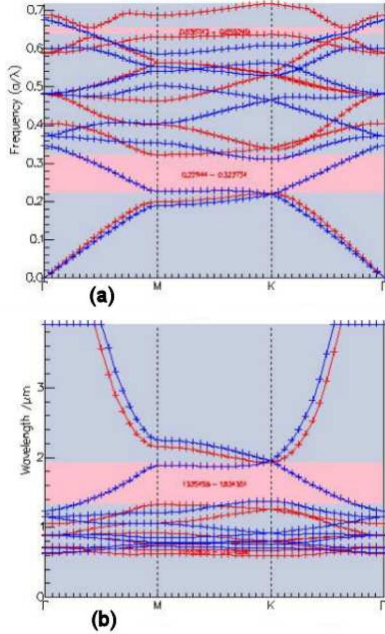
Figure 4.19: Band diagram of  $Al_{0.6}Ga_{0.4}As$  modeled with Crystalwave software for a periodicity of 427.77 nm in a triangular pattern showing two TE band gaps in units of (a) frequency (TE gap of 0.221144-0.322734 and 0.636743-0.655249  $a/\lambda$ ) and (b) wavelength (TE gap of 1.934351-1.325456 and 0.671809-0.652836  $(\mu m)^{-1}$ ).
