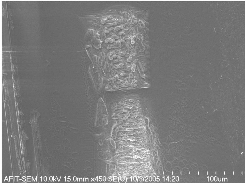
Figure 5.4: SEM image of the attempt to use air as a mask for the beam leaving a 10- $\mu\text{m}$  wide channel. Due to bad drift and re-deposition of material, it can be seen that the FIB process contains too high of charging for this material and the effects of drift cause the results seen here, *i.e.*, a non-usable mess.
