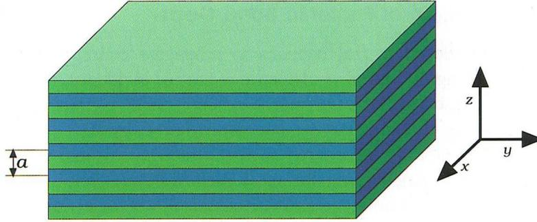
Figure 1.2: One-dimensional crystal, the blue and green represent the different materials of different dielectric constants [12].
