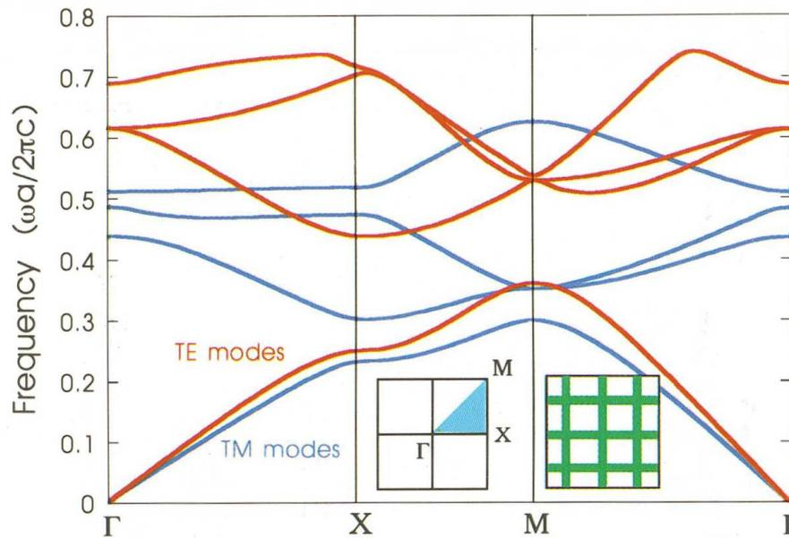
Figure 1.5: Two-dimensional crystal Brillouin zone representation of frequency versus k-space.  $\Gamma$  corresponds to  $k = 0$ ,  $\chi$  corresponds to  $k = (\frac{\pi}{a})x$ , M corresponds to  $k = (\frac{\pi}{a})x + (\frac{\pi}{a})y$ , The inset on the left shows the wave vector with respect to the reciprocal lattice space. The inset on the right shows the reciprocal lattice of the crystal [12].
