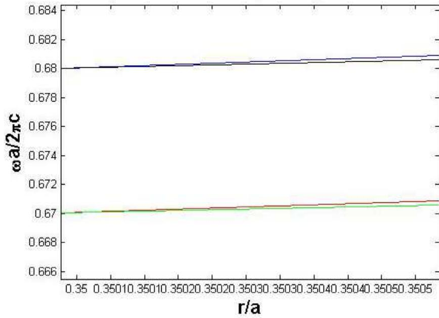
Figure 4.17: Two-dimensional triangular PhC gap map for  $Al_{0.6}Ga_{0.4}As$  with  $a = 1 \mu\text{m}$  and  $r = 0.34 - 0.38 \mu\text{m}$ , based on columns of air ( $\epsilon = 1$ ) in  $Al_{0.6}Ga_{0.4}As$  ( $\epsilon = 11.94$ ) where the TM field polarization band gap is shown between the red and blue lines and the TE field polarization band gap is shown between the green and black lines, showing a complete band gap for this structure.
