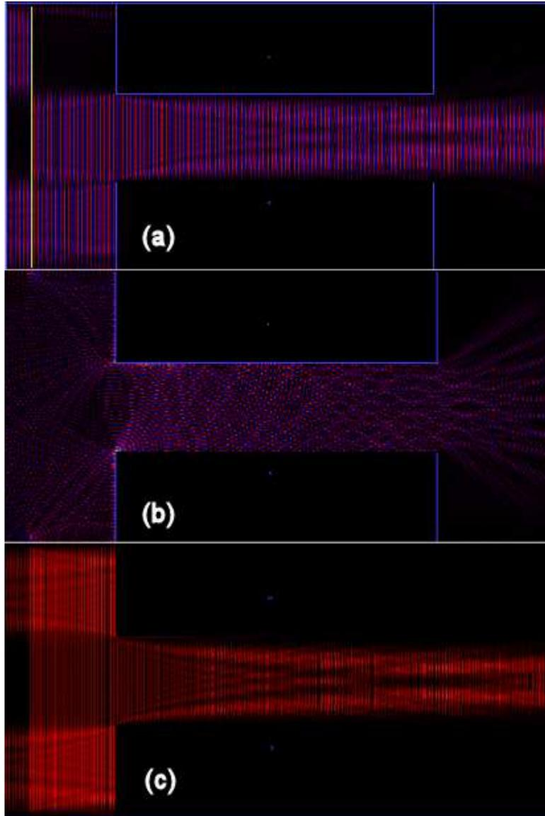
Figure 5.12: Crystalwave modeling results of the coupling of the slab waveguide to the gold channel where (a) is the  $E_x$  field (b) is the  $E_z$  field and (c) is the intensity at a  $0^\circ$  incidence on the gold channel.
