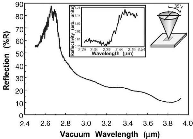
Figure 2.15: Reflectance spectrum at normal incidence of the GLAD fabricated sample in Figure 2.14 [19].
