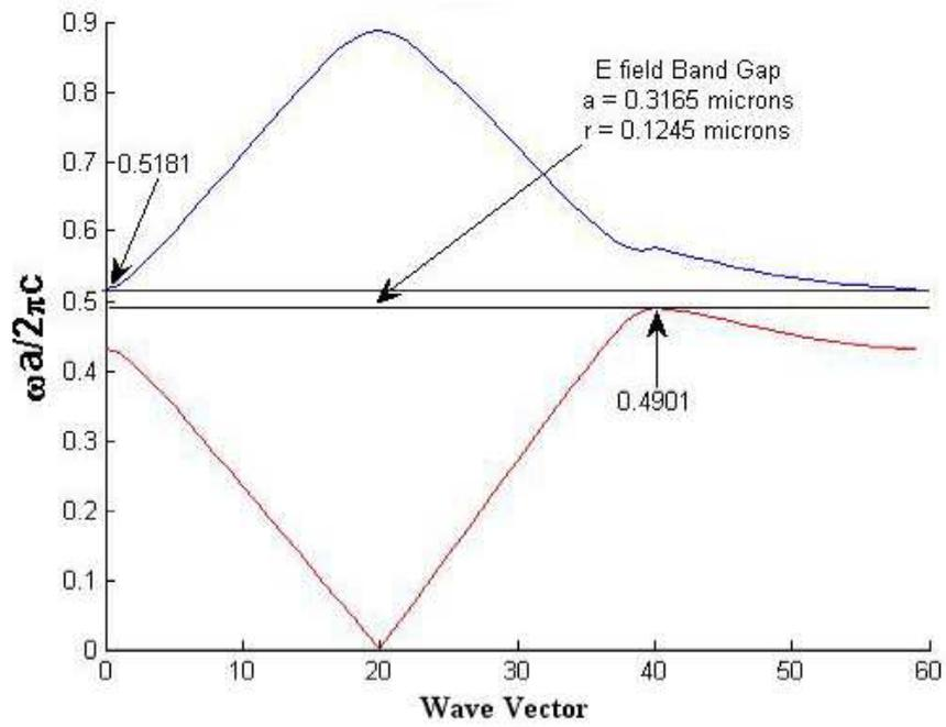
Figure 4.12: Two-dimensional triangular PhC band diagram of APC for a  $1\text{-}\mu\text{m}$  thick layer with  $a = 0.3165$  and  $r = 0.1245$  based on columns of air ( $\epsilon = 1$ ) in APC ( $\epsilon = 2.4649$ ).
