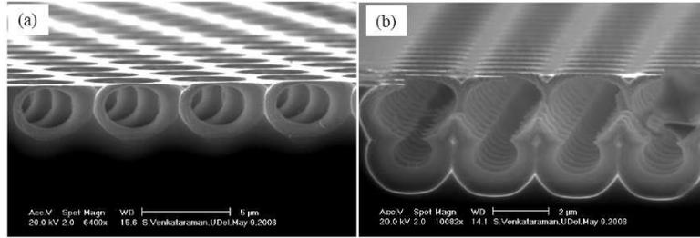
Figure 2.12: SEM image of single-cell and two-layer PhC, using method outlined in Figure 2.10. (a) Shows the results of the first four steps in the novel fabrication technique of Figure 2.10. (b) Shows the results of second four steps in the novel fabrication technique of Figure 2.10 [23].
