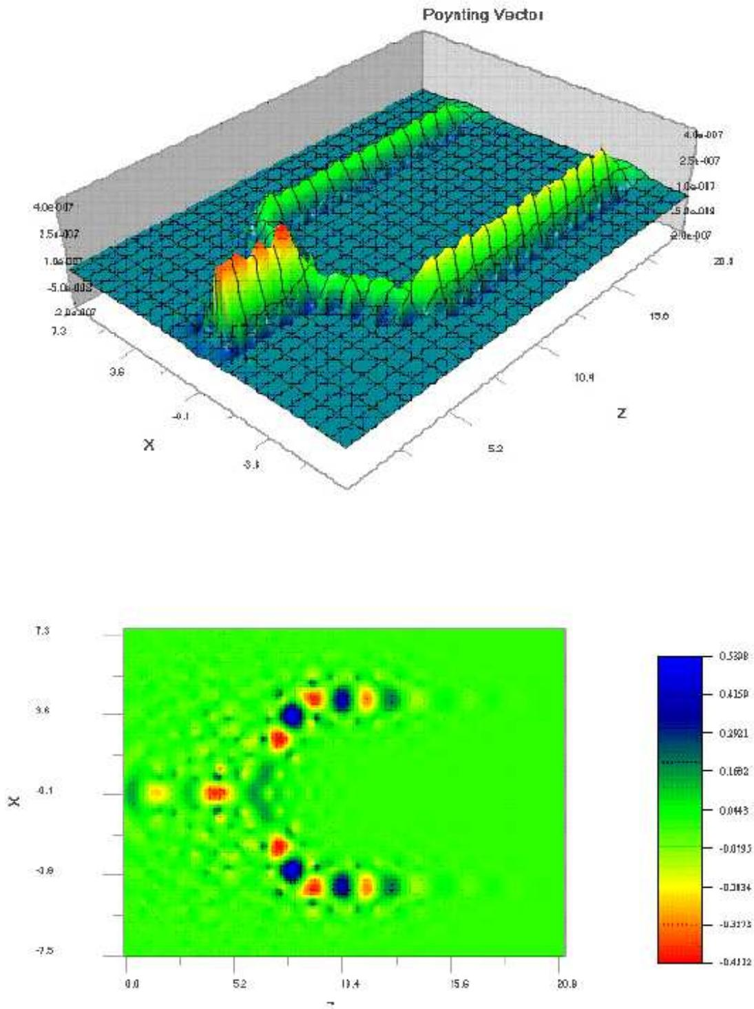
Figure 3.6: Poynting vector (top) and  $E_y$  field (bottom) of Y-split channel depicted in Figure 3.4.
