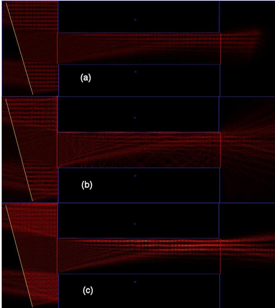
Figure 5.14: Crystalwave modeling results of the coupling of the slab waveguide to the gold channel where (a) is the  $E_x$  field (b) is the  $E_z$  field and (c) is the intensity at a  $10^\circ$  incidence on the gold channel.
