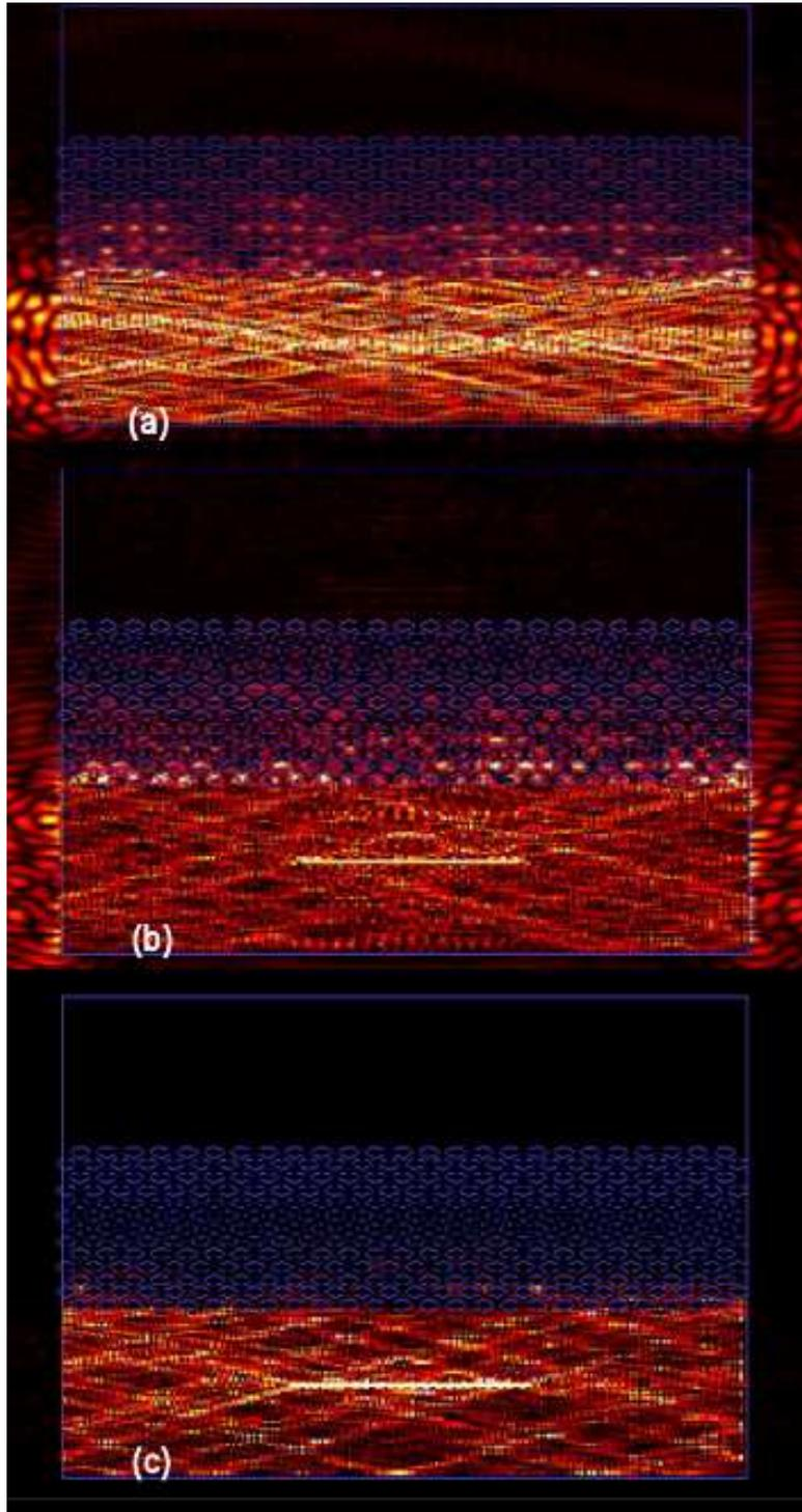
Figure 4.23: FDTD results of a 632.8-nm TE mode exciter at  $0^\circ$  incidence angle with a 200-nm air gap incident on a triangular structure PhC with a periodicity of 427.77 nm and a radius of 149.76 nm for (a) the  $E_x$  field and (b) the  $E_z$  field and (c) the intensity.
