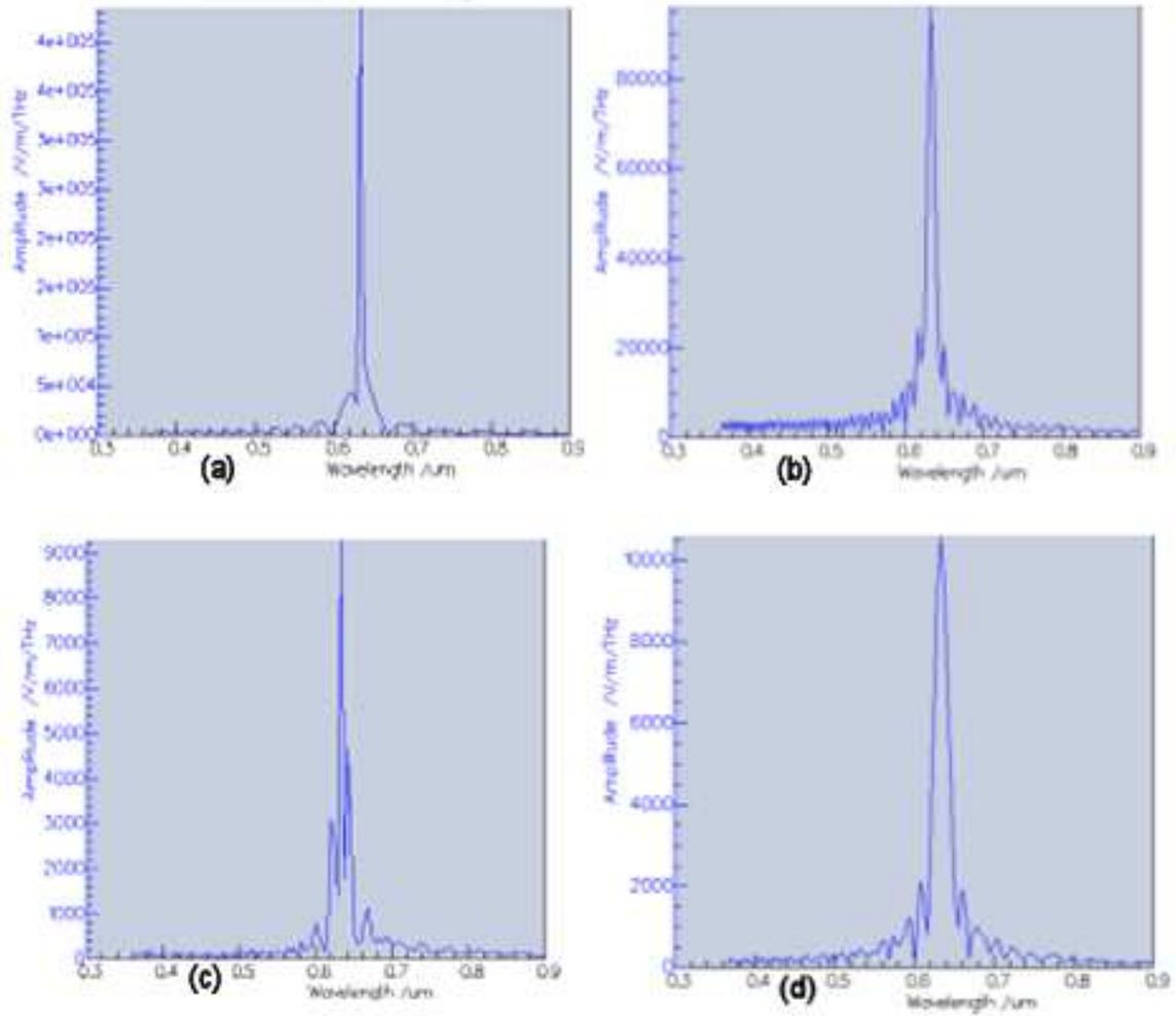
Figure 5.13: The amplitudes of (a) the reference  $E_x$  field (b) the transmitted  $E_x$  field (c) the reference  $E_z$  field (d) the transmitted  $E_z$  field, all at  $0^\circ$  incidence on the gold channel.
