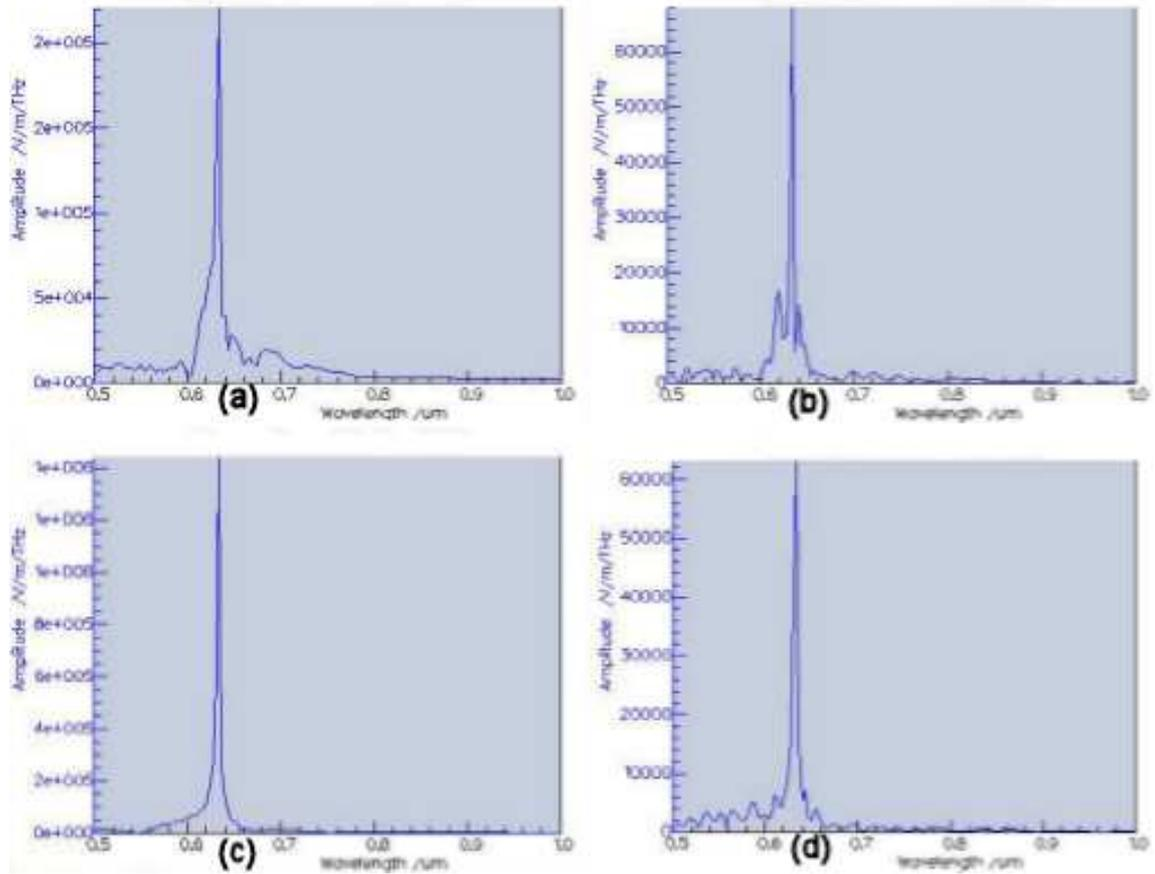
Figure 4.33: PhC design in SU-8 with a periodicity of 320 nm and a column radius of 134 nm excited by a 632.8-nm Gaussian mode at a 45° incidence showing (a) the reference  $E_x$  amplitude and (b) the transmitted  $E_x$  amplitude and (c) the reference  $E_z$  amplitude and (d) the transmitted  $E_z$  amplitude.
