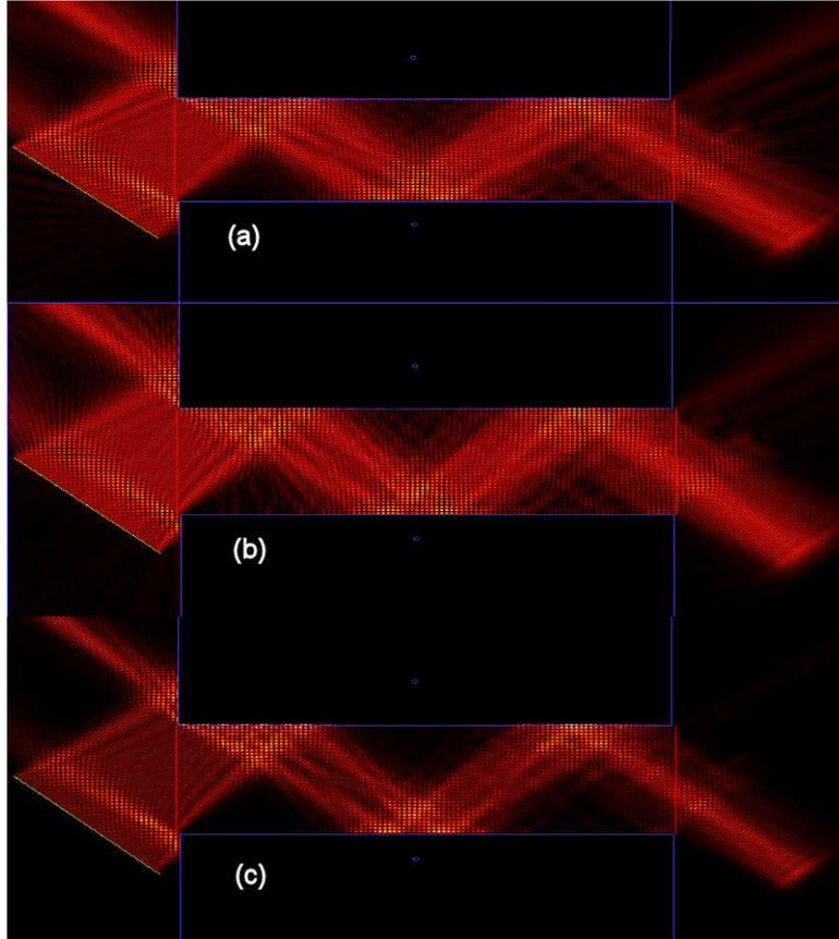
Figure 5.16: Crystalwave modeling results of the coupling of the slab waveguide to the gold channel where (a) is the  $E_x$  field (b) is the  $E_z$  field and (c) is the intensity, all at a  $45^\circ$  incidence on the gold channel.
