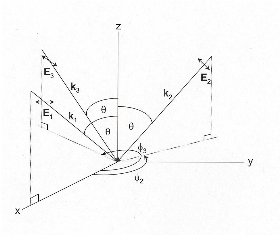
Figure 4.25: Holographic laser beam setup for two-dimensional structures used in this thesis, with the propagation vectors of the three laser beams displayed as  $K_{1-3}$  [20].
