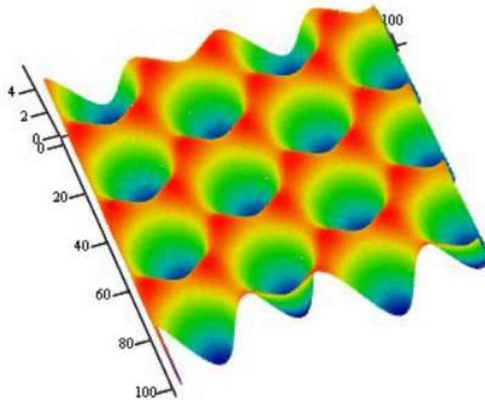
Figure 4.27: Image generated in MATHCAD<sup>®</sup> for  $a = 320$  nm and  $r = 134$  nm in SU-8 photo-resist, created from equations in Appendix E for the holographic laser setup used to create a two-dimensional triangular PhC design, the top and bottom pictures are different perspectives of the same graph.
