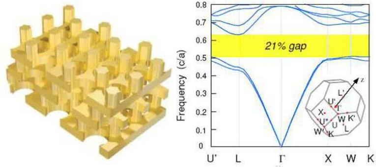
Figure 2.7: Three-dimensional PhC design and associated band diagram [16].
