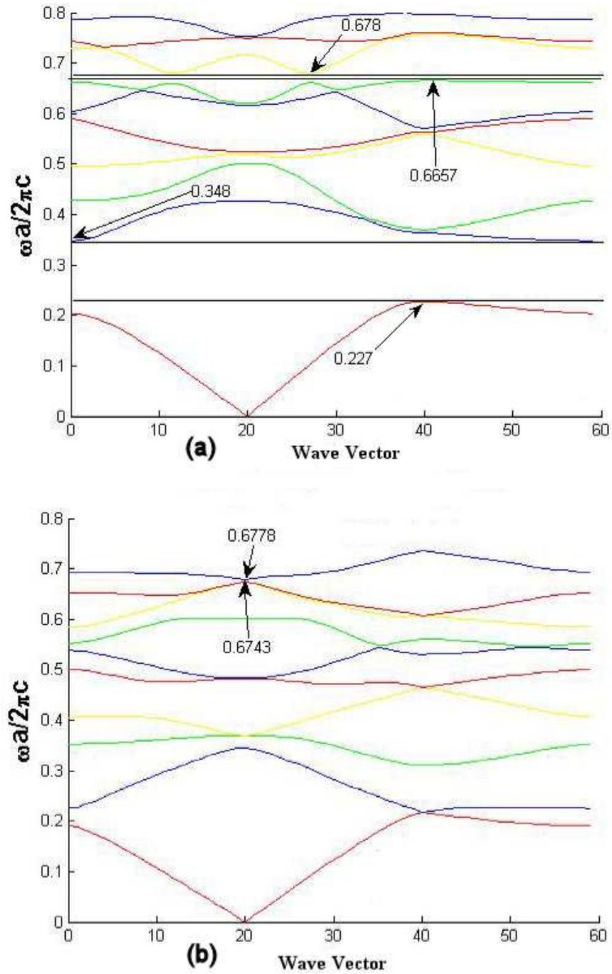
Figure 4.18: Two-dimensional triangular PhC band diagram for  $Al_{0.6}Ga_{0.4}As$  with  $a = 427.77$  nm and  $r = 149.76$  nm, based on columns of air ( $\epsilon = 1$ ) in  $Al_{0.6}Ga_{0.4}As$  ( $\epsilon = 11.94$ ) with the band gaps shown, for (a) E field polarization, and (b) H field polarization.
