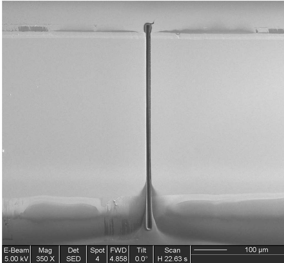
Figure 4.1: SEM image of gold strip with a 10- $\mu\text{m}$  wide channel cut by the FIB.
