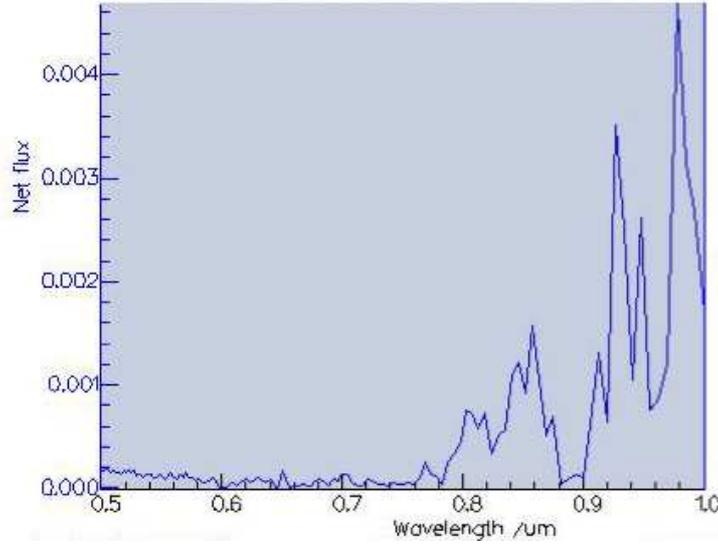
Figure 4.24: FDTD results of a 632.8-nm TE mode exciter net flux at a 45° incidence angle with a 200-nm air gap as a ratio of the transmitted flux to the reference flux on a triangular structure PhC with a periodicity of 427.77 nm and a radius of 149.76 nm.
