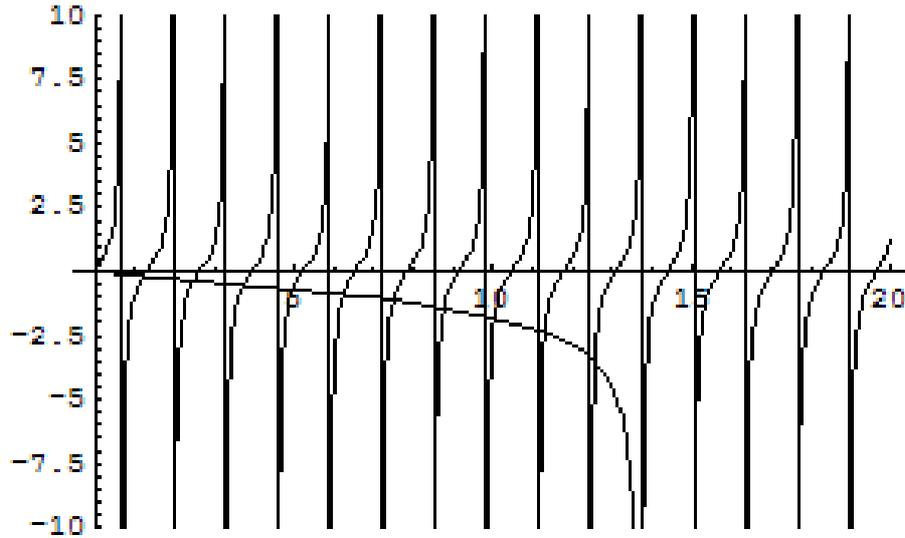
Figure 4.5: MATHEMATICA<sup>®</sup> graph of modes supported in 2.4  $\mu\text{m}$  thick silicon nitride.
