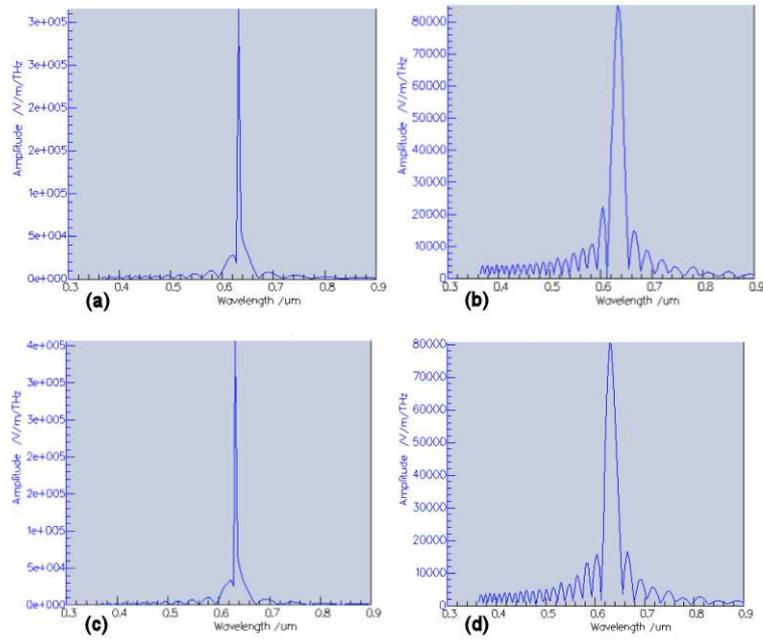
Figure 5.17: The amplitudes of (a) the reference  $E_x$  field (b) the transmitted  $E_x$  field (c) the reference  $E_z$  field, and (d) the transmitted  $E_z$  field, all at  $45^\circ$  incidence on the gold channel.
