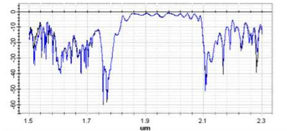
Figure 3.5: Frequency component of the PBG of the Y-split channel depicted in Figure 3.4.
