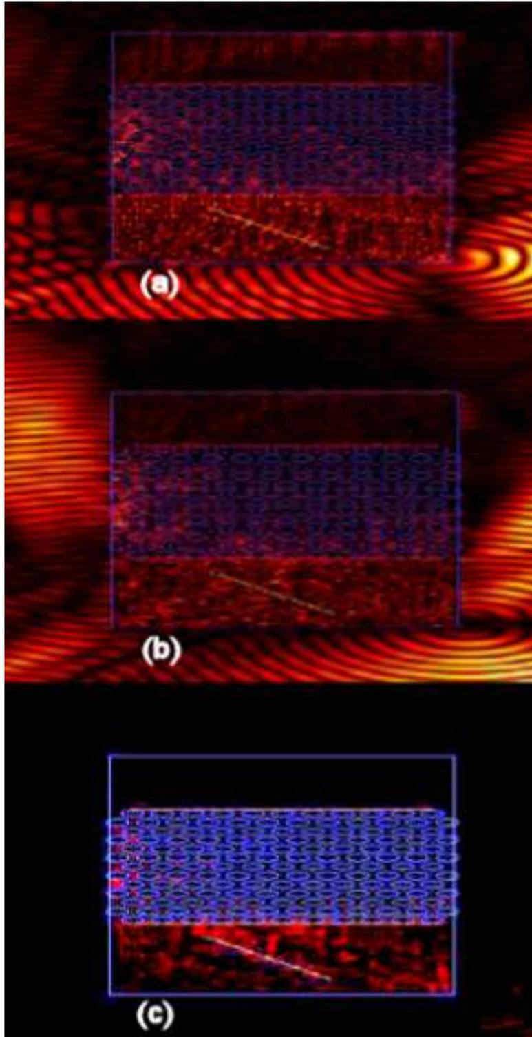
Figure 4.22: FDTD results of a 632.8-nm TE mode exciter at  $45^\circ$  incidence angle with a 500-nm air gap incident on a triangular structure PhC with a periodicity of 427.77 nm and a radius of 149.76 nm for (a) the  $E_x$  field and (b) the  $E_z$  field and (c) the intensity.
