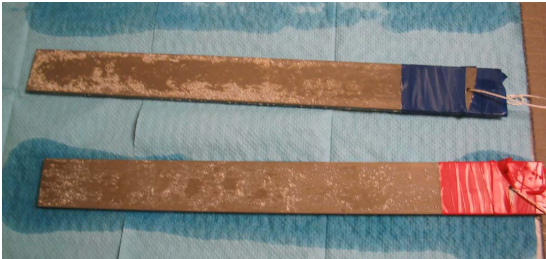
Figure 191. Blue notchless and red middle notched beam after 48 hour corrosion (before cleaning)
