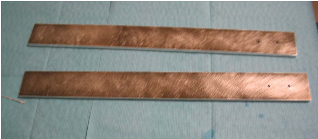
Figure 197. Red notchless beam on top, white/red notched on bottom. Front surfaces before corrosion
