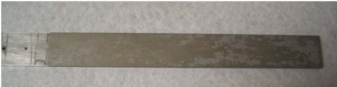
Figure 210. Back of white/red notchless beam after cleaning.
