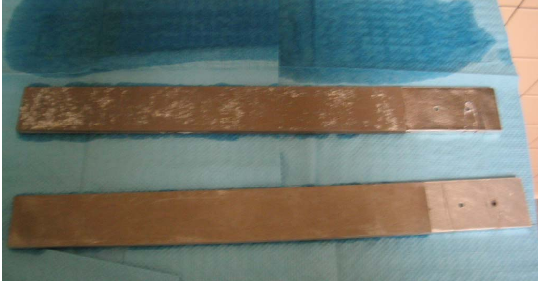
Figure 204. Front of beams after corrosion, before cleaning. Blue/green middle notched beam is on top, White/red notchless beam is on bottom
