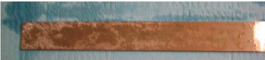
Figure 221. Back of white notchless beam after corrosion and cleaning. Lighter gray areas indicate former presence of Al 2 O 3 deposits.
