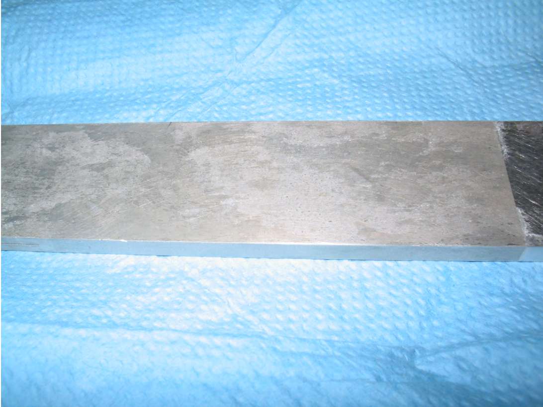
Figure 199. Back of white/red notched beam. Note the presence of pits contained in the lighter areas. Pitting appears to only occur under a region that has previously been covered with salt deposits.
