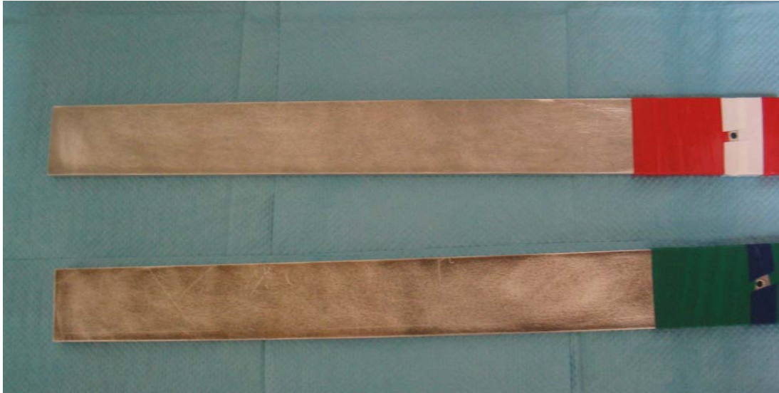
Figure 200. Front of white/red notchless and blue/green middle notched beams before corrosion.
