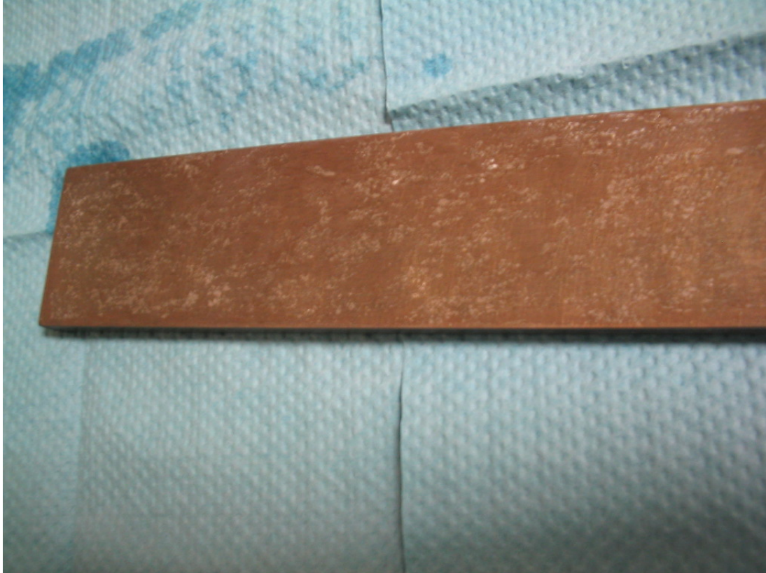
Figure 219. Back of yellow/blue notched beam after corrosion and cleaning
