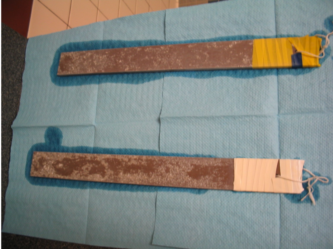
Figure 214. Front of yellow/blue middle beam, back of white notchless beam after corrosion, before cleaning
