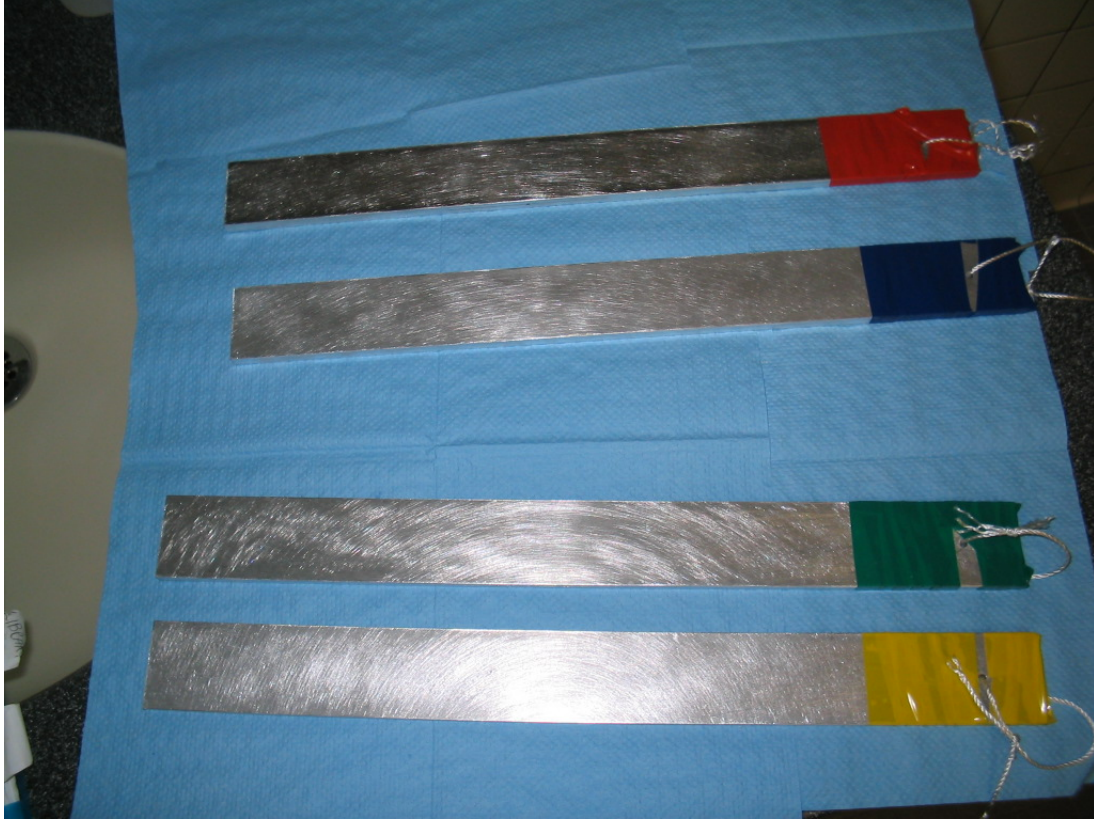
Figure 182. 24 hour and 48 hour beams before immersion. Yellow (notchless) and green (middle notched) beams will be corroded for 24 hours, blue (notchless) and red (middle notched) beams will be corroded for 48 hours.
