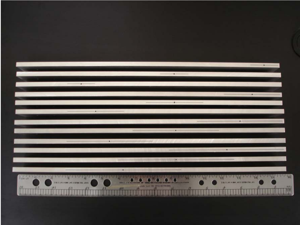
Figure 6. Centrally notched beams. From top to bottom: 4 cm (1.575 in) free end notch, 4 cm (1.575 in) middle notch, 4 cm (1.575 in) clamped end notch, 8 cm (3.150 in) free end notch, 8 cm (3.150 in) middle notch, 8 cm (3.150 in) clamped end notch, 12 cm (4.724 in) free end notch, 12 cm (4.724 in) middle notch, 12 cm (4.724 in) clamped end notch, 16 cm (6.299 in) free end notch, 16 cm (6.299 in) middle notch, 16 cm (6.299 in) clamped end notch.
