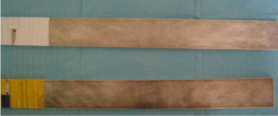
Figure 212. Back of white notchless and yellow/blue middle notched beams before corrosion
