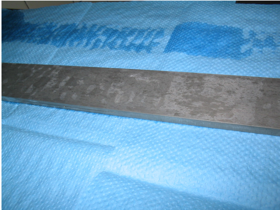
Figure 195. Back of corroded and cleaned red notched beam
