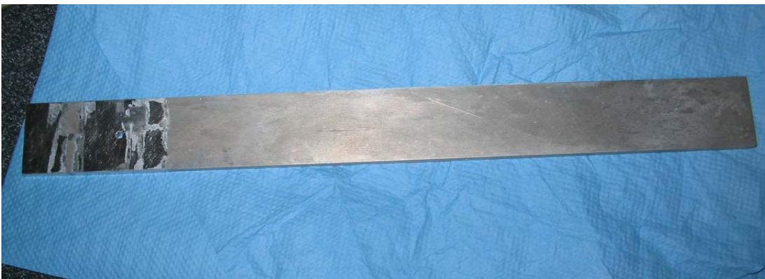
Figure 208. Back of blue/green notched beam after cleaning.
