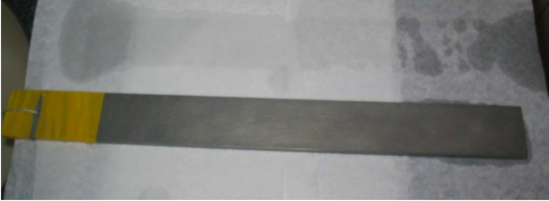
Figure 188. Back of yellow notchless beam-not salt deposits evident
