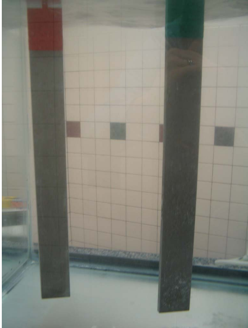
Figure 203. Very few salt deposits present on this side of both beams
