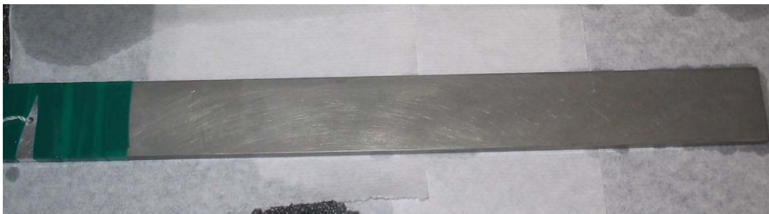
Figure 187. Back of green notched beam-no salt deposits present
