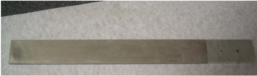
Figure 209. Front of white/red notchless beam after cleaning
