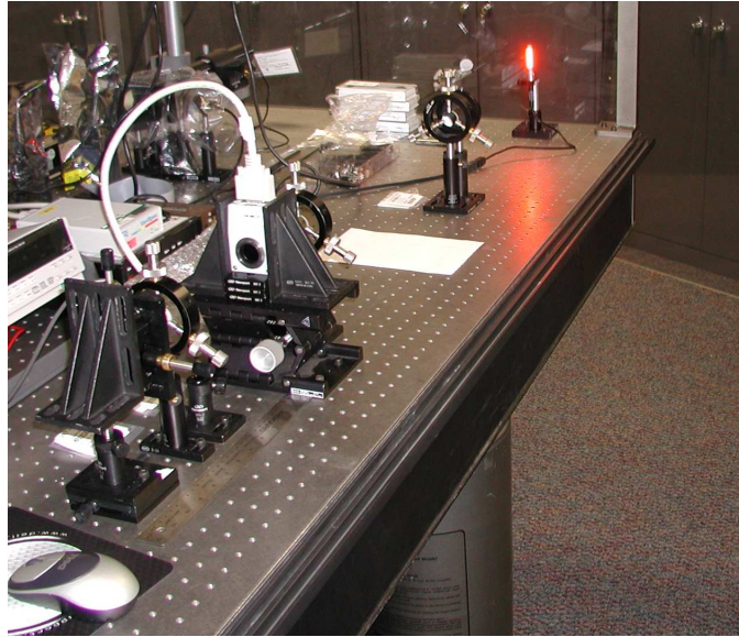
Figure 4.29: The experimental set-up of ASIR-TB for testing the MBSIR algorithm. The system used three lenses to demagnify the spectral source 50 times, while passing collimated light through the LCTF. The source is located at the end of the optics bench, at the top right of the figure.
