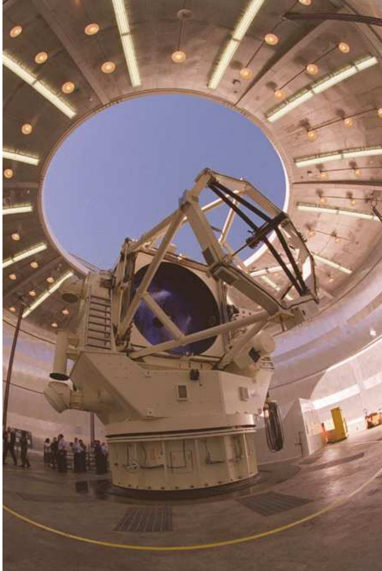
Figure 4.1: The Advanced Electro-Optical System (AEOS). AEOS is the entrance aperture for ASIS.
