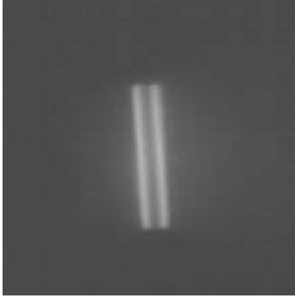
Figure 4.33: An image of the two filament like areas of the Newport/Oriel Hg(Ar) pencil lamp. The image was captured through the LCTF with a selected center wavelength of 546nm. The Ne source looks similar when imaged with the NIR filter.
