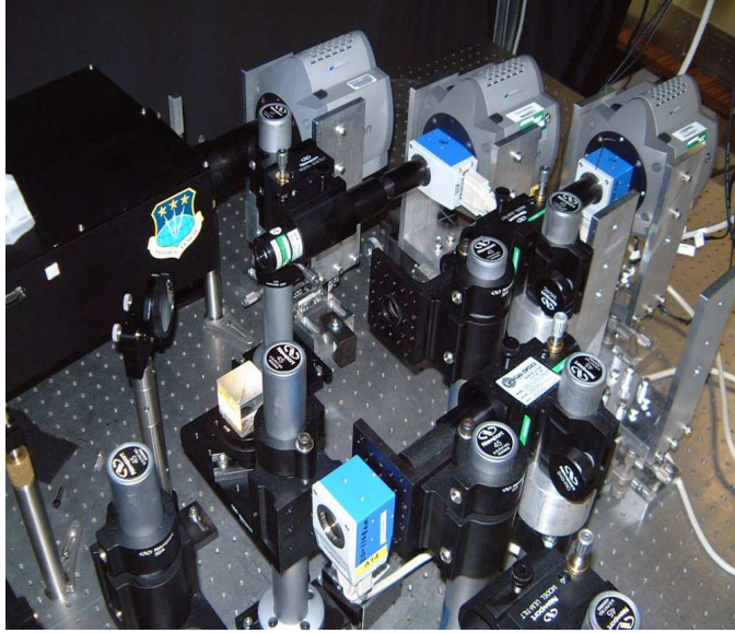
Figure 4.2: Picture of the ASIS optics after the AO bench. The two cameras to the right of the picture are the ASIS visible imaging channels. The blue cubes attached to the cameras are the visible LCTFs. The additional LCTF at the bottom of the picture is the NIR LCTF.
