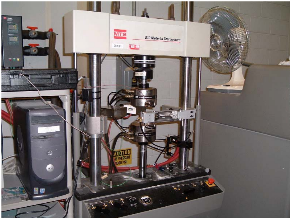
Figure 13: 3 KIP MTS Hydraulic Machine
