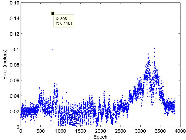
Figure 4.8: 3-D error for the road test using method 1 in early testing. Large spike corresponds to a incorrectly initialized ambiguity.
