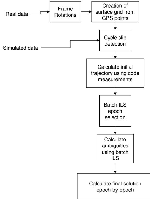
Figure 3.6: Block diagram of overall algorithm process.
