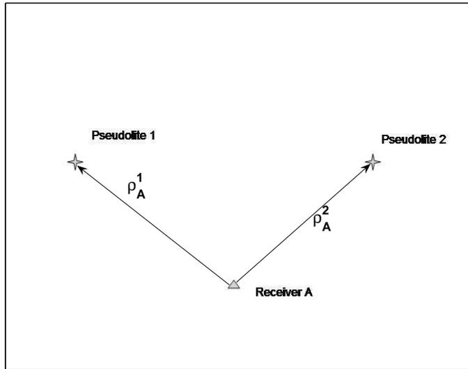
Figure 2.1: Single Difference Between Receiver A and Pseudolites 1 and 2
