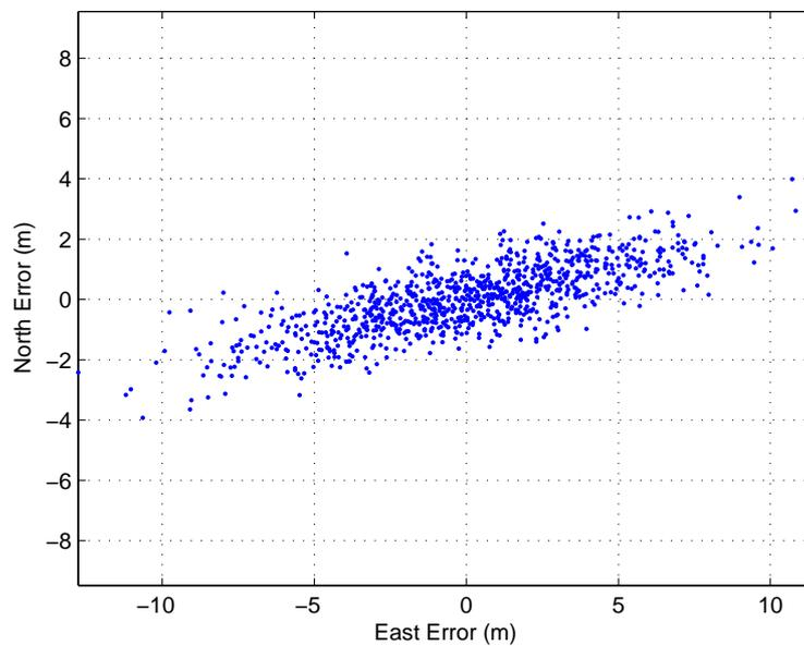
Figure 1.2: Horizontal position estimation errors with no aiding.
