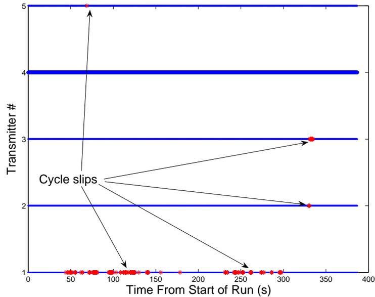
Figure 3.5: Plot of each transmitter and the cycle slips for each. Other than number 4, each transmitter experiences at least one cycle slip.
