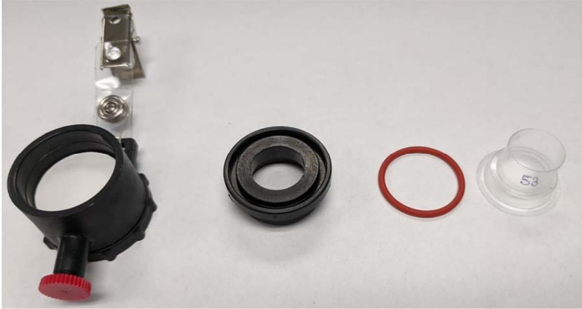
**Figure 22. IOM Disassembled and Ready for Equilibration**
