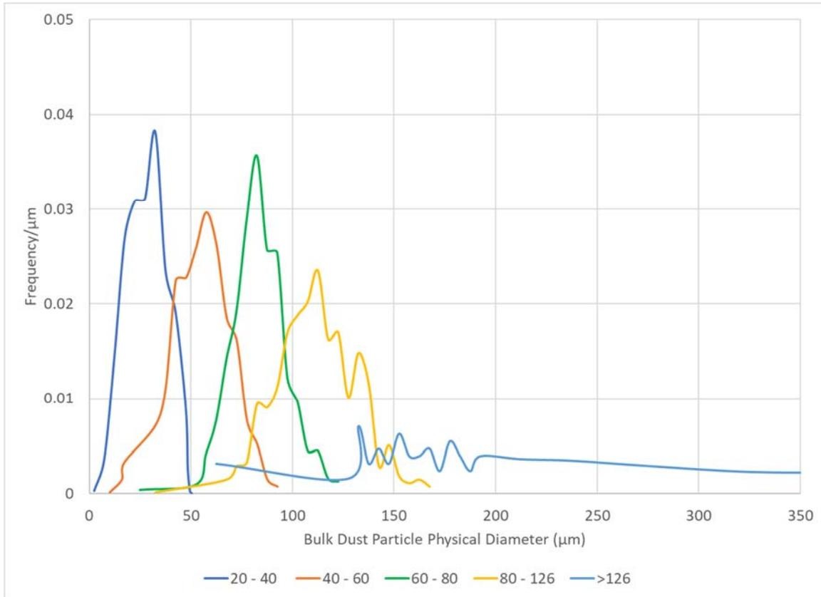
**Figure 18. Size Distribution for Each Sieve Fraction**
