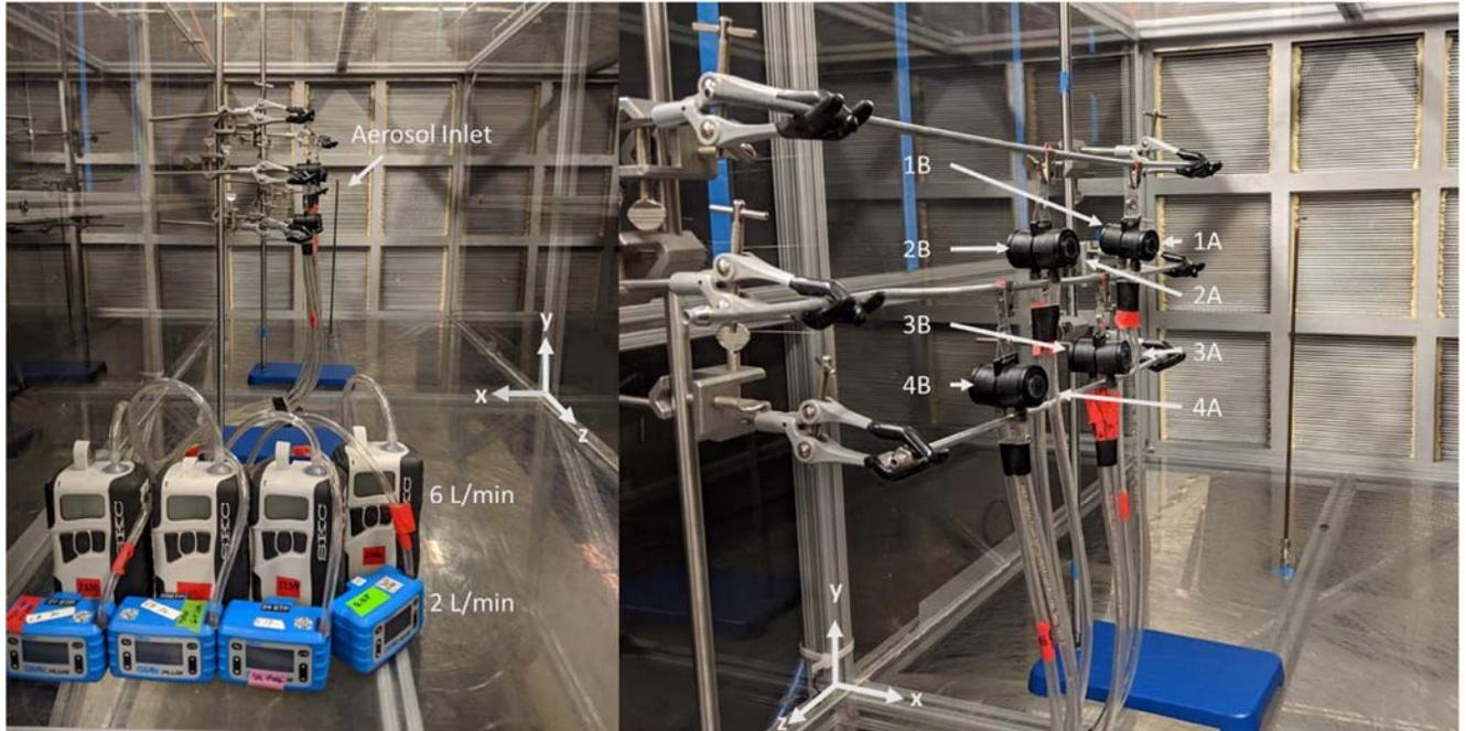
**Figure 25. Final Experiment Setup in Aerosol Chamber**
