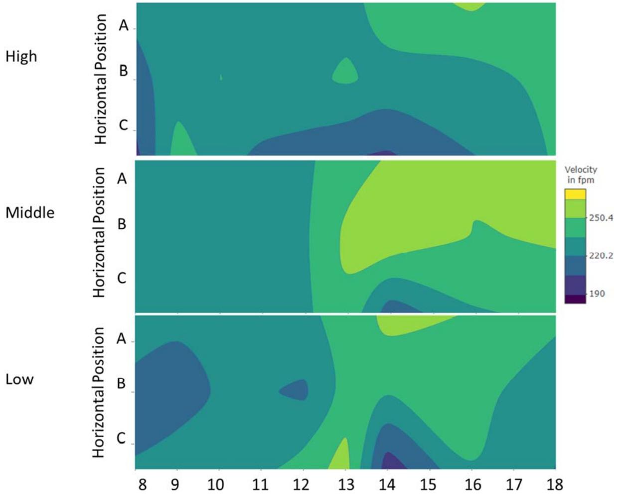
**Figure D4. Vertical Velocity Profile of the Chamber at 60 Hz, with Flow
