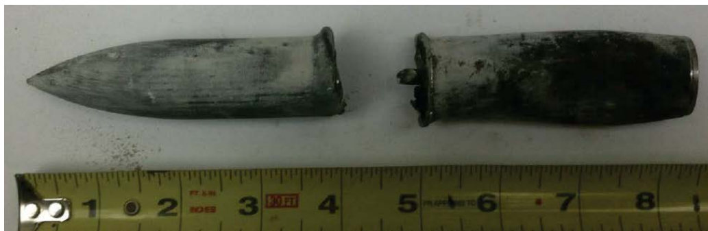
Figure 5. The projectile failed at the midpoint of the shaft after the transition from dense lattice to sparse lattice.
