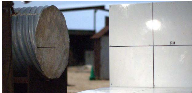
Figure 3. The concrete target Richards used was not reinforced and was contained by a thin cylindrical outer layer of steel.
