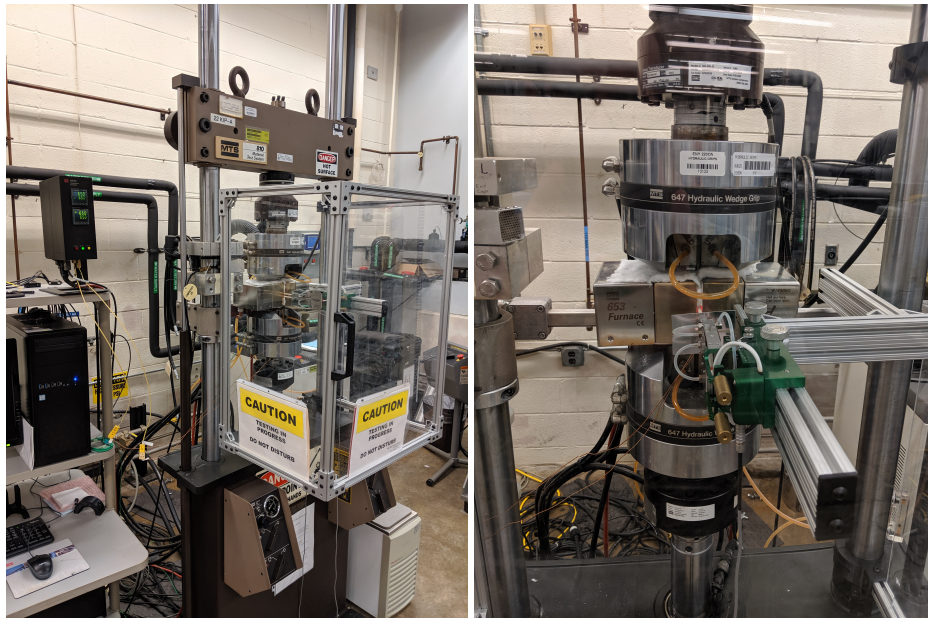
Figure 4.6: A creep-rupture experiment is underway on the MTS 810 servo hydraulic machine. Also shown are the MTS 653 heater and Epsilon extensometer. A protective enclosure is in place to minimize airflow during the test, as well as to prevent accidental interference with the experiment.
