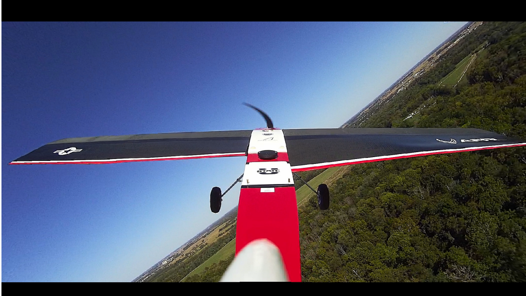
Figure 27: The VCCW shows anti-symmetric trailing edge deflection. The right ribs are deflecting the edge down. The deflection changes cause the wind to blow over the wing creating lift on the wing to control the aircraft.
