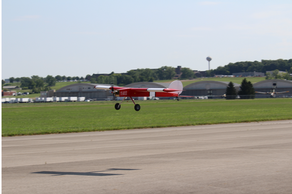
Figure 26: Base wing during take off. The base wing has all of the standard control capabilities: aileron, elevator, and rudder. The fuselage is designed to use either the base wing or VCCW.
