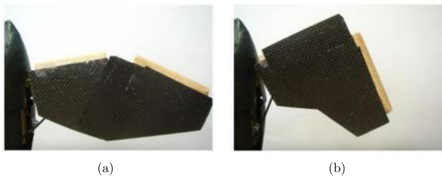
Figure 2: The expandable wing changes its aspect ratio. (a) shows the wing in its expanded state and (b) shows the wing in folded state. The aspect ratio changes from 4.7 to 8.5 in two seconds which decreases drag significantly.
