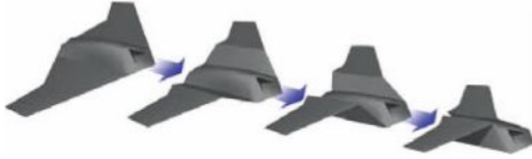
Figure 7: Lockheed-Martin developed Z-wing morphing. The aircraft has the ability to fold its wings toward the center to change the aircraft from a long-range flight to high speed dash and kill and back.
