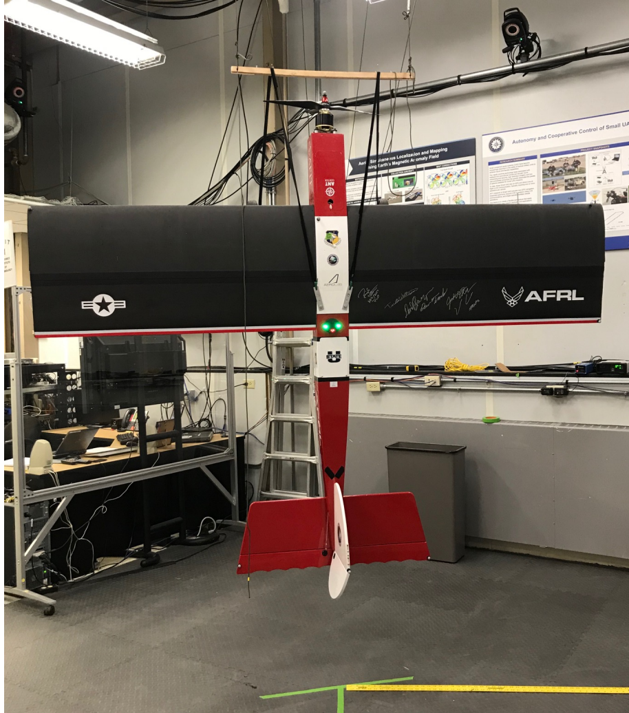
Figure 25: Testing on the VCCW occurred after all the flight test were completed. The aircraft is in the roll configuration and suspended by the fuselage to prevent damage to the wing. One of the Vicon cameras is shown in the top right corner. The 15° rotation marker is shown below the aircraft.
