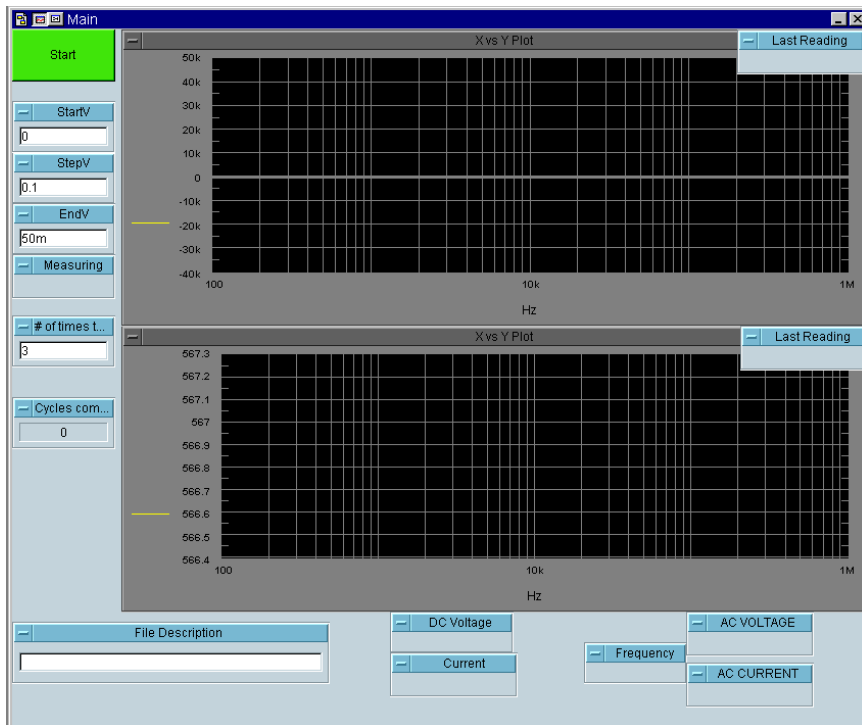
Figure A.4: Small signal frequency response test setup to measure inductance, capacitance and resistance.
