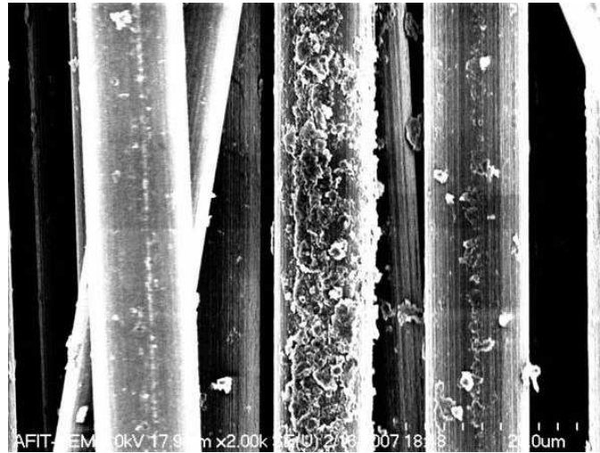
Figure 5.7: Sample F6 shows rutting on the surface in the wide view image of some of the fibers and yet another with a roughened surface that looks like it was in the early stages of delamination of the outer surface
