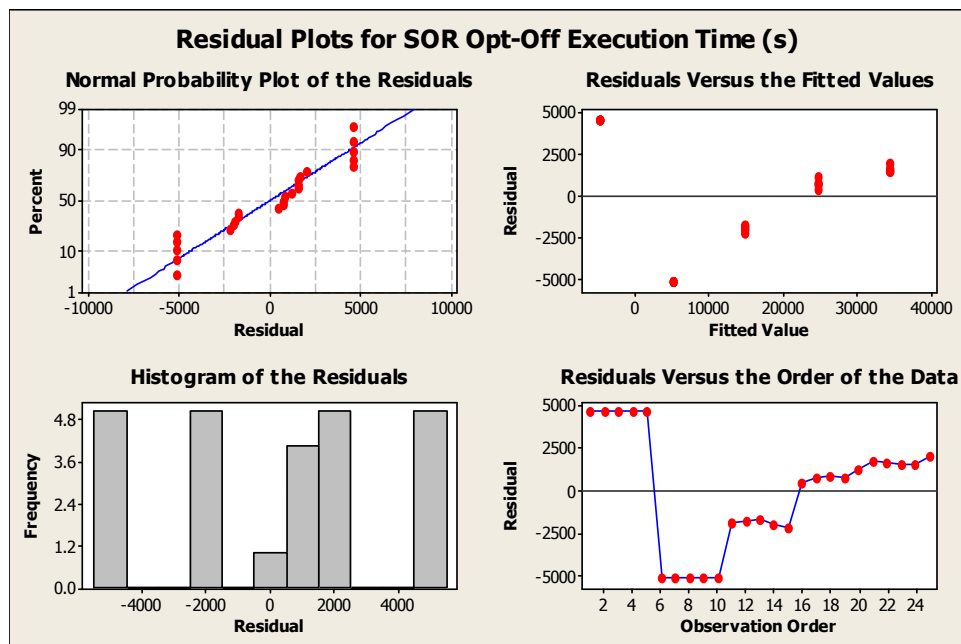
Figure A.24. 4-in-1 Plot for SOR with OllyDbg and Optimization Off, Levels 1-5
