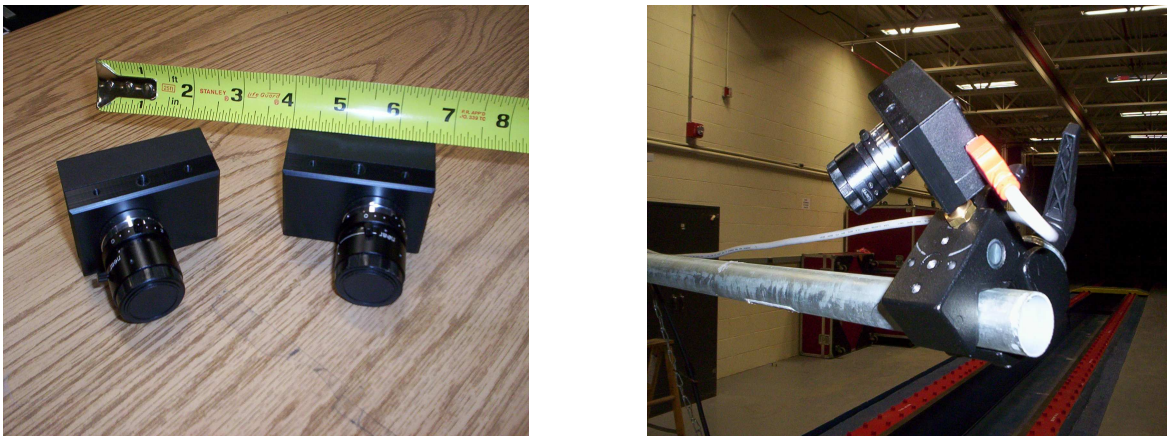
Figure 8: CCD Cameras and Camera Baseline Rod. CCD cameras and their relative size (left). CCD camera mounted on the baseline rod and attached to the IEEE 1394 fire wire.
