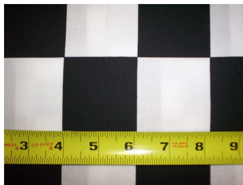
Figure 18: Calibration Checkerboard Dimensions. Squares are 53.975 mm x 53.975 mm on each side.
