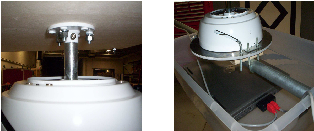
Figure 7: Modified Ceiling Fan. Left image shows the fan attachment to the bottom of the base platform. Right image shows the circular base plate added to the fan with U-clamps to hold the 10 ft. camera rod.
