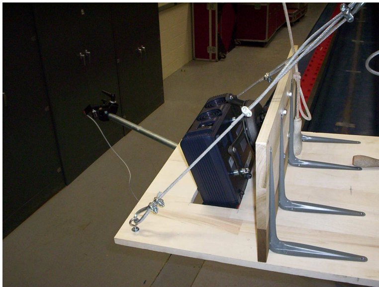
Figure 11: Digital Projector. BenQ PB6200 projector mounted to the vertical support. Cutout shown in the base platform allows for adjustments to the projector field of transmission.
