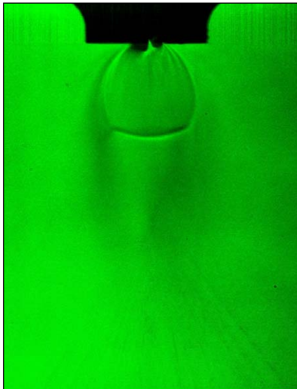
Figure 32. Shadowgraph image, ethylene, nozzle #1, d = 0.5\text{mm} , T_r = 1.01 , P_r = 1.03
