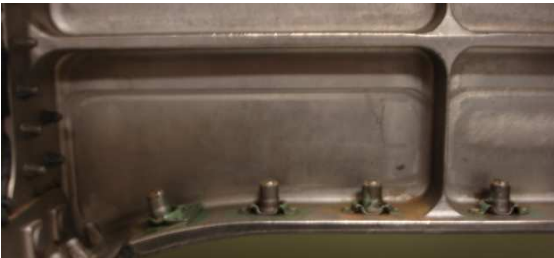
Figure 2.12 F-15 bulkhead: closeup of undamaged bulkhead where damage occurred
