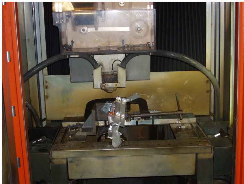
Figure 2.16 F-15: arrangement of F-15 specimen in EDM machine for first cut
