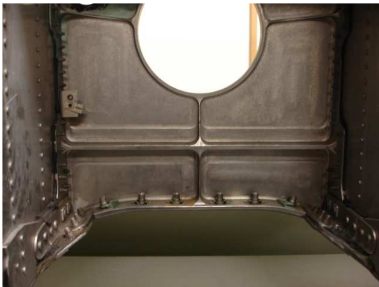
Figure 1.4 F-15 bulkhead: undamaged bulkhead provided to AFIT
