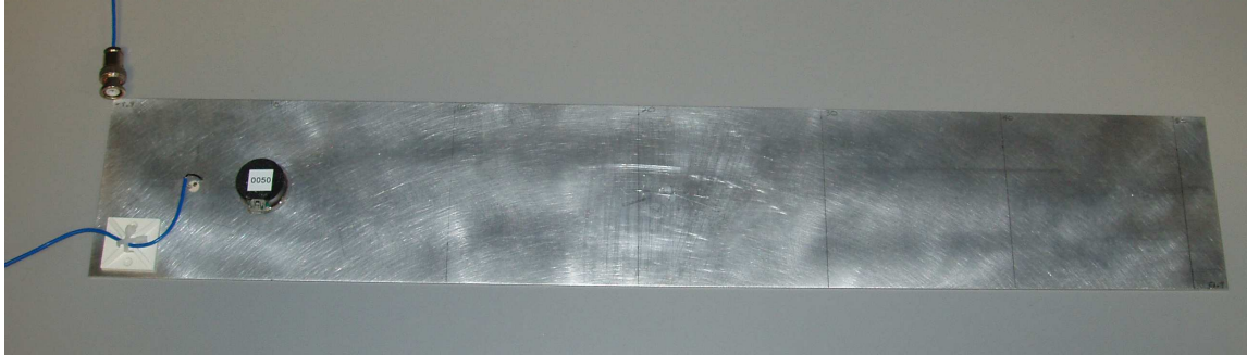
Figure 2.1 Small plate: aluminum plate with attached sensors
