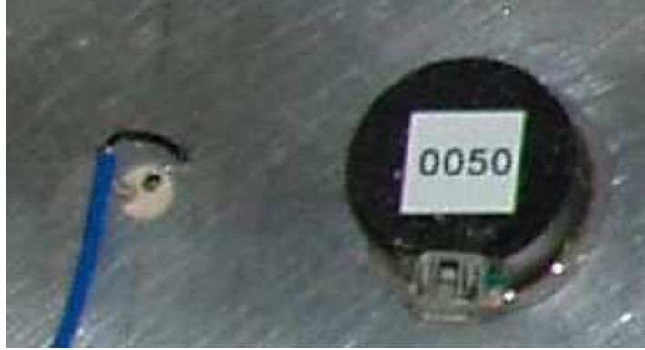
Figure 2.2 Small plate: closeup of attached APC 850 and M.E.T.I.-Disk 3 sensors
