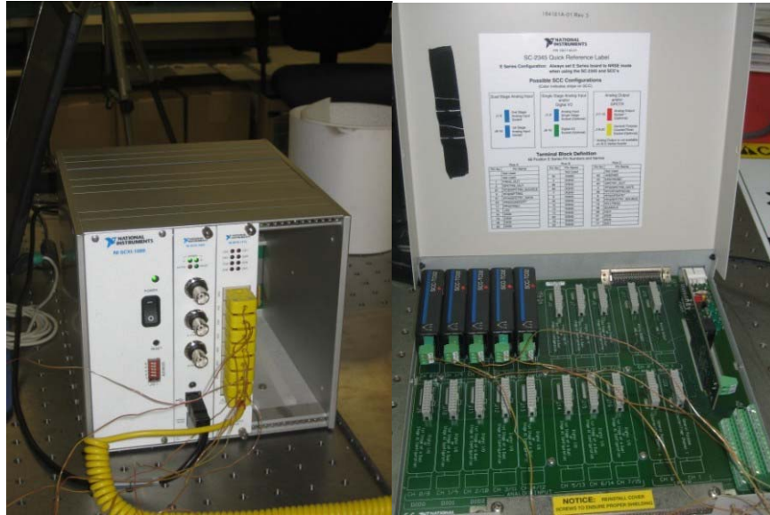
Figure 27: National Instruments (17) Multi-input Type-K Thermocouple Interfaces
