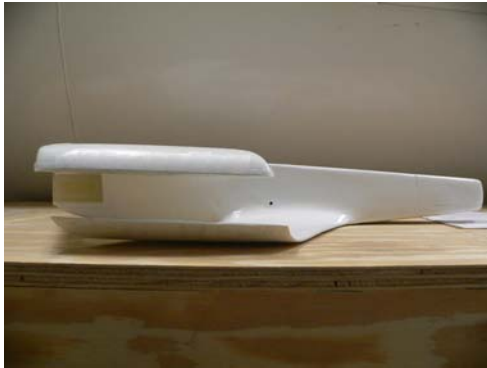
Figure 18: 24" Houck Configuration with 2" Cut in Flow Guide
