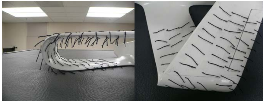
Figure 29: Tufts on 24” Houck Configuration for Flow Visualization
