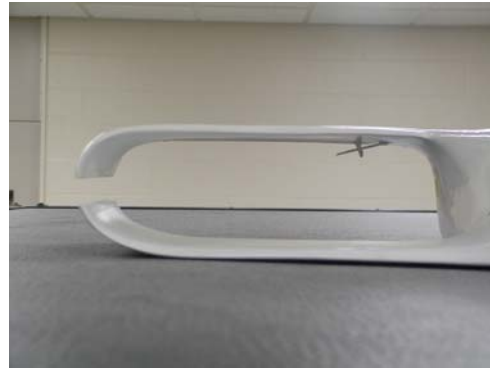
Figure 17: 24" Houck Configuration with 1" Cut in Flow Guide
