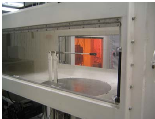
Figure 22: Test Section, Sting Mechanism, and Balance
