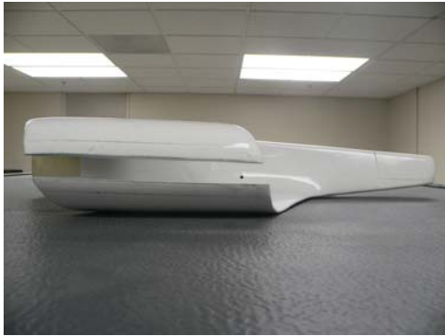
Figure 17: 24" Houck Configuration with 1" Cut in Flow Guide
