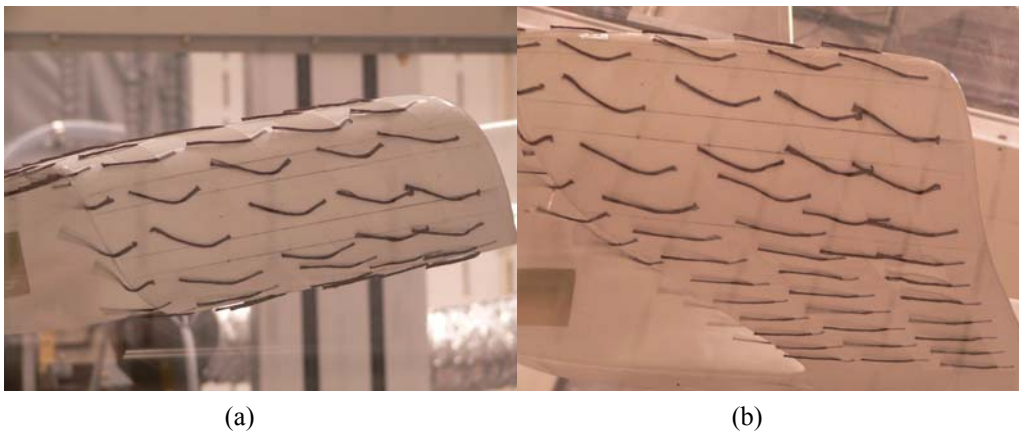
Figure 32: Flow Visualization of 24" Houck Configuration at 50 mph, 8.22° AoA
