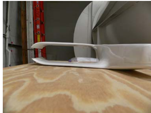
Figure 18: 24" Houck Configuration with 2" Cut in Flow Guide
