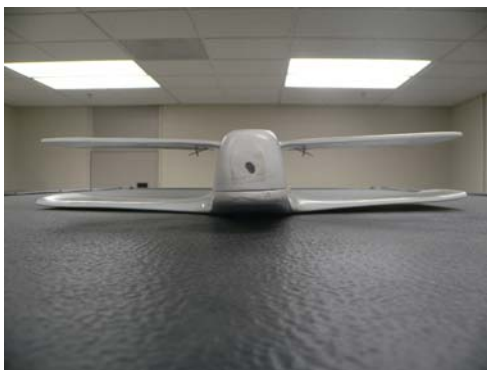
Figure 19: 24" Houck Configuration with No Flow Guides
