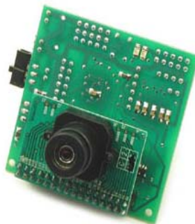
Figure 11. CMUcam2 Vision Sensor Courtesy of Acroname Inc, www.acroname.com
