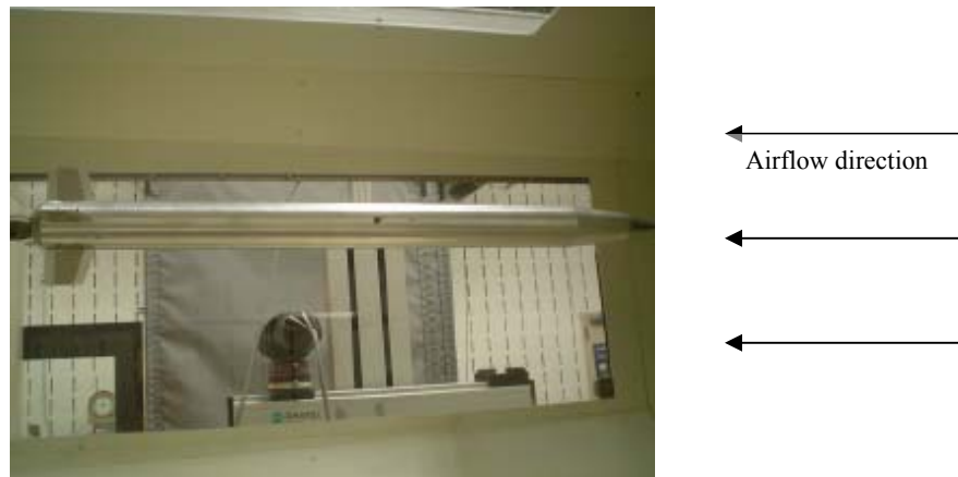
Figure 12. Missile model mounted in tunnel.
