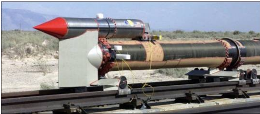
Figure 2 - Dual Rail Sled with Pusher Motors
