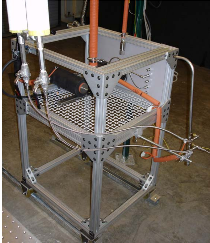
Figure 36: Combustor stand with exhaust probe assembly.
