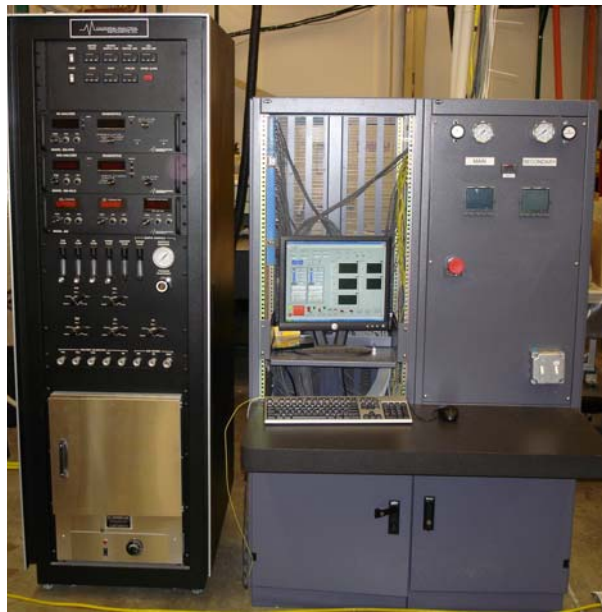
Figure 18: California Analytical Instruments raw exhaust analyzer test bench (l) and laboratory computer control station (r).
