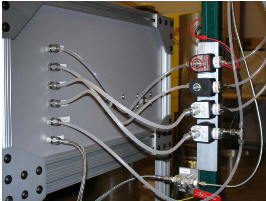
Figure 31: Solenoid valves controlling ignition and purge systems and their connection to the combustor stand.
