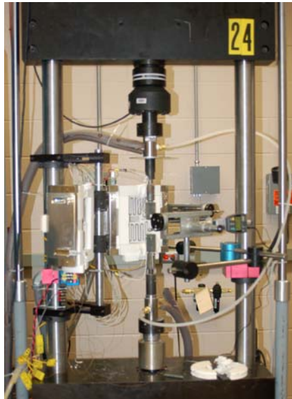
Figure 3.21: Equipment used for testing CT specimen. Optical microscope and extensometer equipment is included on apparatus for manually recording data while testing.
