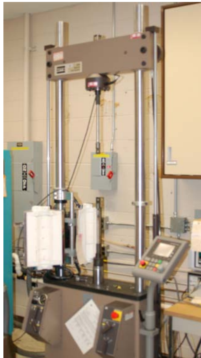
Figure 3.16: MTS 810 Material Test System used to obtain tensile property data.
