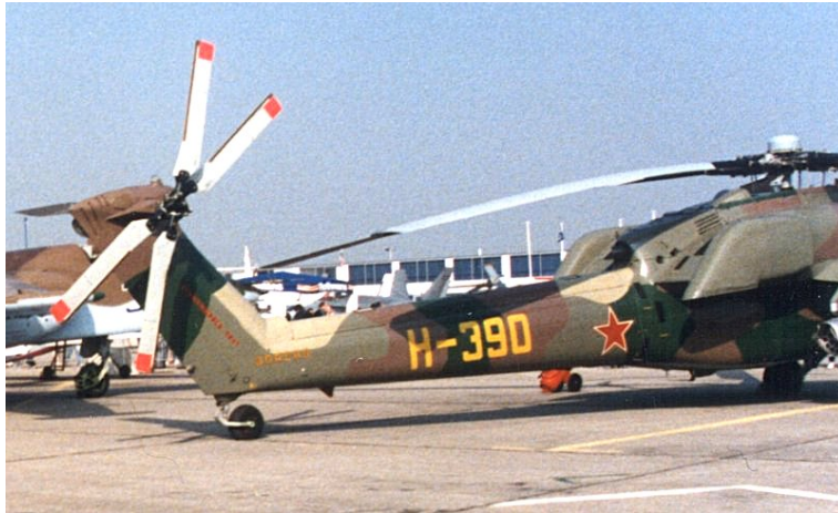
Figure 3. MIL MI-28 Scissor Tail Rotor Variant
