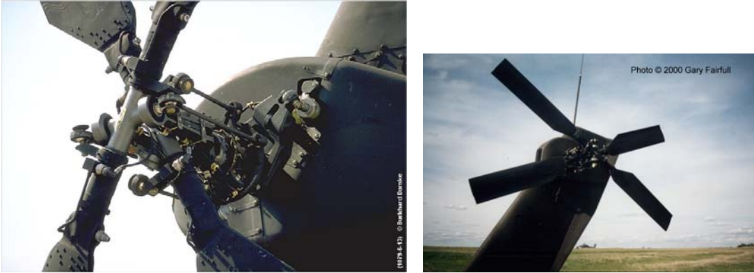
Figure 1. AH-64 Apache Tail Rotor Hub and Rotor Blades
