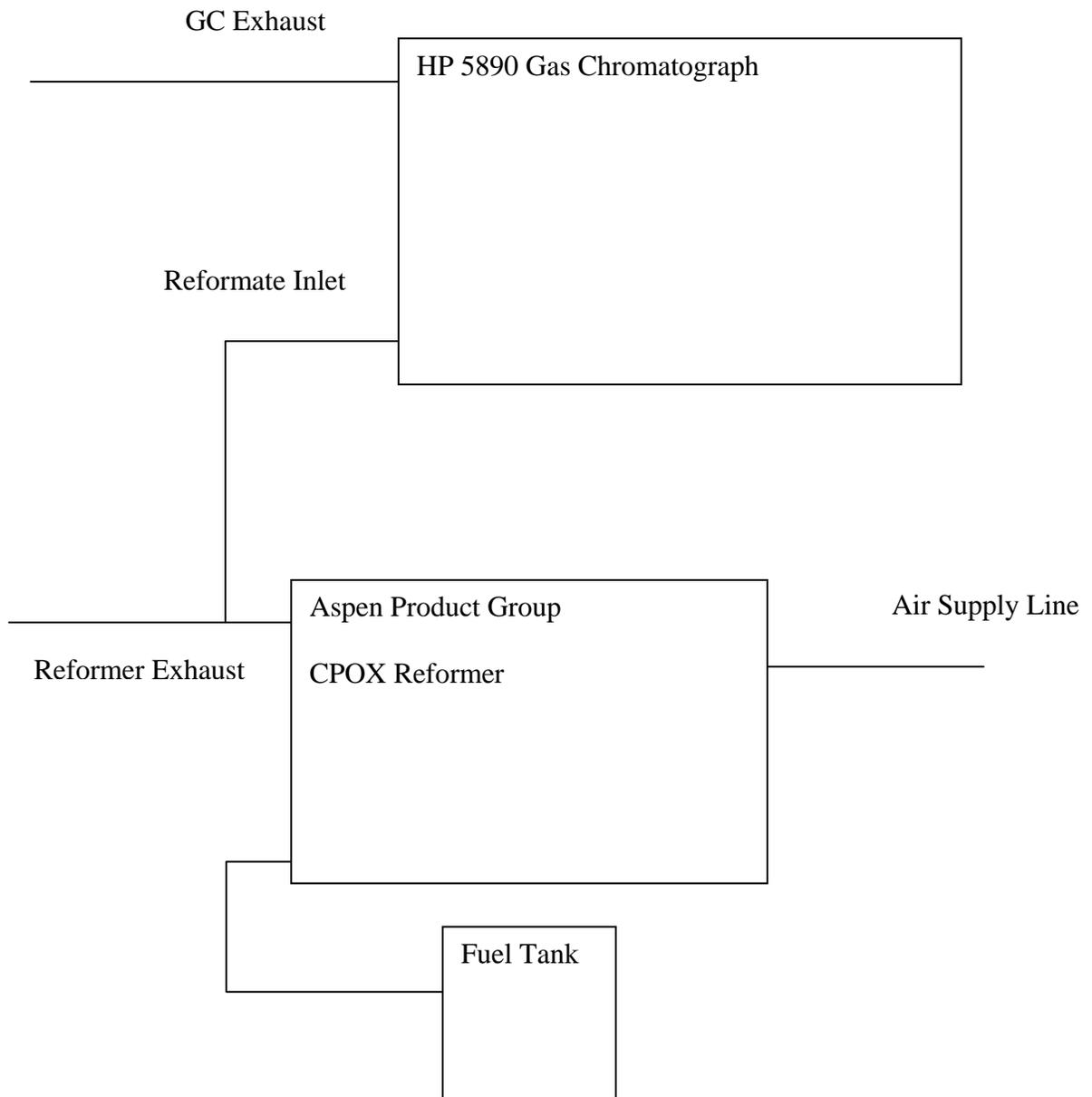
**Figure 6: Schematic of experiment setup**
