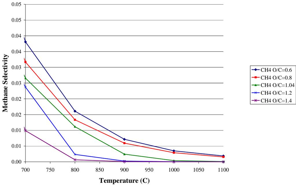
**Figure 16: Carbon selectivity to methane with varying O/C ratios with respect to temperature**
