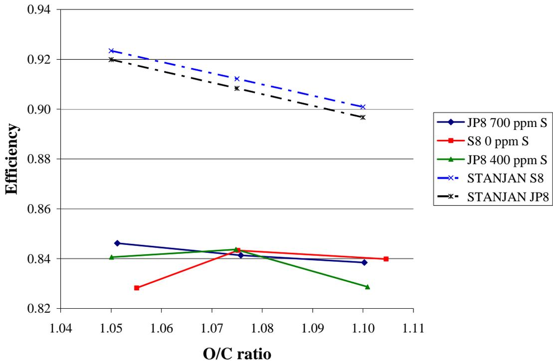
**Figure 28: Efficiency of Aspen Reformer with various fuels and modeled fuels with respect to O/C ratios**
