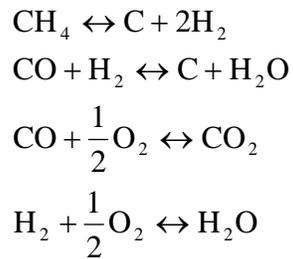
The reactions above either cause coking or will take a desired product of CO and H<sub>2</sub> and convert it into an undesirable product. The design points for the reformer with JP8 fuel are shown in Table 3. Table 3 shows the reformer should be used at an O/C ratio of 1.04 and a temperature of approximately 1000°C.
