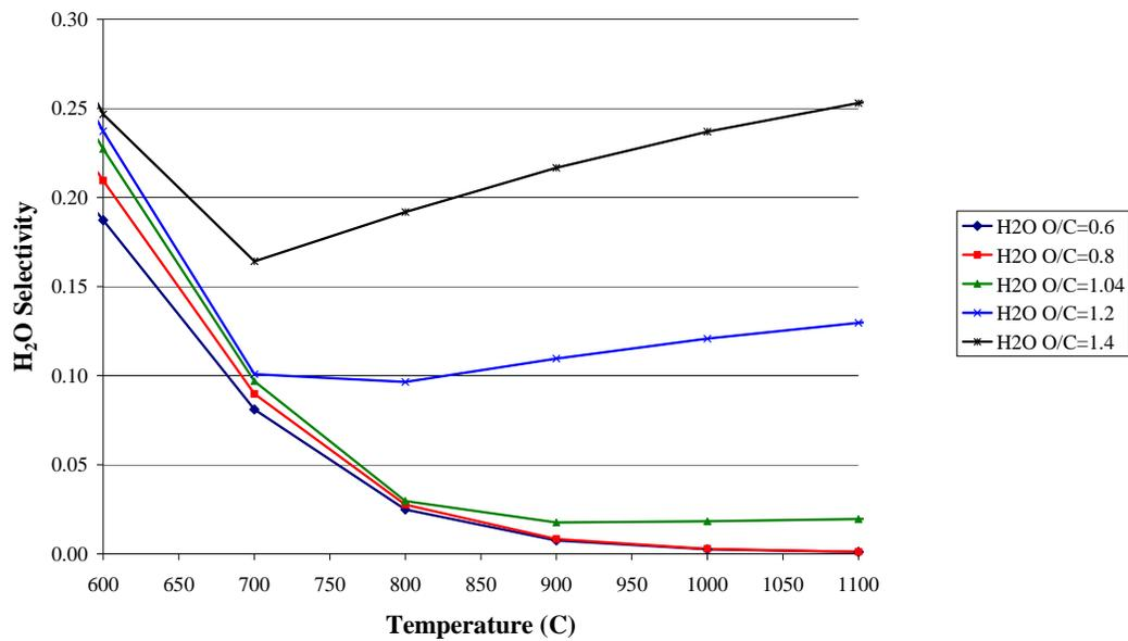
**Figure 17: Hydrogen selectivity to water varying O/C ratios with respect to temperature**
