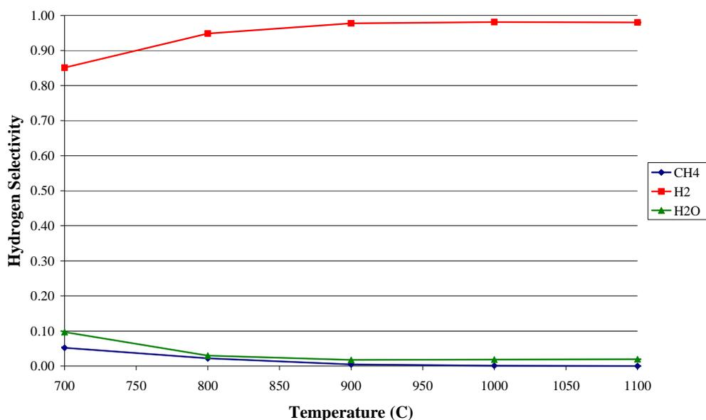
**Figure 15: Major hydrogen products with an O/C ratio of 1.04 with respect to temperature**
