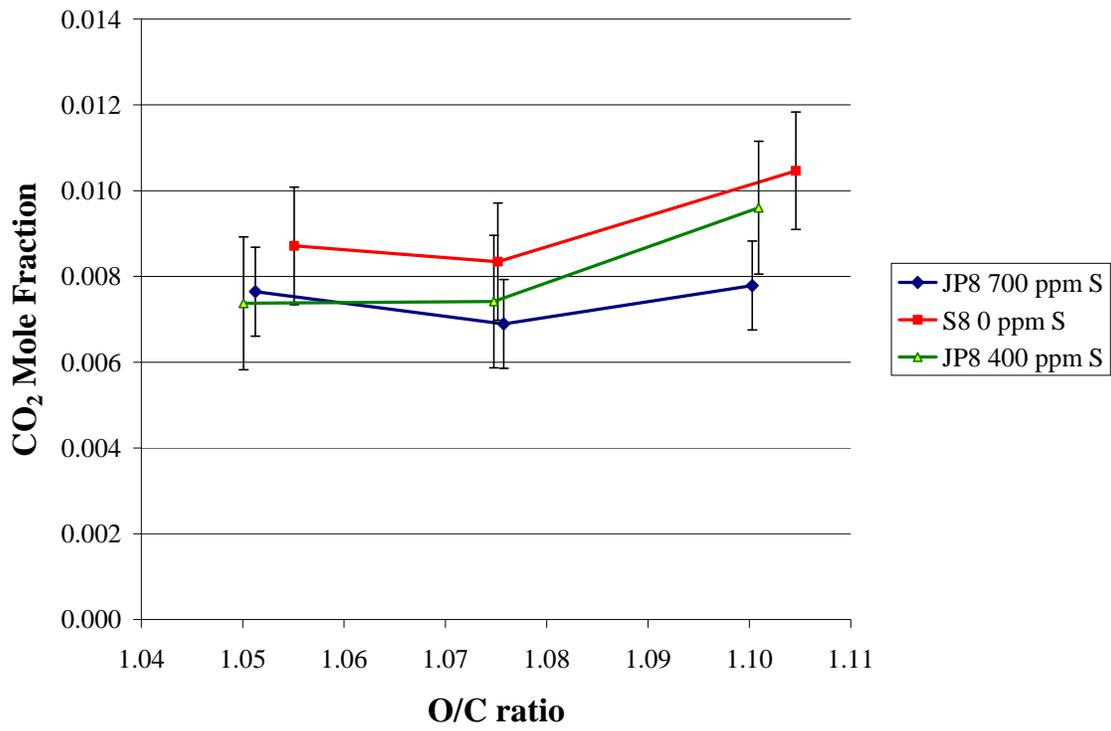
**Figure 35: CO<sub>2</sub> varying O/C ratios with statistical error**
