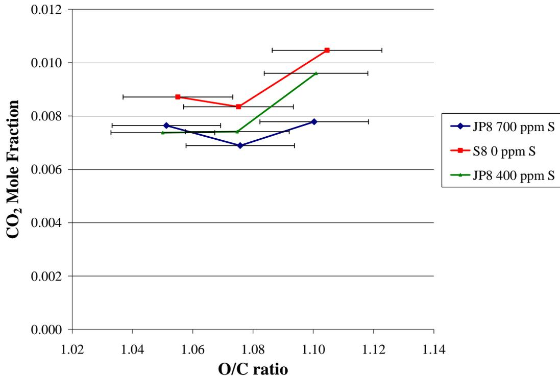
**Figure 36: CO<sub>2</sub> varying O/C ratios showing O/C ratio systematic error**
