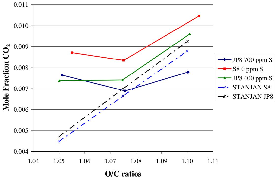
**Figure 26: The effects of varying O/C ratios on the CO<sub>2</sub> production with various fuels and modeled fuels**
