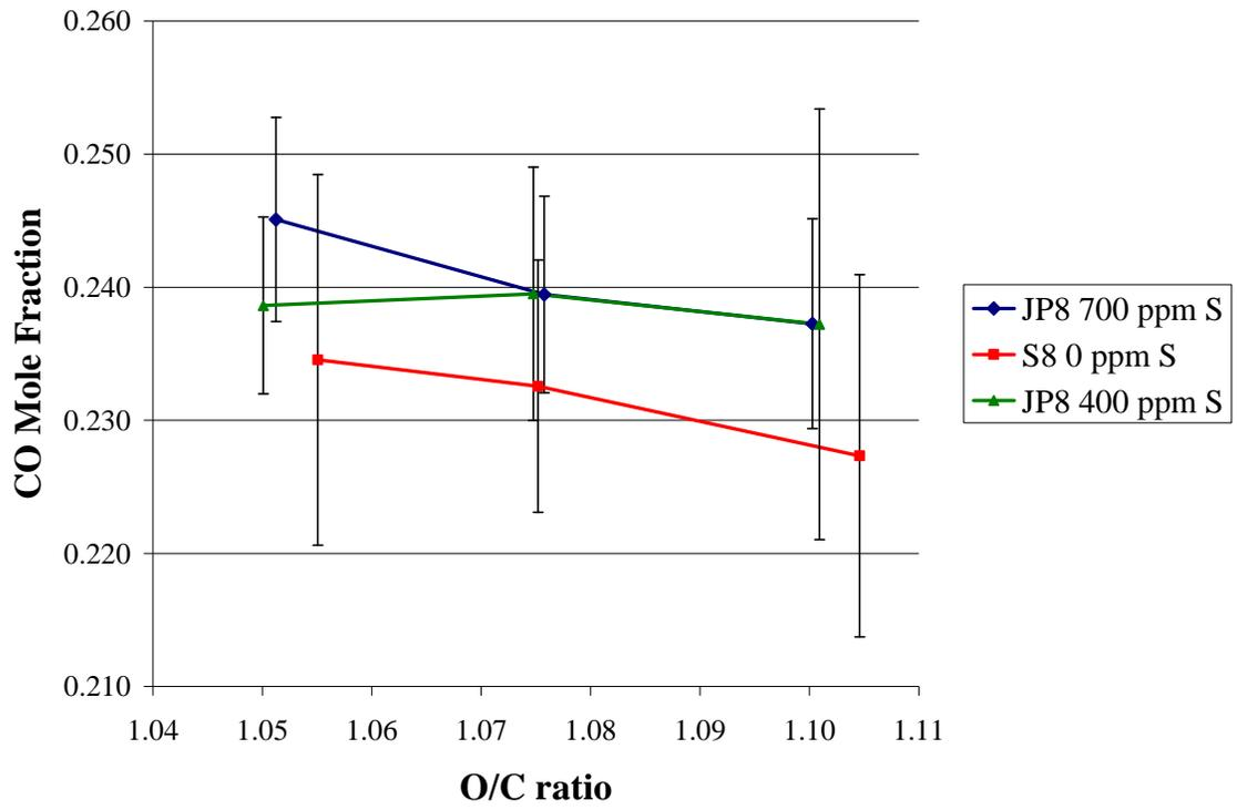
**Figure 33: CO varying O/C ratio with statistical error**
