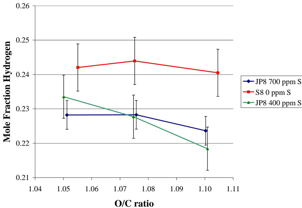
**Figure 8: Hydrogen varying O/C ratio with statistical error**
