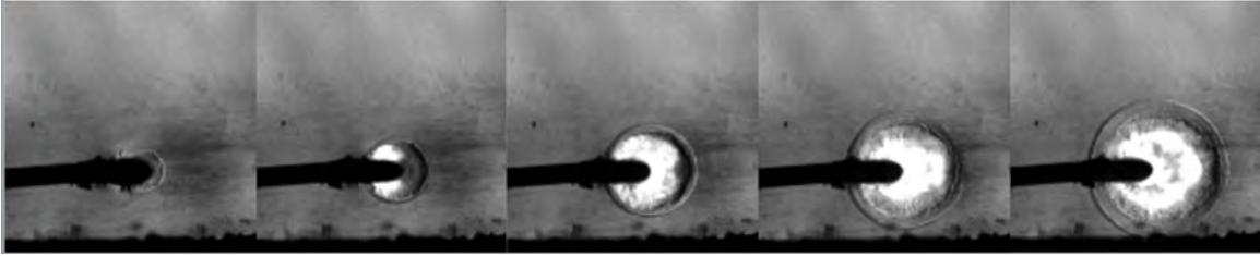
Figure 4.1. Video of 45° inclination into mixture with \phi=1 (210,526 fps)
