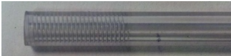
Figure 3.12. An example of pre-detonator threading on 6.35 mm OD tube
