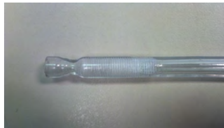
Figure 4.9. Melted 33 mm threaded tubing formed a nozzle shape
