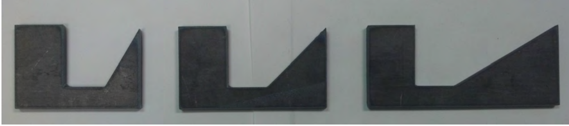
Figure 3.10. Channel geometry with 30°, 45° and 60° wedges
