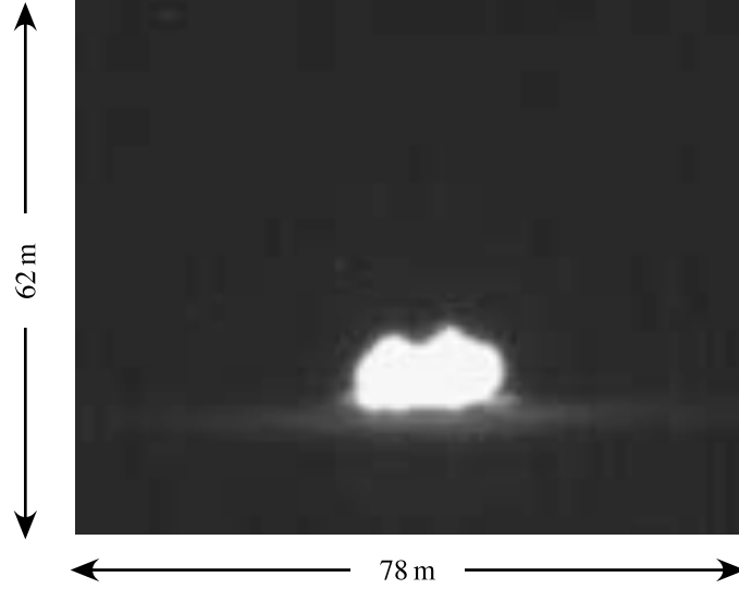
Figure 23: Image captured by the Alpha NIR FPA ( 320 \times 256 ) during the detonation of 50 kg of TNT. The square root of the fireball area, defined by the number of saturated pixels, is approximately 10.5 m.
