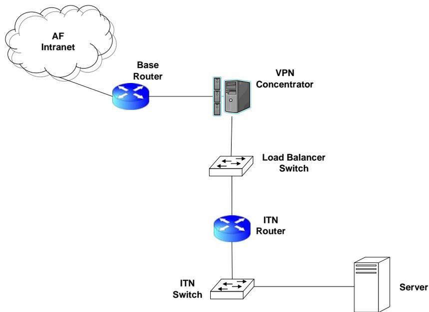
Figure 2.7: Base Network Diagram According to CITS Block 30 Specifications [9]
