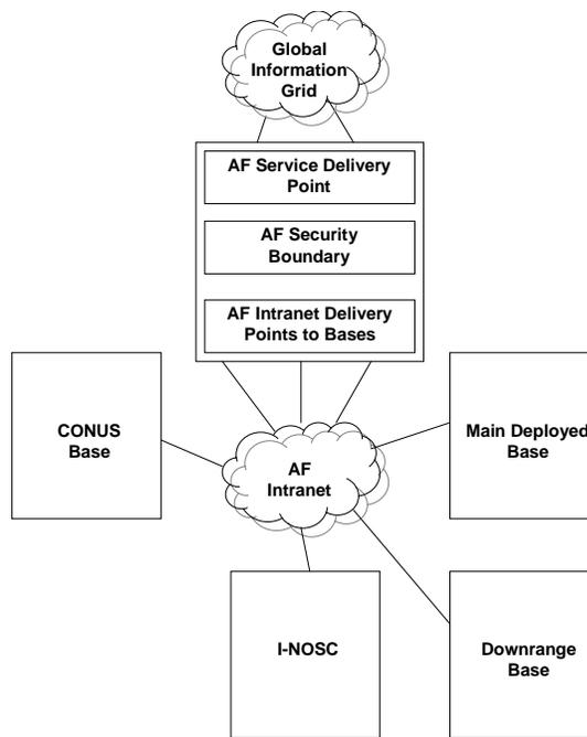
Figure 2.6: Logical Diagram CITS Block 30 Architecture [9]
