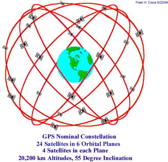
Figure 2.1: View of the GPS constellation orbits [DAN98].
