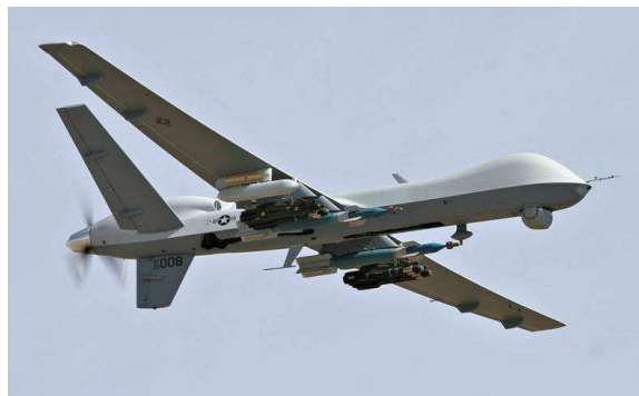
Figure 1.2: The second generation predator with munition carrying hard-points. The precursor to platforms specifically designed asUCAVs.
