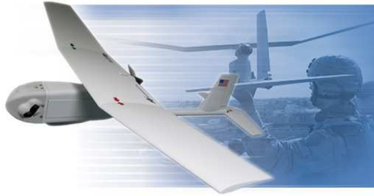
Figure 1.1: The Raven, a hand-launched UAV by AeroViroment [3]
