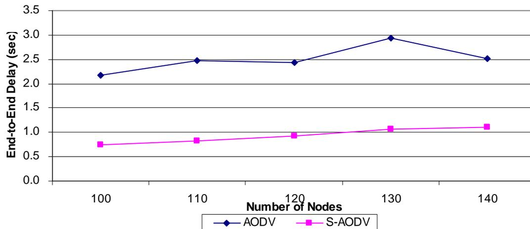
Figure 4.20: End-to-End Delay vs Network Size (Big network)
