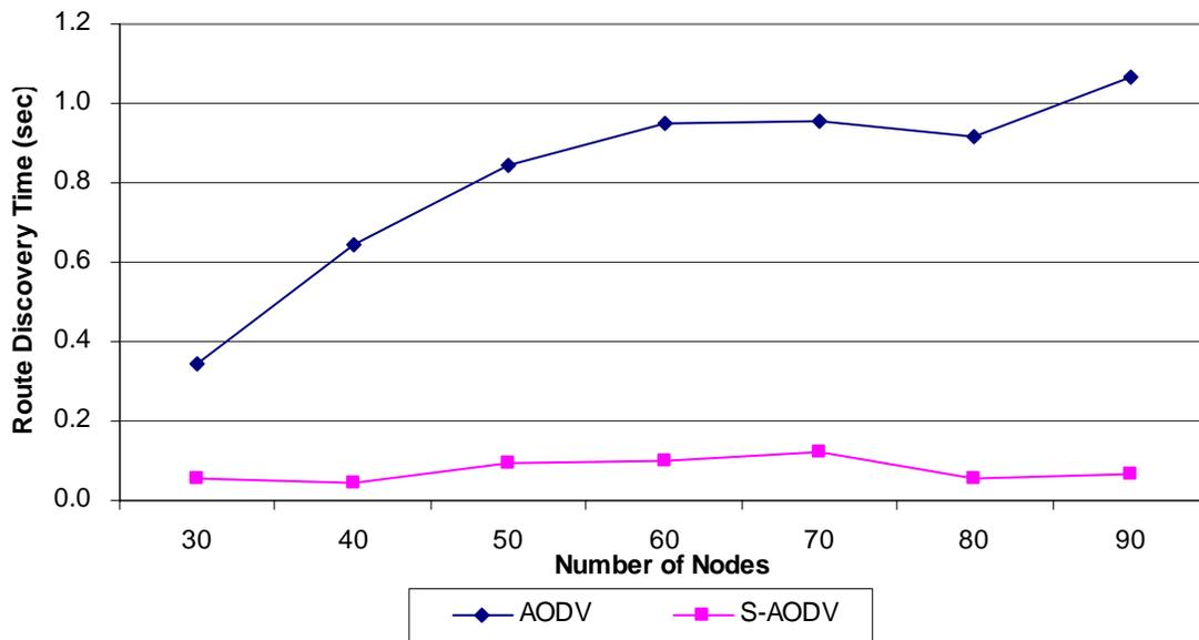
Figure 4.4: Route Discovery Time vs Network Size-uniform Traffic Load
