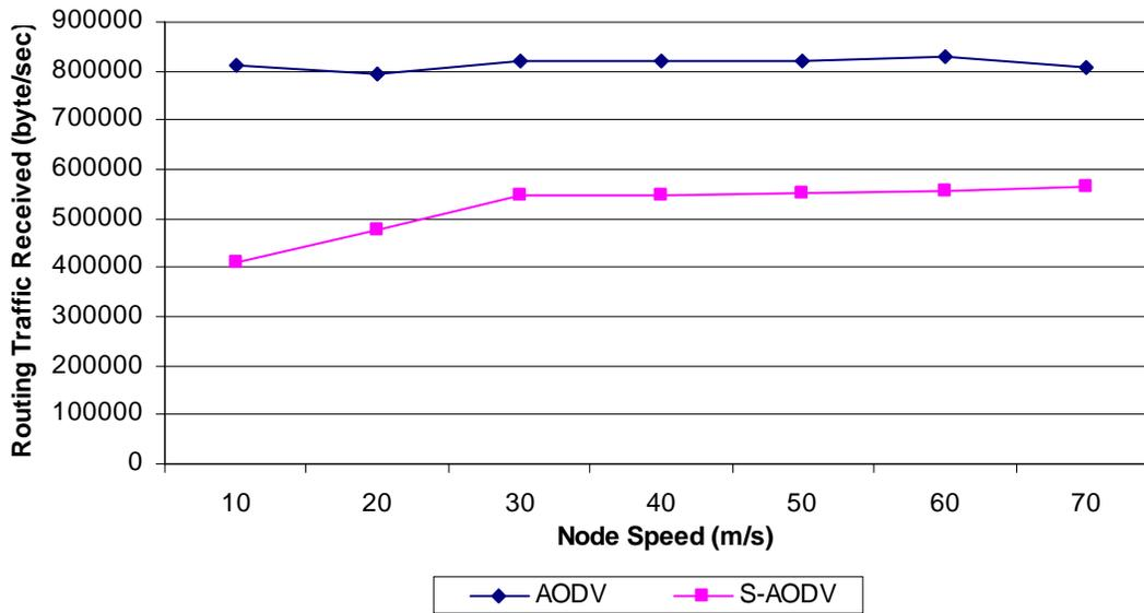
Figure 4.5: Routing Traffic Received Rate vs Node Speed
