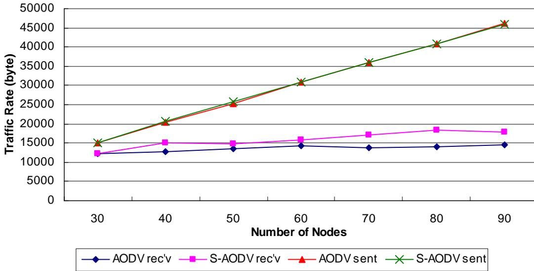
Figure 4.15: Throughput vs Network Size-varying Traffic Load
