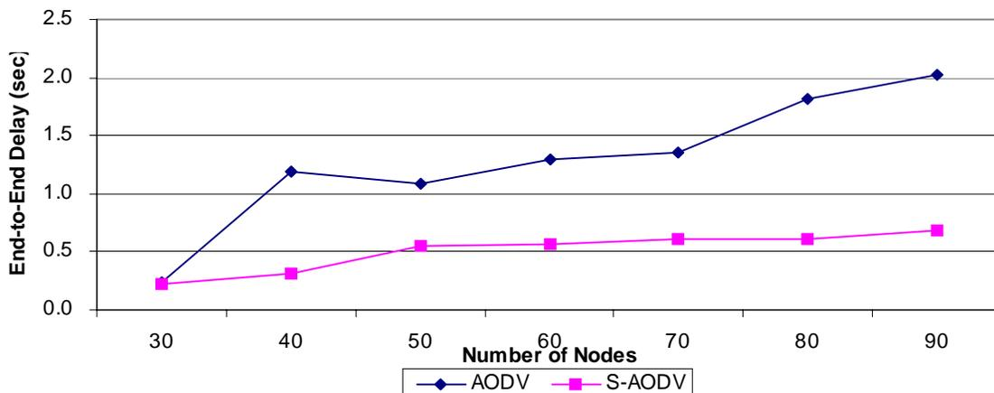
Figure 4.12: End-to-End Delay vs Network Size-Uniform Traffic Load
