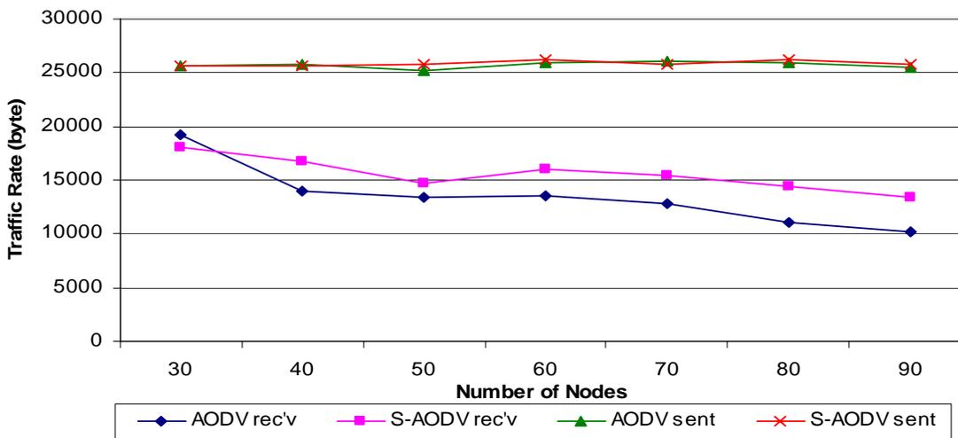
Figure 4.16: Throughput vs Network Size-uniform Traffic Load
