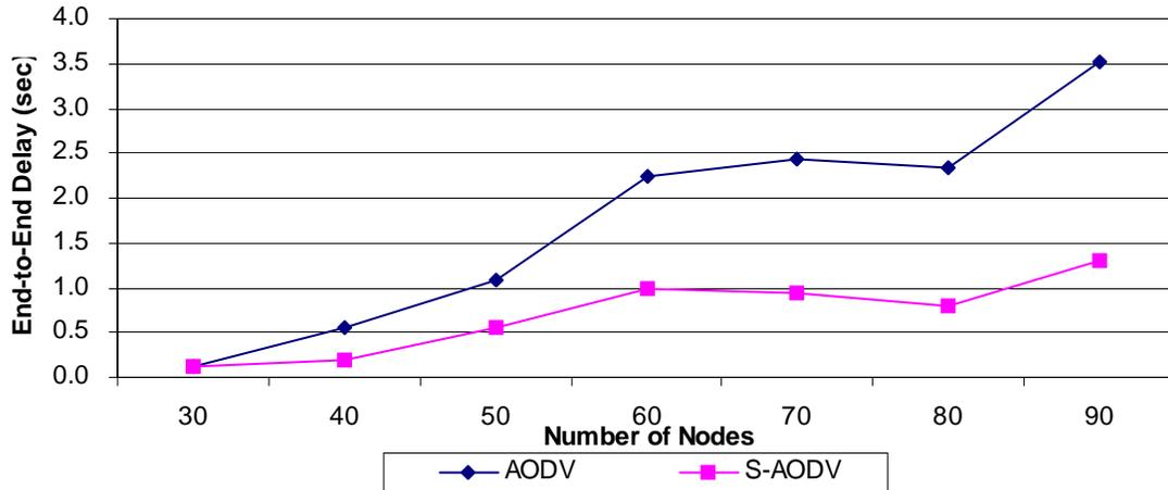
Figure 4.11: End-to-End Delay vs Network Size-varying Traffic Load
