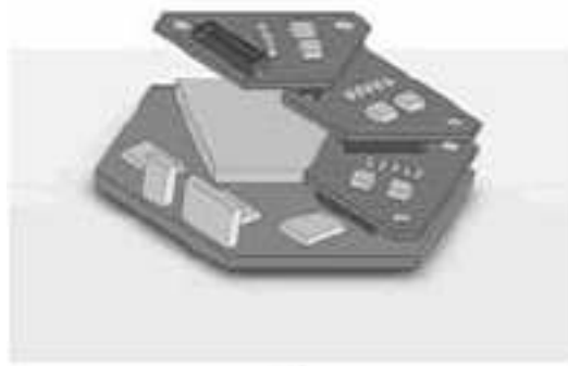
Figure 2.4: The circuitry behind D’Souza’s TerminatorBot, showing the spiral design of the removable FPGA modules
