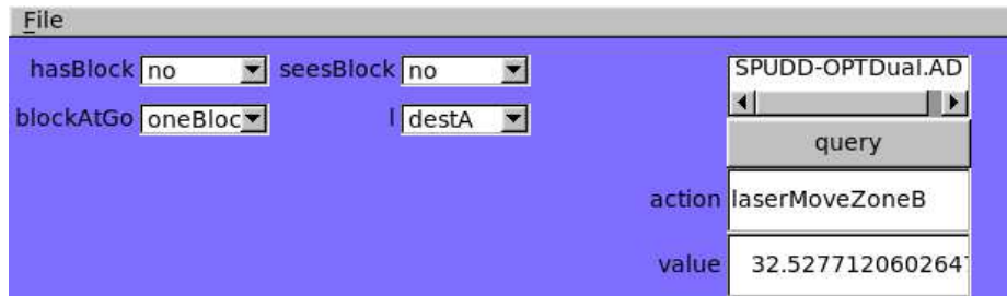
Figure 4.5: A screenshot of the SPUDD interface used to trace through a policy graph. Here, it shows to take the laserMoveZoneB action when the robot is currently at DestA with one block at the goal.
