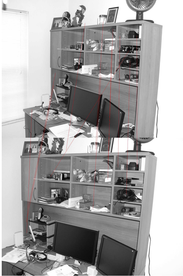
Figure 3.3: An example matching image showing good candidate for keypoint match quality check.
