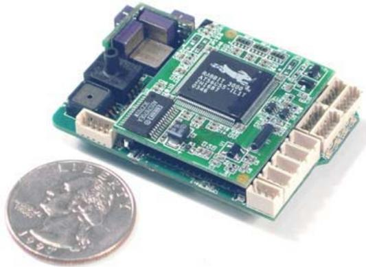
Figure 11: Kestrel Autopilot System (©2008 Procerus Technologies)
