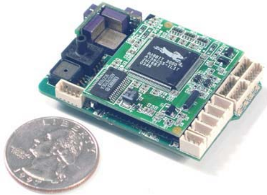
Figure 11: Kestrel Autopilot System (©2008 Procerus Technologies)
