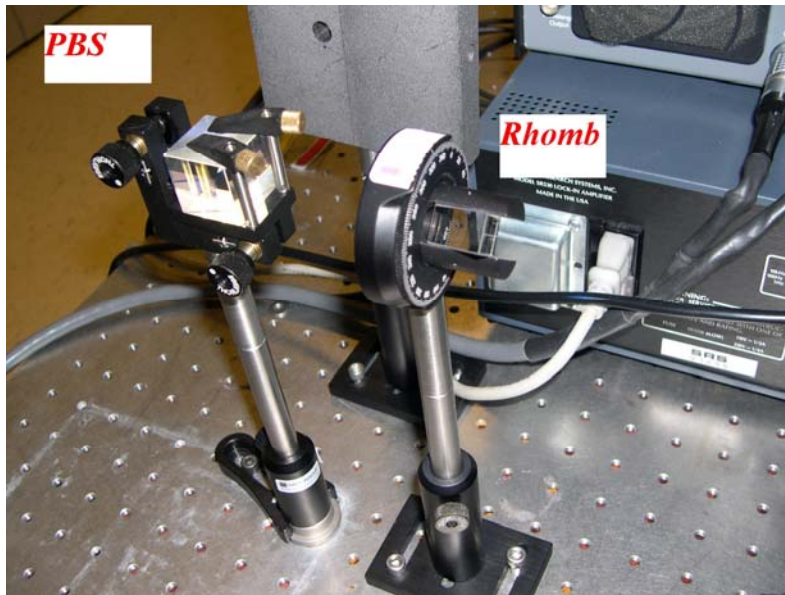
Figure 3.4. A polarizing beam splitter and a rhomb, acting as a quarter waveplate, protect the laser against damaging back reflection.
